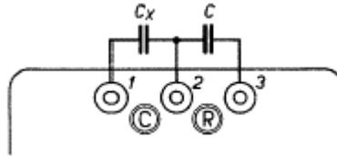
For capacitors, the capacitor to be checked is connected to the terminal "C" and the comparison standard connected to "2 and 3". Bridge balance knob "V" is used to indicate how many per cent it is larger or is smaller than the comparison standard. This measurement can be done at reduced sensitivity, which is a very fast way for rough checking, (see below).
