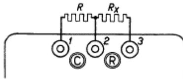
The same procedure can be used to measure of the resistance of electrolytes and other solvents. In this case it is recommended to use a voltage source with a higher frequency (e.g. 500 or 1000 Hz), to prevent electrolysis or polarisation. The "S" on open bridge can also be fed with a voltage source with a higher frequency (500 or 1000 Hz) for use with electrolytics to prevent polarisation. Terminals inside the case need to be accessed to use this feature.
