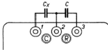
To measure of capacities larger than  $10\ \mu\text{F}$  connect the unknown capacitor to terminal "C" and a similar standard capacity between "2 and 3". Turn knob "S" to the "Open Bridge" position "\/" and after adjusting "V" for balance the unknown capacitance = scale reading  $\times$  standard capacity.
