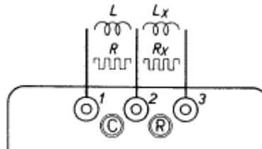
For resistances and self inductances the parts to be checked are connected to the terminal "R" and the comparisons standard connected to "1 and 2".
