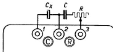
At balance the capacity of the electrolytic capacitor equals the reading multiplied by the standard capacitor and the parasitic resistance of the electrolytic capacitor equals  $1/\text{reading} \times$  setting of the calibrated resistor.
