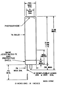
Note: Within this length, maximum diameter of tube is 0.78".
