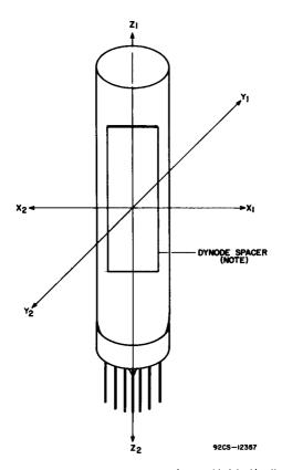
Note: The plane of each dynode spacer is parallel to the X-Z plane. The Z-axis is the major axis of the tube.
