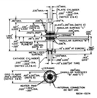
REFERENCE PLANE "A" IS DEFINED AS THAT PLANE AGAINST WHICH ANNULAR SURFACE "B" OF THE GRID FLANGE ABUTS.
