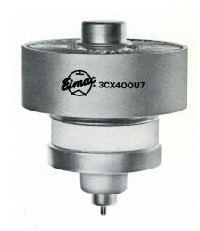
200 watts of useful CW rf power may be obtained with better than 33% efficiency, and better than 10 dB of gain. At frequencies near 900 MHz the amplifier circuit may be essentially a quarter-wave radial or rectangular resonator for the anode, and a three-quarter wave coaxial line section between ground and cathode. The amplifier is described in this data sheet. Terminal collets are available and are listed.
