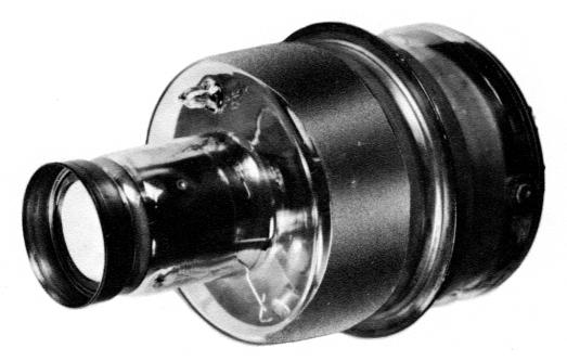
The Image Converter Tube acts as an electronic shutter in photographing extremely short duration events such as explosion phenomena
