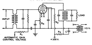
C = 0.05 µf R<sub>3</sub> = 1 R<sub>1</sub> = 0.25 MEGOHM R<sub>K</sub> = 1 R<sub>2</sub> = 30000 OHMS
