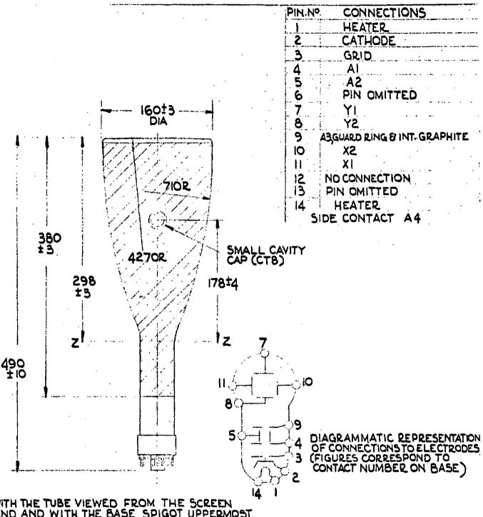
WITH THE TUBE VIEWED FROM THE SCREEN END AND WITH THE BASE SPIGOT UPPERMOST A POSITIVE POTENTIAL APPLIED TO CONTACT II SHALL DEFLECT THE SPOT TOTHE LEFT & A POSITIVE POTENTIAL APPLIED TO CONTACT 7 SHALL DEFLECT THE SPOT UPWARDS
