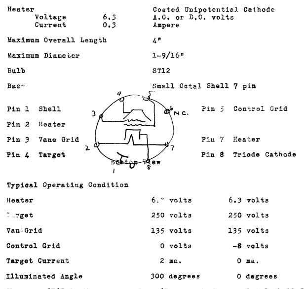
The type 6X6G is the same as Type 685 except that an Octal Shell Bage is used instead of a small six pin base.
