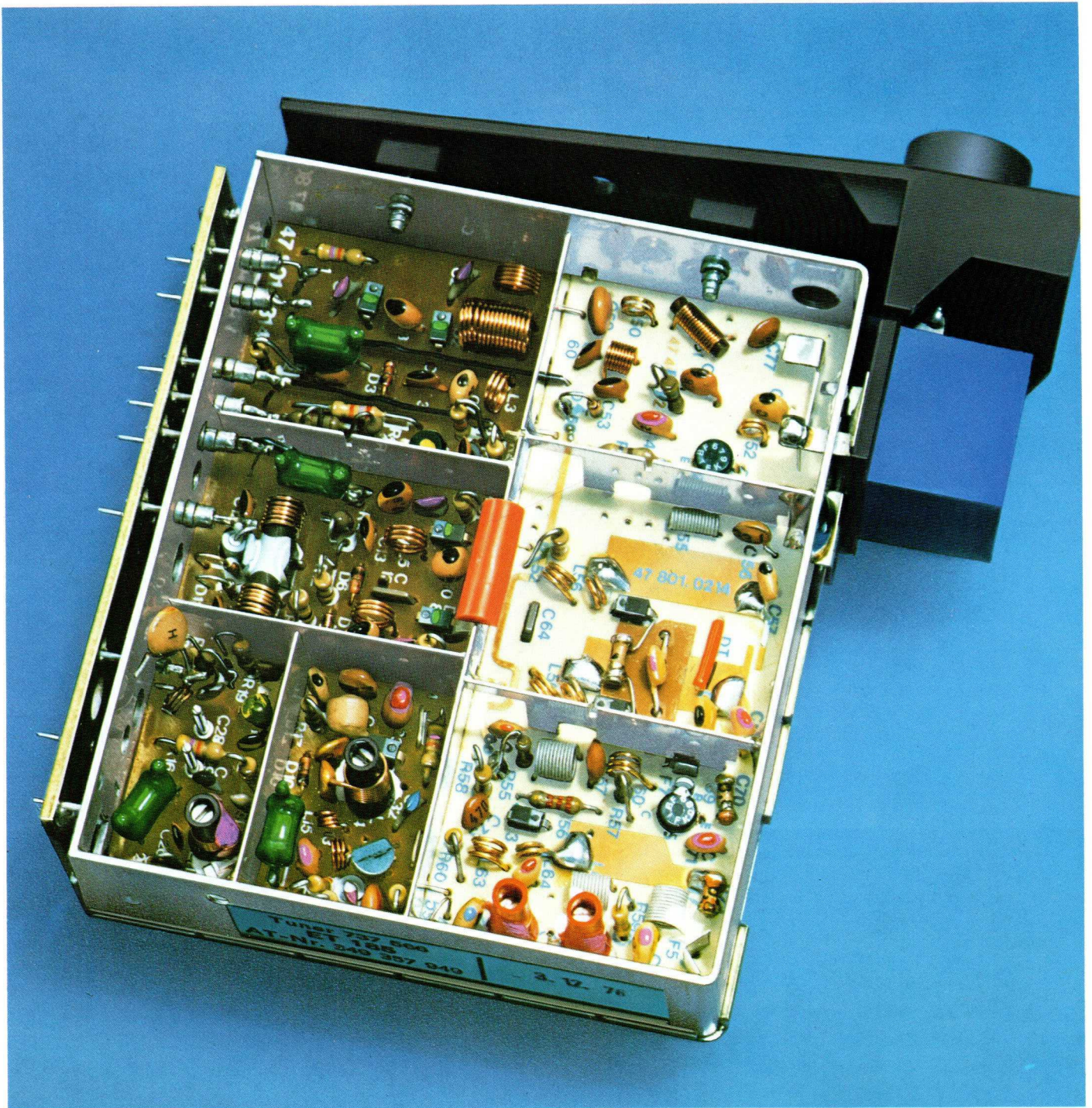
4 4 The view into an open UHF/VHF tuner illustrates the careful processing of all parts
