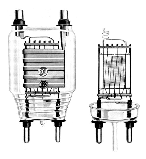
Intended primarily for U.H.F. operation, Radiotron 833 is a 300 watt plate dissipation high-mu triode of special construction for use as R.F. Amplifier, Oscillator and Class B modulator. The plate voltage may be as high as 3000 volts, with a maximum input of 1250 watts. Under typical Class C Telegraphy conditions of operation a maximum power output of 1000 watts is obtainable, while as a plate-modulated R.F. Amplifier the maximum power output is 635 watts. As a result of the special
