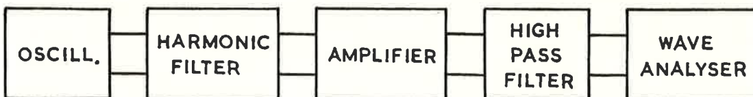
Fig. 1. Method used for measuring oscillator distortion (RT81).
