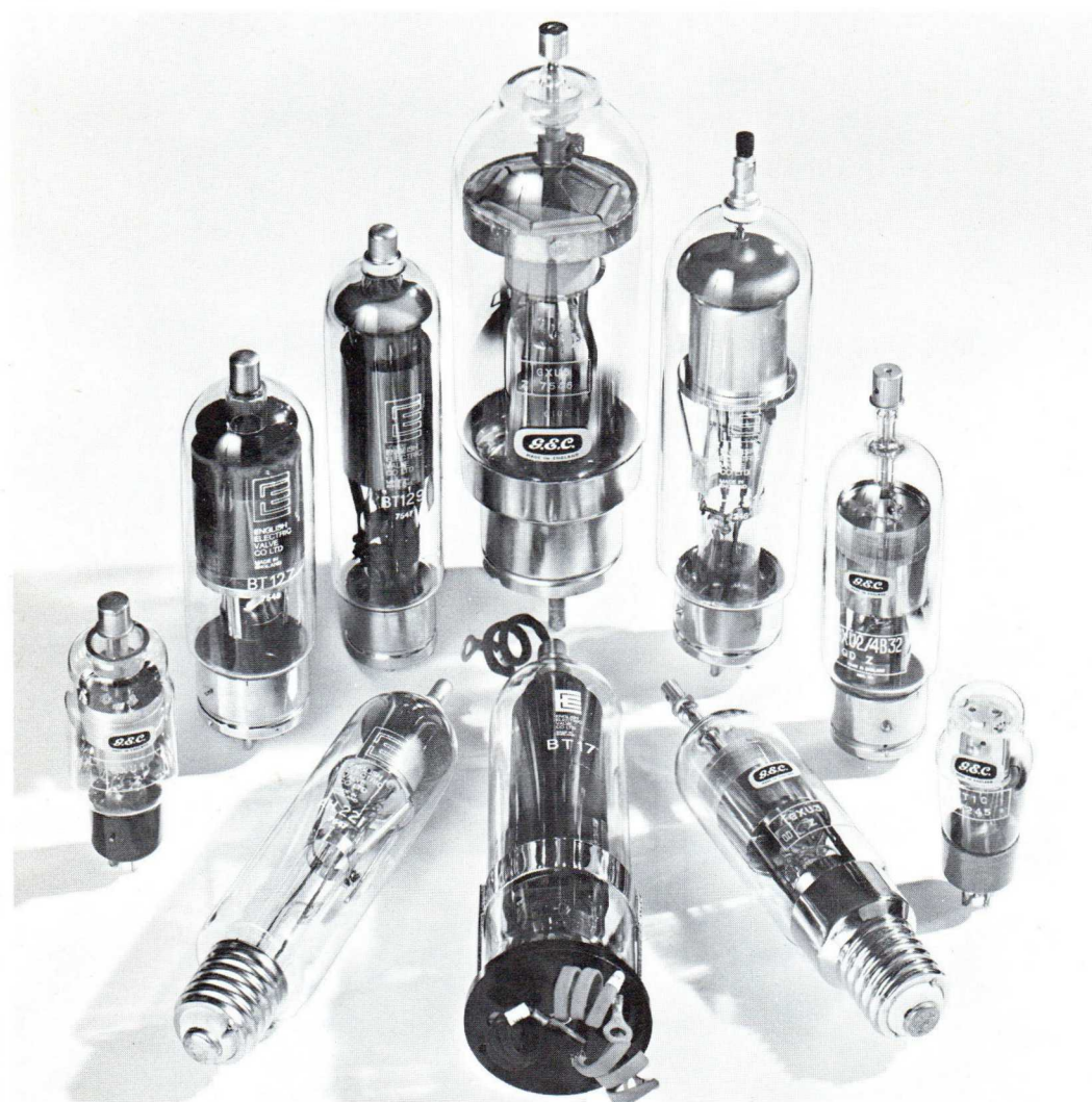
A group of Rectifiers and Thyratrons
