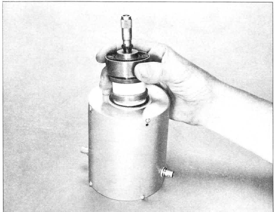
Figure 8—Dummy Tube and Cavity for Effective Capacitance Measurement
