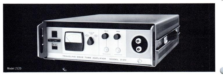
Huggins non-stop quality line of Traveling Wave Tube Amplifiers embodies a conceptually-fresh approach to TWT packaging—an approach which exemplifies quality and technological achievement. Compact, versatile microwave units covering the frequency range of 250 mc to 18.0 Gc are offered in the standard line. Broadband small-signal gain is typically 30 db, and output powers up to 2 watts are available as standard units. All models can be supplied to commercial or military specifications.
