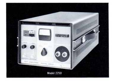
Power Supply Regulation: ±0.1% High Voltage; 2.0% AC Filament Voltage (200 and 300 Series); 1.0% DC Filament Voltage (100 Series); 20 mv peak ripple (200 and 300 Series, DC filament units available on special request).
