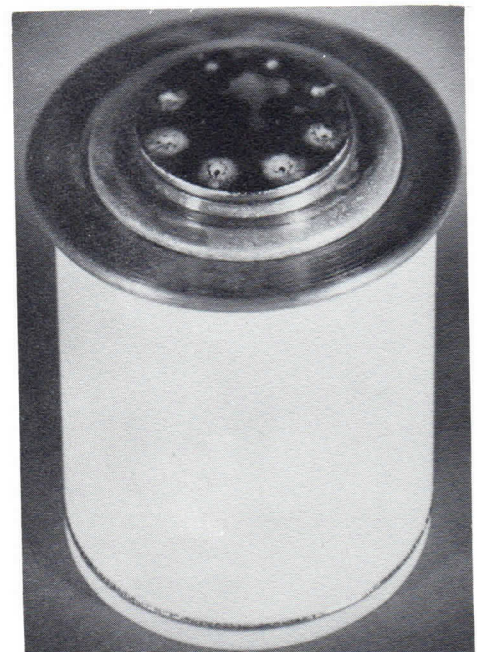
Figure 4: Anode of the same tube showing deep holes at the impact areas of the discharge. Gradient grids have eight .104" dia. holes.
