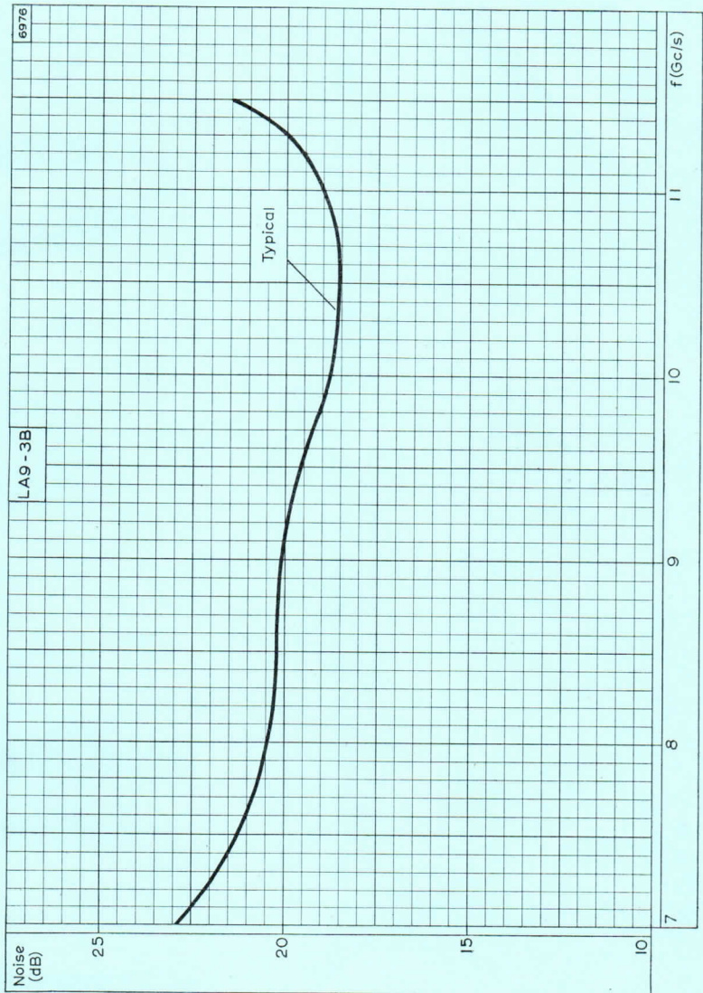
TYPICAL NOISE FACTOR PLOTTED AGAINST FREQUENCY
