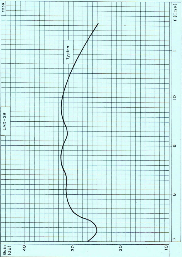
TYPICAL GAIN PLOTTED AGAINST FREQUENCY
