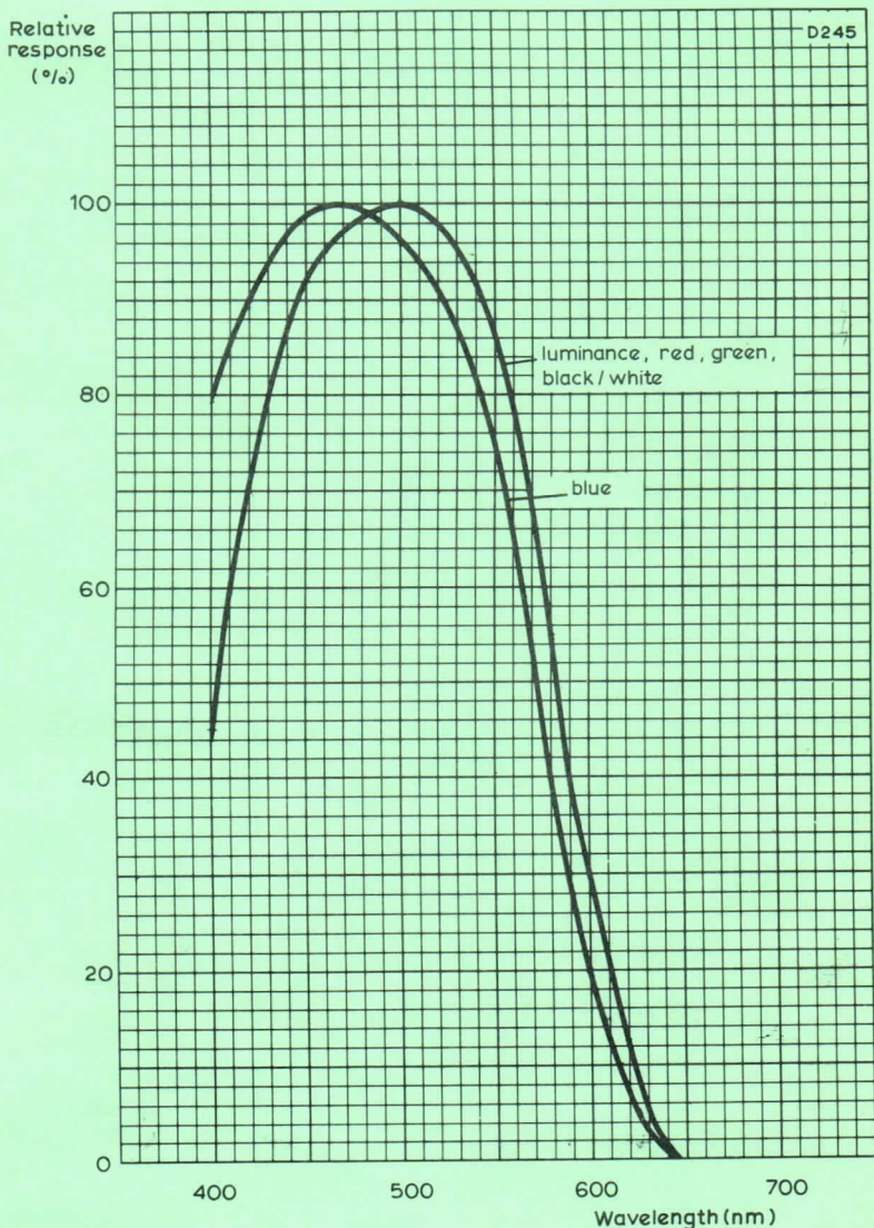
TYPICAL SPECTRAL RESPONSE CURVES
