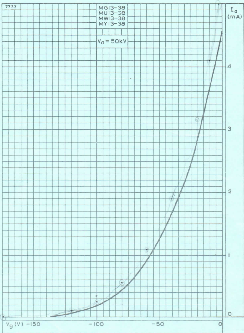
ANODE CURRENT PLOTTED AGAINST GRID VOLTAGE
