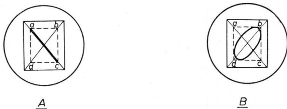
Fig. 70. A a-c is the trace when Z in Fig. 12 is a resistor and the variable resistor R is adjusted until V_R = V_Z B Trace when Z in Fig. 14 is the capacitor or inductor under test and variable resistor R is readjusted so that V_R = V_Z
