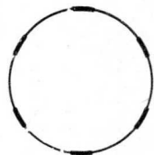
Fig. 79. Trace corresponding to f_1/f_2 = 6 using the circular time base method with beam modulation
