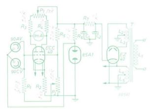
Fig. 76. Circuit of the V.T. voltmeter to be used with the spectro photometer.
