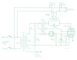
Fig. 50. Circuit diagram of the smoke detector.
