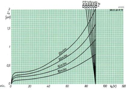
Fig. 24.  $I_a/V_a$  characteristic.
