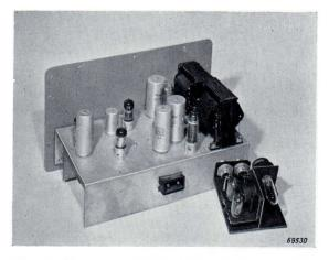
Fig. 61. The scanner (right) and the phototube amplifier opened.
