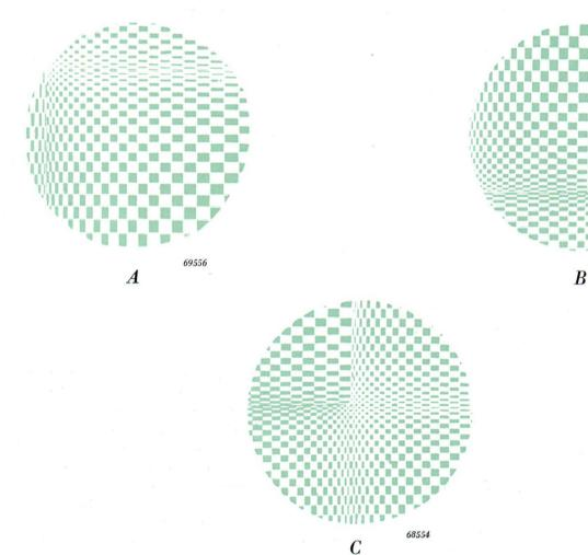
Fig. 55. Gratings to use in combination with an aniseikon. Any combination of two of these gratings will result in the aniseikonic effect.
