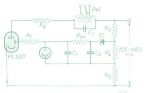
Fig. 44. Circuit diagram of relay amplifier with trigger tube PL 1267.
