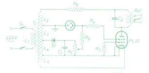
Fig. 41. Circuit diagram of an electronic switch with thyratron PL 21.
