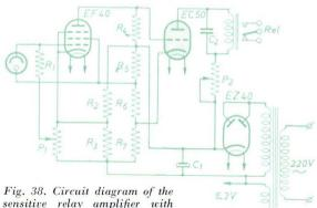
This circuit is very sensitive. If  $P_1$  is adjusted minutely at such a value that the EC 50 is on the verge of firing, a decrease of light of less than 0.001 lm is sufficient to close the relay (with a gas-filled phototube of a sensitivity of 150  $\mu$ A/lm). In this case, however, the relay will not open again when the light is restored to the original value. If the relay has to close and to open, the maximum sensitivity of this circuit is 0.004 lm.
