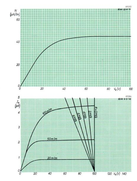
Fig. 10. Saturation characteristic.
