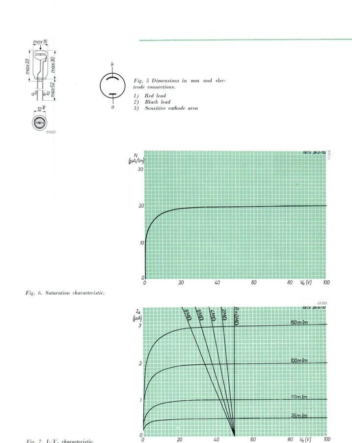
Fig. 7.  $I_a/V_a$  characteristic.
