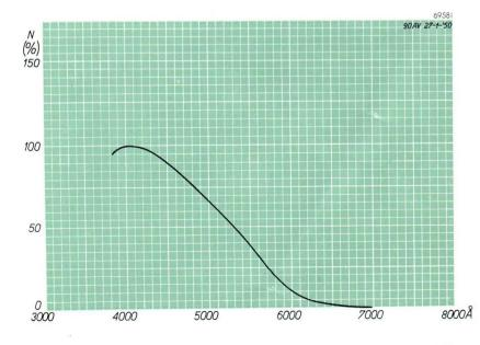
Fig. 2. Spectral response curve of phototube with "C" type of cathode.
