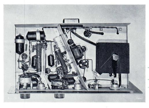
Fig. 62. Under-chassis view of the phototube amplifier.
