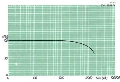
Fig. 21. Frequency characteristic of gasfilled phototube.
