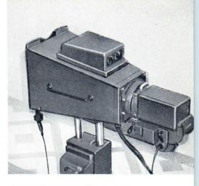
Fig.37. Camera part of X-ray apparatus for medical mass chest examination. The phototube installation measuring the light intensity on the luminescent screen (the photo timer) is mounted in the hood.
