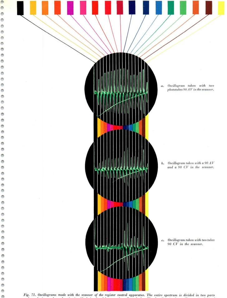
Fig. 71. Oscillograms made with the scanner of the register control apparatus. The entire spectrum is divided in two parts and to obtain good synchronization black is placed between the yellow shades. The first line in the oscillogram is obtained with black and can be used as a reference line to compare the response for the different colours.
