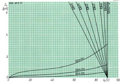
Fig. 33.  $I_a/V_a$  characteristic.
