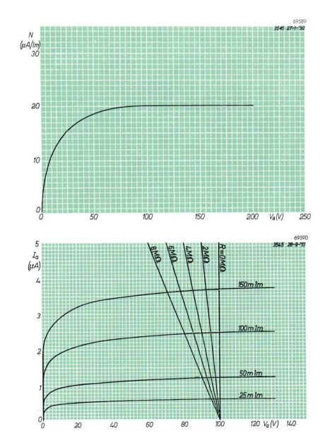
Fig. 18. Saturation characteristic.
