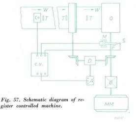
motor A. The field coils of this motor are excited by the electronic register control unit CU, this obtaining its commanding signals from the phototube P and from the magnetic pick-up M, whilst it is brought into the control position by the switch S.
