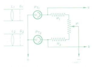
Fig. 53. Schematic diagram of and "Aniseikon".  $L_1$  and  $L_2$ form the binoculars with the gratings  $G_1$  and  $G_2$  behind. The scene is projected on the cothodes of the phototubes,  $Pt_1$  and  $Pt_2$ , the photo current is balanced with the potentiometer P. When something in the scene alters, the balance is upset and a voltage difference occurs between a and b.
