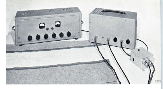
Fig. 60. The electronic part of the register control apparatus. Left: the electronic control apparatus; middle: the phototube amplifier; right: the scanner. In the foreground a colour printed blanket; note the marking spot (the dark stripe on the right side).
