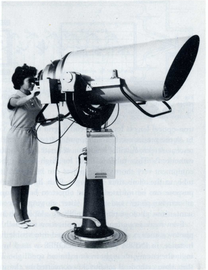
Fig. 97. Telescope with image intensifier (10 000), with which the scenery can be observed in the light from the stars.
