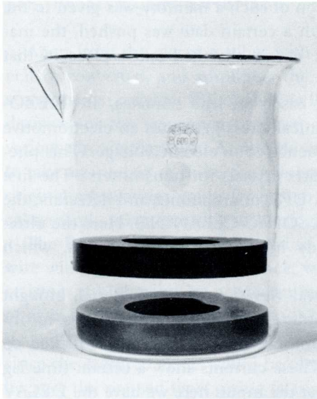
Fig. 26. A ferroxdure magnet ring is kept floating in the air by the magnetic repellent force of another ferroxdure magnet ring. (Philips Technical Review).
