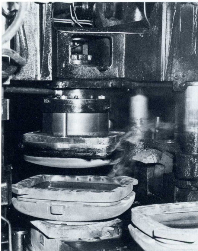
Fig. 20. Pressing the glass screens of rectangular picture tubes.
