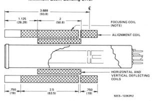
Note: Cross-hatching indicates wound portion of focusing coil.
