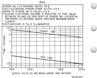
8054 DYNODE No. I - TO - CATHODE VOLTS = 1/6 E EACH SUCCEEDING DYNODE - STAGE VOLTS = 1/12 E ANODE-TO-DYNODE No. 10 VOLTS + 1/2E FOCUSING-ELECTRODE VOLTS = 1/2E BETWEEN 50 AND 100 PER CENT OF DYNODE No.1 POTENTIAL (REFERRED TO CATHODE) WHICH PROVIDES MAXIMUM ANODE CURRENT PHOTOCATHODE IS FULLY ILLUMINATED. 10-7 TRANSIT 8 TIME **TIME - SECONDS** 6 4 2 RISE TIME 10-8 800 1000 1500 SUPPLY VOLTS (E) BETWEEN ANODE AND CATHODE 2000 92LS -1541
