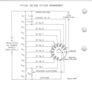
C<sub>1</sub>, C<sub>2</sub>: 0.01  $\mu$ F non-inductive type, 400 volts (dc working). Values dependent on amplitude and duration of pulse. R<sub>1</sub> through R<sub>12</sub>: 33,000 ohms, 2 watts. R<sub>13</sub>: 2.5 megohms, 2 watts, adjustable. Note I: Adjustable between approximately 500 and 1250 volts dc.
