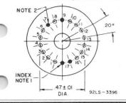
Note 1 – Lead is cut off within 0.12" of glass button for indexing. Note 2 – Lead Nos.7,9, and 17 are cut off within 0.12" of the glass button.
