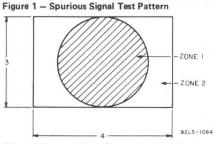
Allowable spot size for each zone is shown in Table I for the 8541A and Table II for the 8541. To be classified as a spot, a contrast ratio of 1.5:1 must exist for white spots and 2:1 for black spots. Smudges, streaks, or mottled and grainy background must have a contrast ratio of 1.5:1 to constitute a reject item. Minimum separation between any 2 spots greater than 1 raster line is limited to 16 raster lines.
