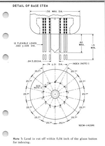
Note 2: Lead No.12 is cut off within 0.04 inch of the glass button.
