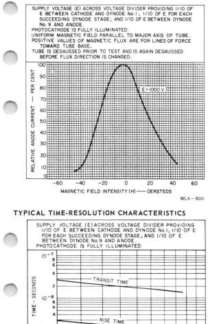
SUPPLY VOLTS (E) BETWEEN ANODE AND CATHODE 92LS-3010
