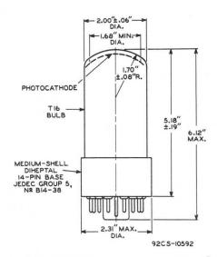
CENTER LINE OF BULB WILL NOT DEVIATE MORE THAN  $2^{\circ}$  IN ANY DIRECTION FROM THE PERPENDICULAR ERECTED AT THE CENTER OF BOTTOM OF THE BASE.
