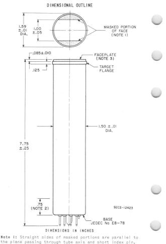
Note 2: Within this area the minimum bulb diameter dimension does not apply.
