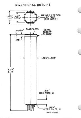
Note 1: Straight Sides Of Masked Portions Are Parallel To The Plane Passing Through Tube Axis And Short Index Pin. Note 2: Within This Distance, Diameter Of Bulb Is 1.025" + 0.003"-0.030".
