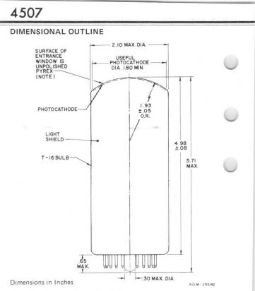
Note: Caution must be employed when handling this tube because of the thinness (approx. 0.02 inch thick) of the entrance window.
