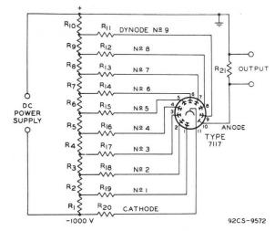
R1 R2 R3 R4 R5 R6 R7 R8 R9 R10: 1 megohm, 1/2 watt R11: 2 megohms, 1/2 watt R12: 5.1 megohms, 1/2 watt R13 R14 R15 R16 R17 R18 R19 R20: 8.2 megohms, 1/2 watt R21: 820,000 ohms, 1/2 watt
