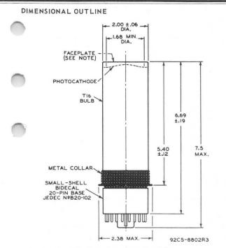
${\mathfrak E}$  of bulb will not deviate more than  $2^0$  in any direction from the perpendicular erected at the center of bottom of the base.
