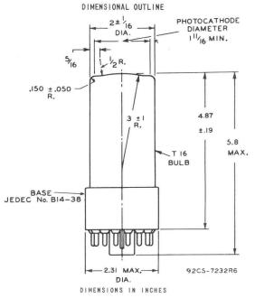
Center line of bulb will not deviate more than  $2^{\circ}$  in any direction from perpendicular erected at the center of bottom of the base.
