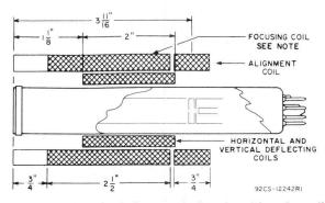
Note: Cross-hatching indicates wound portion of focusing coil.
