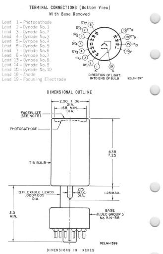
Note: Within 1.68-inch diameter, deviation from flatness of external surface of faceplate will not exceed 0.010 inch from peak to valley.
