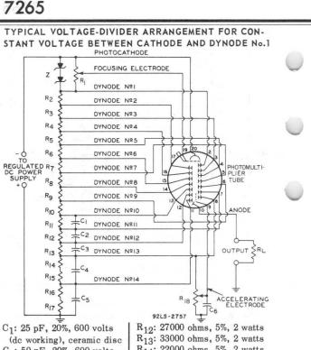
C<sub>2</sub>: 50 pF, 20%, 600 volts (dc working), ceramic disc C<sub>3</sub>: 100 pF, 20%, 600 volts
