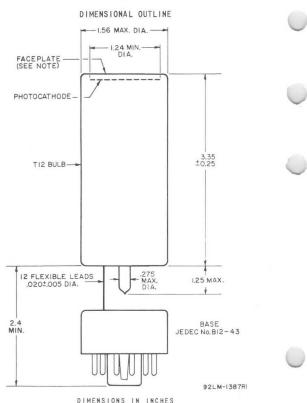
Note: Within 1.24-inch diameter, deviation from flatness of external surface of faceplate will not exceed 0.010-inch from peak to valley.
