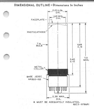
$\ensuremath{\mathbb{Q}}$  of bulb will not deviate more than  $2^o$  in any direction from the perpendicular erected at the center of bottom of the base.
