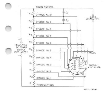
C<sub>1</sub>: 0.02  $\mu$ F, 20%, 500 volts (dc working), ceramic disc C<sub>2</sub>: 0.01  $\mu$ F, 20%, 500 volts (dc working), ceramic disc R<sub>1</sub>: 910,000 ohms, 2 watts
