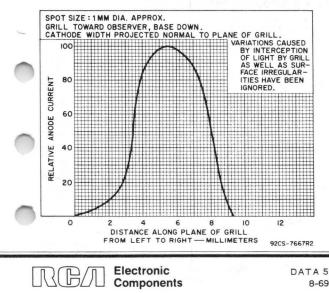
TYPICAL VARIATION OF SENSITIVITY AS TUBE IS ROTATED WITH RESPECT TO FIXED LIGHT BEAM
