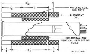
Dimensions in Inches Note: Cross-hatching indicates wound portion of focusing coil.
