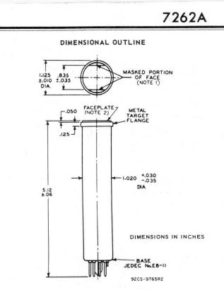
**Note 1:** Straight sides of masked portions are parallel to the plane passing through tube axis and short index pin.
