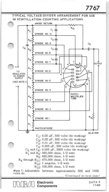
Note 2: Capacitors  $C_1$  through  $C_6$  should be connected at tube socket for optimum high-frequency performance.
