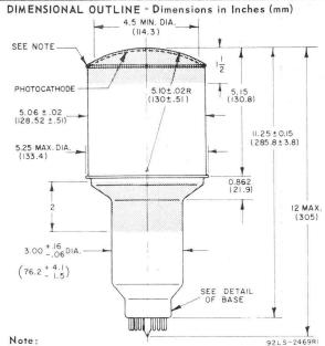
Care must be taken in mounting the tube so that the tube envelope is not subjected to excessive pressure which could strip the glass-to-metal seals. In no case should mounting supports be used in the shaded areas.
