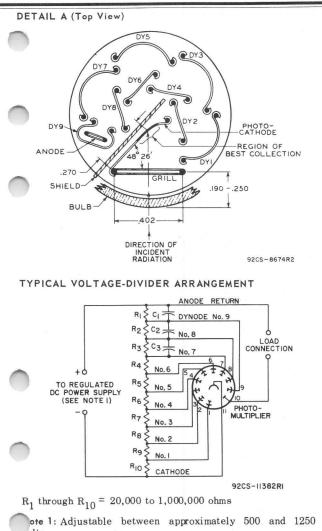
volts. Note 2: Capacitors  $C_1$  through  $C_3$  should be connected at tube socket for optimum high-frequency performance.
