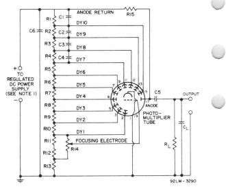
$\begin{array}{rrrr} C_1: & 0.05 \ \mu\text{F}, 500 \ \text{volts} \\ C_2: & 0.02 \ \mu\text{F}, 500 \ \text{volts} \\ C_3: & 0.01 \ \mu\text{F}, 500 \ \text{volts} \\ C_4: & 0.005 \ \mu\text{F}, 500 \ \text{volts} \\ C_5 \ \text{and} \ C_6: & 0.005 \ \mu\text{F}, 3000 \ \text{volts} \\ R_1 \ \text{through} \ R_{13}: \ 470 \ k\Omega, 5\%, 1/2 \ W \\ R_{15}: \ 1 \ M\Omega, 5\%, 1/2 \ W \\ R_{L}: \ 100 \ k\Omega, 5\%, 1/2 \ W \end{array}$
