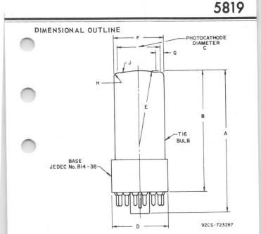
E of bulb will not deviate more than 2<sup>0</sup> in any direction from the perpendicular erected at the center of bottom of the base.
