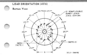
Note 1: Lead No.14 is cut off within 0.04 inch of the glass button for indexing.
