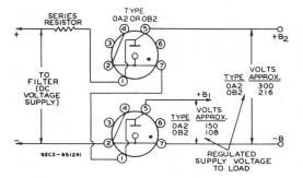
Typical circuit using two OA2's or two OB2's to provide regulated supply voltages of approximately 300 or 216 volts and 150 or 108 volts to load. Socket connections are so made that voltage on load is removed when either tube is taken from its socket.
