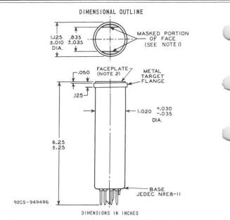
Note 1: Straight sides of masked portions are parallel to the plane passing through tube axis and short pin. Note 2: Faceplate glass is Corning No.7056 having a thickness of 0.094  $\pm$  0.012 inch.
