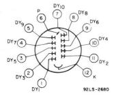
Lead 1: Dynode No.1 Lead 2: Dynode No.3 Lead 3: Dynode No.5 Lead 4: Dynode No.7 Lead 5: Dynode No.9 Lead 6: Anode
