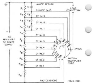
C<sub>1</sub>: 0.05  $\mu$ F, 20%, 500 volts (dc working), ceramic disc C<sub>2</sub>: 0.02  $\mu$ F, 20%, 500 volts (dc working), ceramic disc C<sub>3</sub>: 0.01  $\mu$ F, 20%, 500 volts (dc working), ceramic disc C<sub>4</sub>: 0.005  $\mu$ F, 20%, 500 volts (dc working), ceramic disc R<sub>1</sub> through R<sub>10</sub>: 390,000 ohms, 5%, 1/2 watt R<sub>11</sub>: 910,000 ohms, 5%, 1/2 watt
