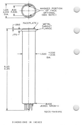
**Note:** Straight sides of masked portions are parallel to the plate passing through tube axis and short pin.
