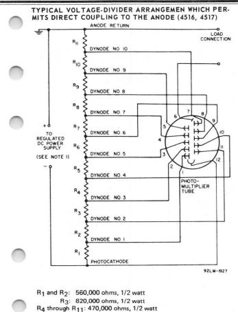
Note 1: Adjustable between approximately 500 and 1800 volts dc. Note 2: Component values are dependent upon nature of application and output signal desired.
