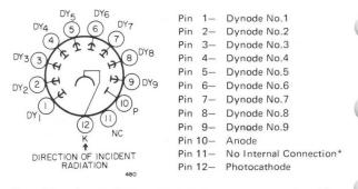
Note: The tube should be rotated about its major axis to provide maximum anode current.
