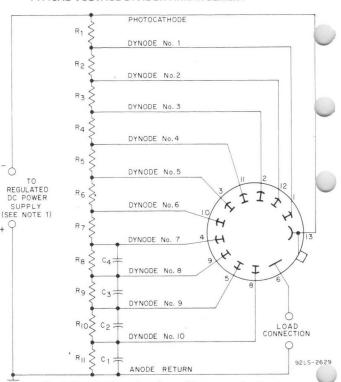
TYPICAL VOLTAGE-DIVIDER ARRANGEMENT
