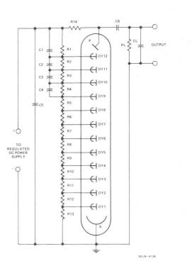
C1: 0.05, 500 VDC, Ceramic Disc C2: 0.02, 500 VDC, Ceramic Disc C3: 0.01, 500 VDC, Ceramic Disc R1 through R10: 270 kΩ±5%,
