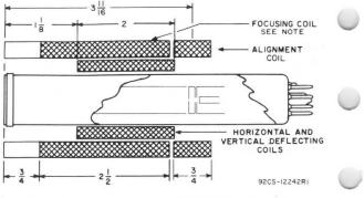
Note: Cross-hatching indicates wound portion of focusing coil.
