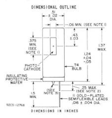
NOTE 1: Minimum projected cathode length and width on plane parallel to grill wires. NOTE 2: Soldering or welding to the leads within this region is
