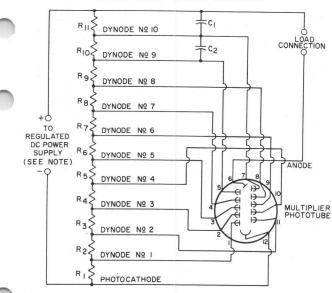
TYPICAL VOLTAGE-DIVIDER ARRANGEMENT
