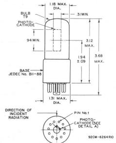
**C** of bulb will not deviate more than 2<sup>0</sup> in any direction from the perpendicular erected at center of bottom of base.
