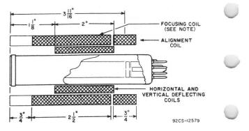
Note: Cross-hatching indicates wound portion of focusing coil.
