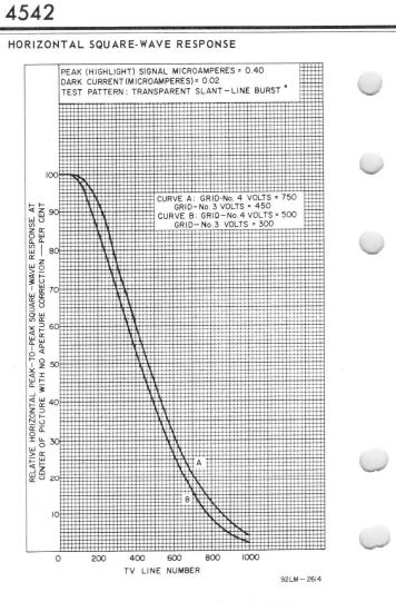
\*Amplitude response measured using the RCA P200 slantline burst pattern with horizontal center response balanced on the 400 line chevrons.
