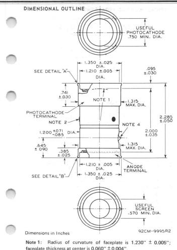
Note 2: Three insulated lead tips will not extend beyond maximum O.D. of tube. Leads are used only during tube manufacture.
