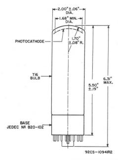
CENTER LINE OF BULB WILL NOT DEVIATE MORE THAN  $2^{\rm O}$  in any direction from the perpendicular erected at the center of bottom of the base.
