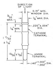
NOTE: WHEN TUBE IS ROTATED ABOUT THE LONGITUDINAL AXIS OF ITS CATHODE TERMINAL, NO PART OF THE ANODE TERMINAL WILL FALL OUTSIDE OF A 0.241"-DIAMETER CIRCLE CONCENTRIC WITH THE LONGITUDINAL AXIS OF THE CATHODE TERMINAL.
