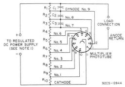
$R_1$  through  $R_{10}$  = 20,000 to 5,000,000 ohms. NOTE I: Adjustable between approximately 500 and 1250 volts. NOTE 2: Capacitors  $C_1$  through  $C_3$  should be connected near tube base for optimum high-frequency performance.
