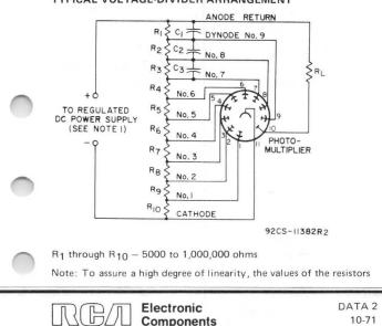
making up the voltage-divider network should be such that the current through the network, for the selected operating supply voltage, is at least 10 times greater than the maximum average anode current required.
