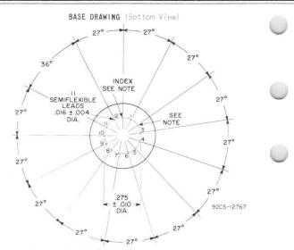
NOTE: Lead is cut off within 0.10 inch of the glass button for indexing.
