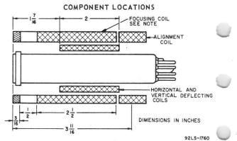
NOTE: CROSS-HATCHING INDICATES WOUND PORTION OF FOCUSING COIL.
