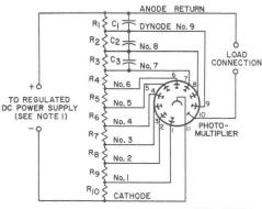
TYPICAL VOLTAGE-DIVIDER ARRANGEMENT
