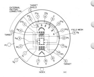
Basing Schematic For Types 4807/V1 And 4807A/V1
