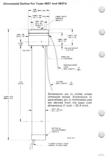
Note 1: Perpendicularity to fiber optic surface is 0.002" T.I.R. Centering is determined by holding and rotating at positions X-X<sub>1</sub> above.
