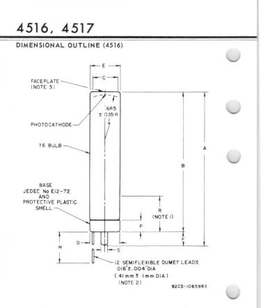
Note 1: Within this length, maximum diameter of tube is 0.78".
