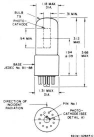
$\mathcal{Q}$  of bulb will not deviate more than  $2^{\circ}$  in any direction from the perpendicular erected at center of bottom of base.
