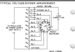
$R_1$  through  $R_{10} = 20,000$  to 1,000,000 ohms
