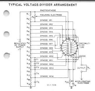
C<sub>1</sub>: 25 pF, 20%, 600 volts (dc working), ceramic disc C<sub>2</sub>: 50 pF, 20%, 600 volts (dc working), ceramic disc C<sub>3</sub>: 100 pF, 20%, 600 volts (dc working), ceramic disc C<sub>4</sub>: 250 pF, 20%, 600 volts (dc working), ceramic disc C<sub>5</sub>: 500 pF, 20%, 600 volts (dc working), ceramic disc C<sub>6</sub>: 100 pF, 20%, 1000 volts (dc working), ceramic disc R<sub>1</sub>: 24000 ohms, 5%, 1 watt
