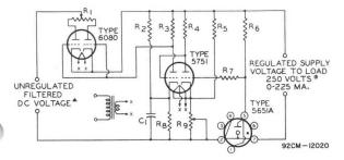
$\begin{array}{l} C_1 = 0.1 \ \mu\text{f}, \ 400 \ \text{volts} \\ R_1 = \text{Plate current balanc-} \\ \text{ing potentiometer,} \\ 160 \ \text{ohms, 10 watts} \\ R_2 = 12000 \ \text{ohms, 2 watts} \\ R_3 = 470000 \ \text{ohms, 1/2 watt} \\ R_4 = \sqrt{70000} \ \text{ohms, 1/2 watt} \end{array}$
