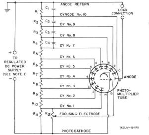
TYPICAL VOLTAGE-DIVIDER ARRANGEMENT
