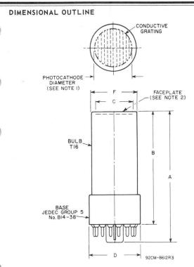
**Note 1:** The grating consists of 12 equally spaced conductive strips having a maximum width of 0.02" (0.5 mm).
