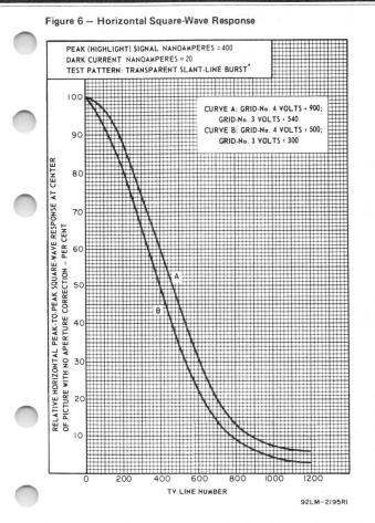
\*Amplitude response measured using the RCA-P200 slant-line burst pattern with horizontal center response balanced on the 400 line chevrons.
