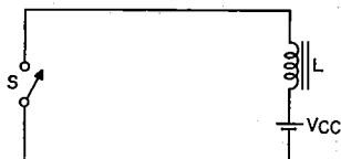
Fig. 85—Simplest form of deflection circuit.
