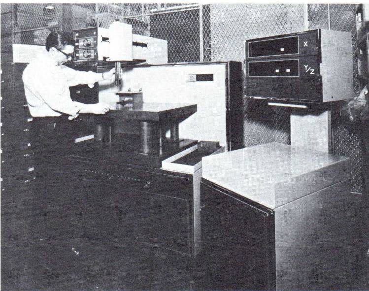
Electronic micrometers for high-precision, three-dimensional measurements in Incoming Inspection department.
