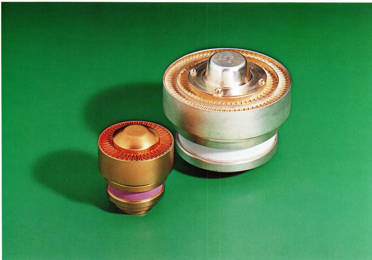
The power output tetrode YL 1110/1 (7650) for applications up to 1 GHz is shown on the left. On the right the 1.1 kW tetrode YL 1231 can be seen which is specially suitable for r.f. stages up to a frequency of 220 MHz.
