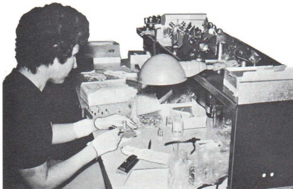
Hand assembly operation of magnetrons indicates the precise skill required for low volume, high precision products.
