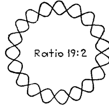
(c) Gear-wheel patterns obtained by inserting high frequency at point B to modulate sensitivity
