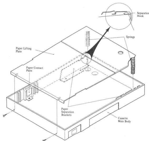
Fig. 4-57 Cassette Assembly Main Components
