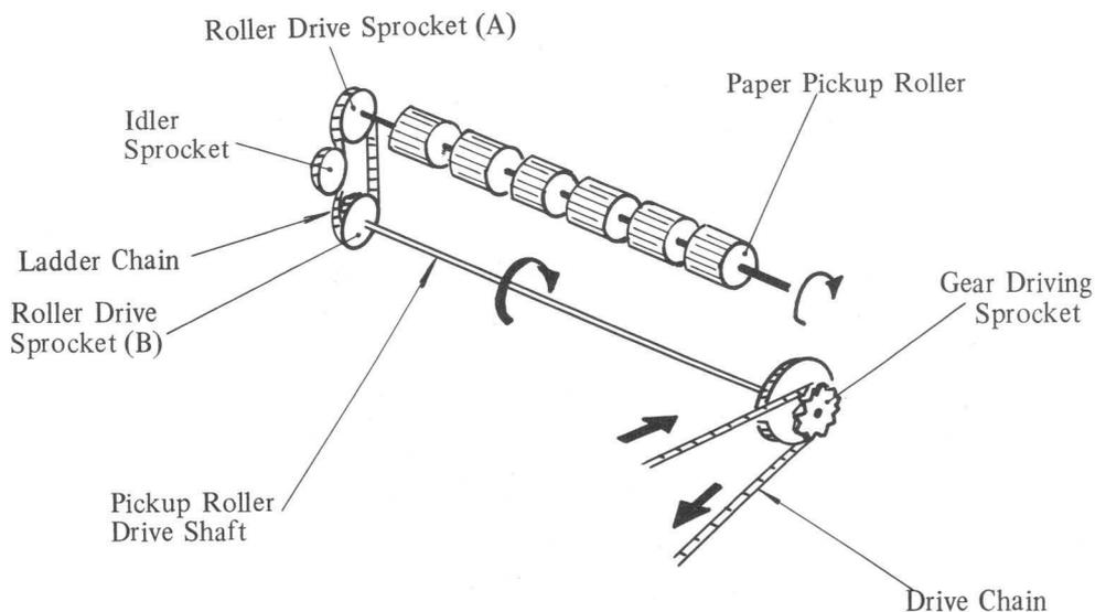
Fig. 4-58 Pickup Roller Rotation Drive
