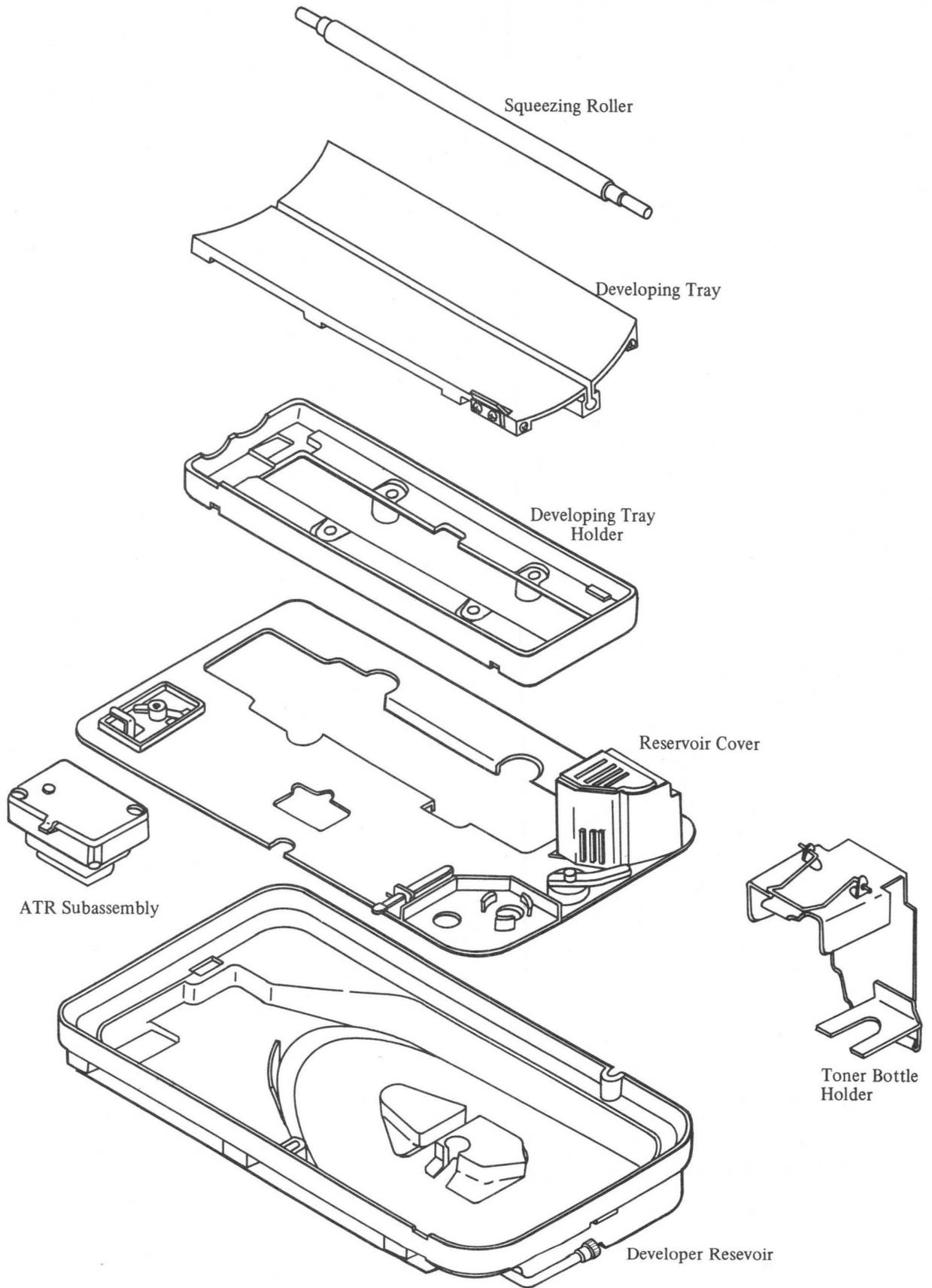
Fig. 4-35 Developer Assembly Main Components
