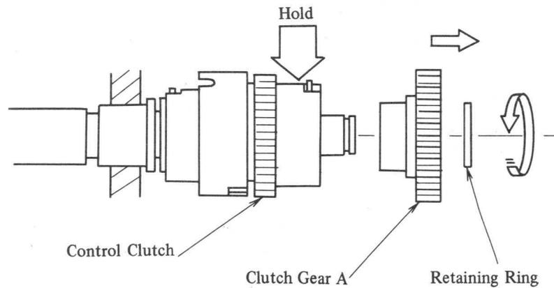
Fig. 4-73 Timing Roller Drive Disassembly (A)
