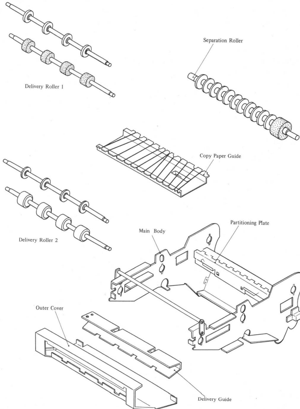
Fig. 4-86 Copy Conveying Assembly Main Components
