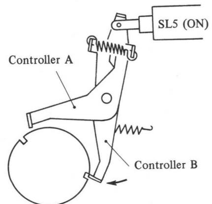
Fig. 4-63 Controller Assembly Operation (B)
