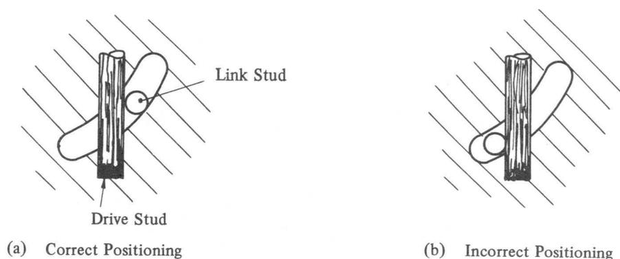
Fig. 4-111 Drive and Link Stud Positioning
