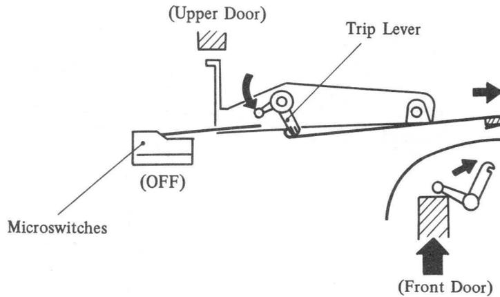
Fig. 4-117 Door Switch Group Operation (B)
