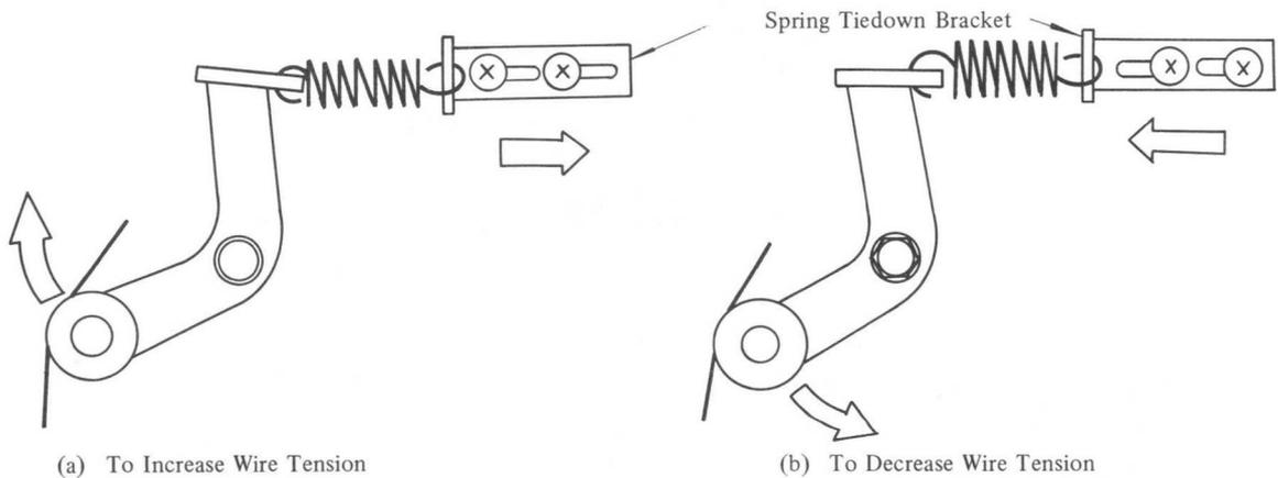
Fig. 4-10 Wire Tension Adjustment
