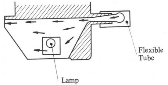
Fig. 4-37 Developer Flow Through ATR Subassembly
