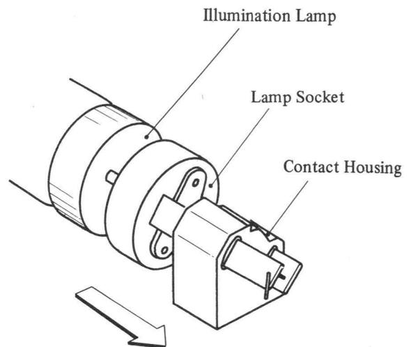
Fig. 4-16 Removal of Lamps
