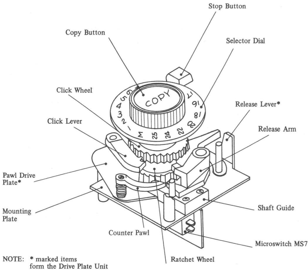
Fig. 4-104 Copy Selector Subassembly Main Components
