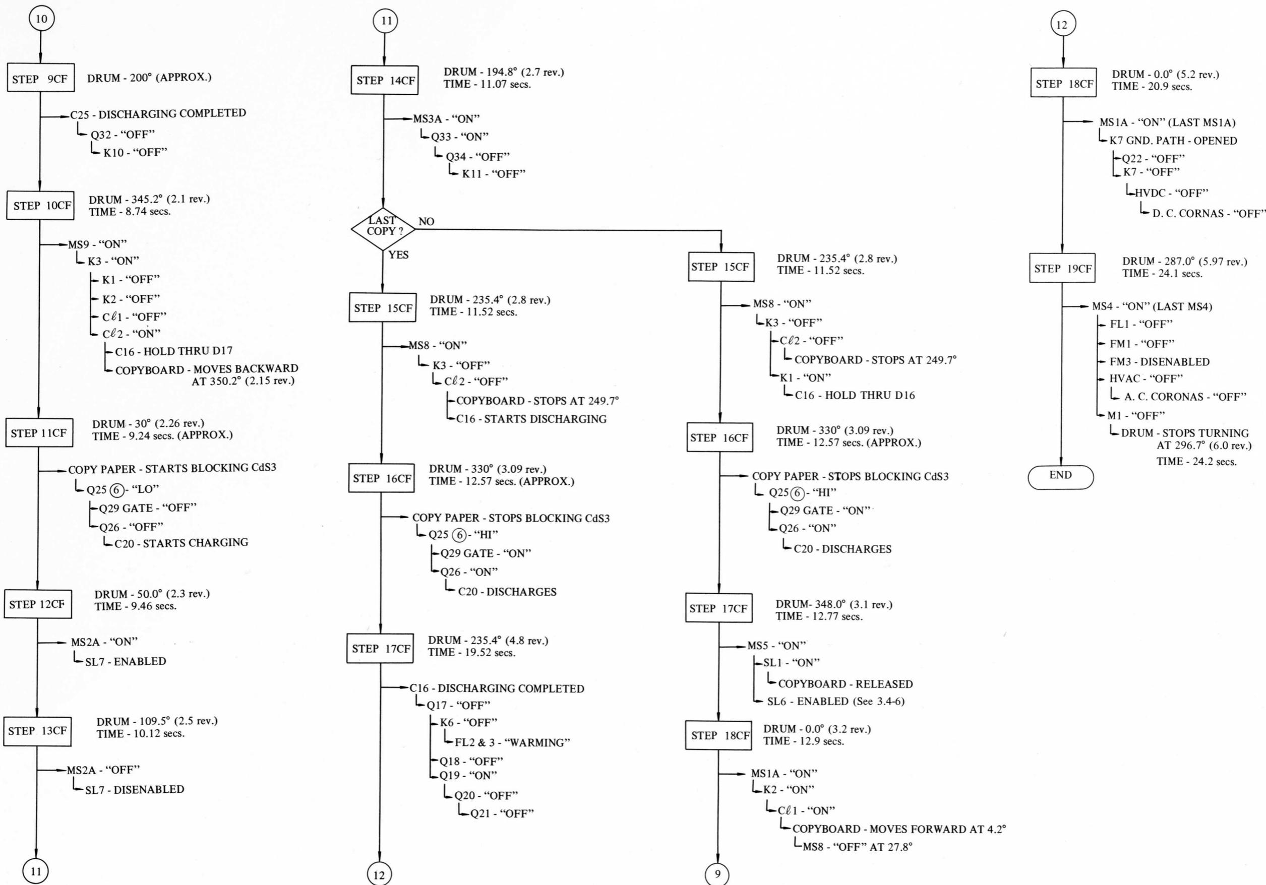
Fig. 3-2 COPY Flowchart (Sheet 3 of 3)
