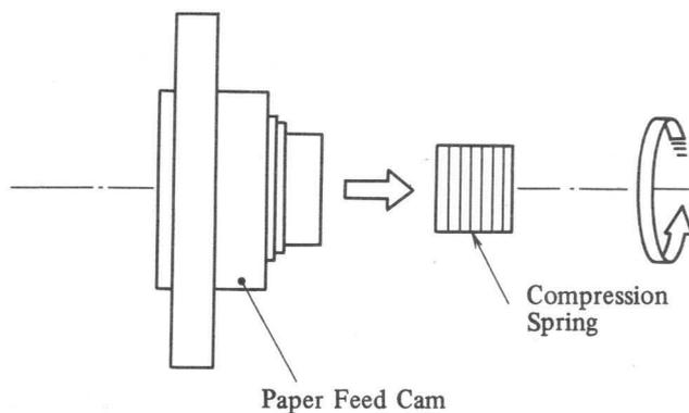
Fig. 4-79 Paper Feed Cam Drive Disassembly (D)
