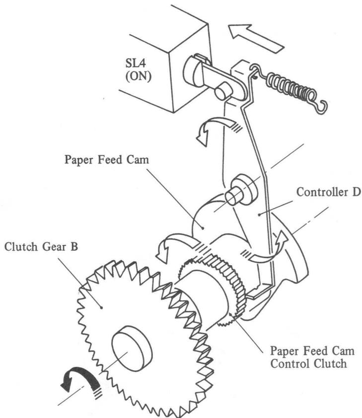
Fig. 4-64 Controller Assembly Operation (C)
