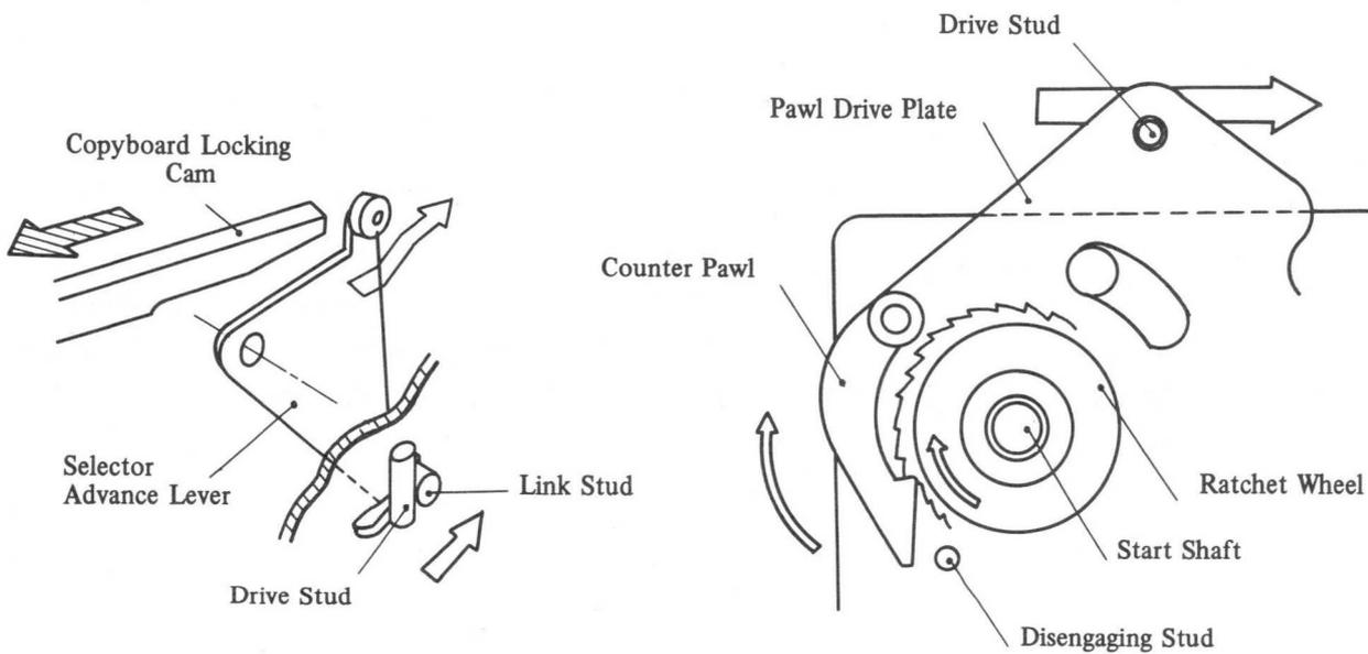
Fig. 4-107 Copy Selector Operation (B)
