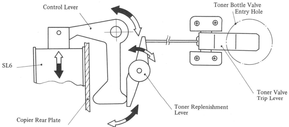
Fig. 4-43 Replenishing Mechanism Main Components
