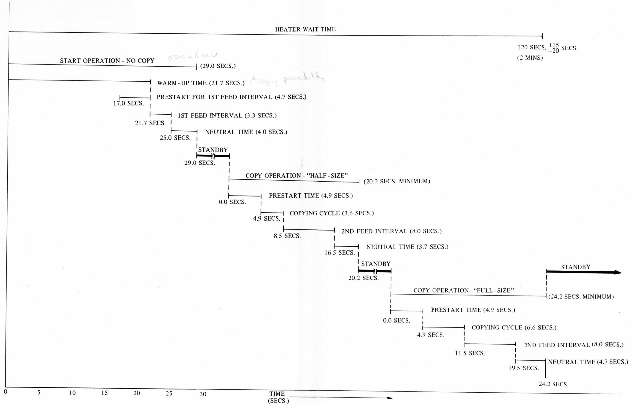
Fig. 3-4 Significant Operation Times
