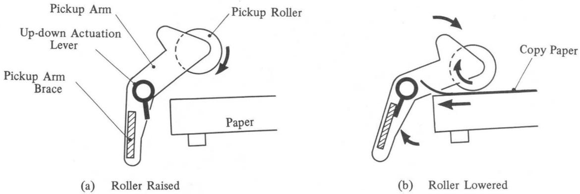
Fig. 4-60 Pickup Roller Up-Down Drive
