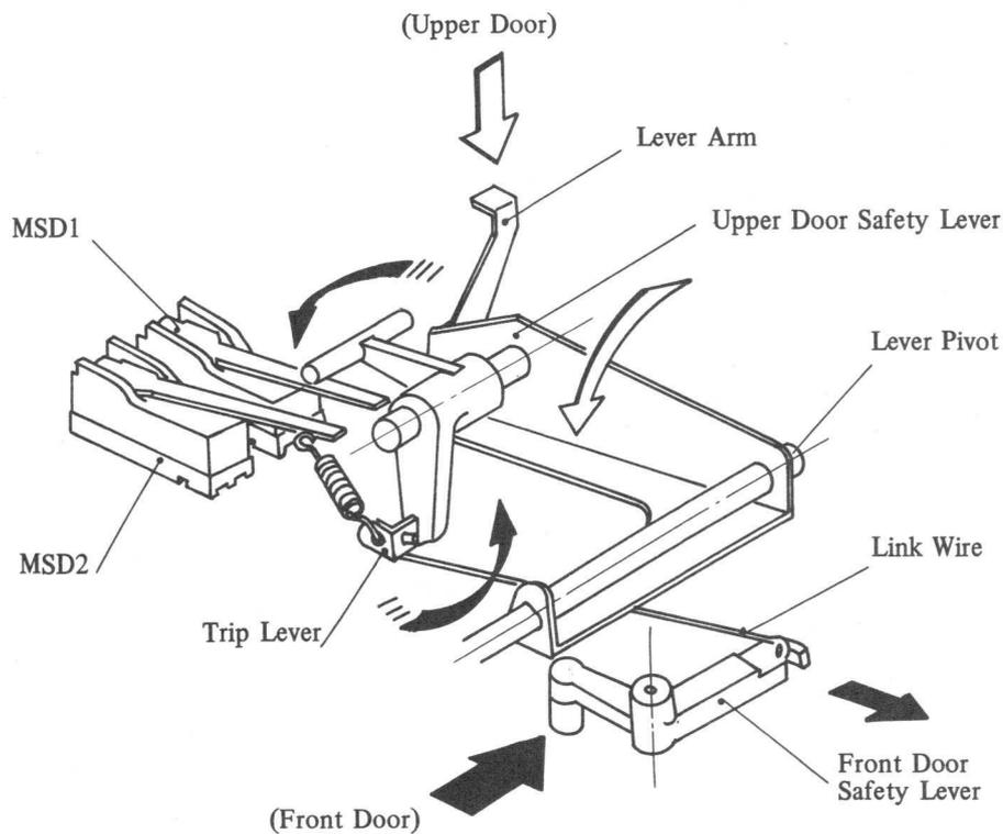
Fig. 4-115 Door Switch Group Main Components
