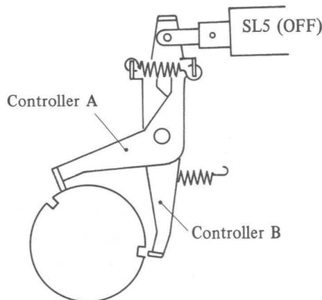
Fig. 4-65 Controller Assembly Operation (D)
