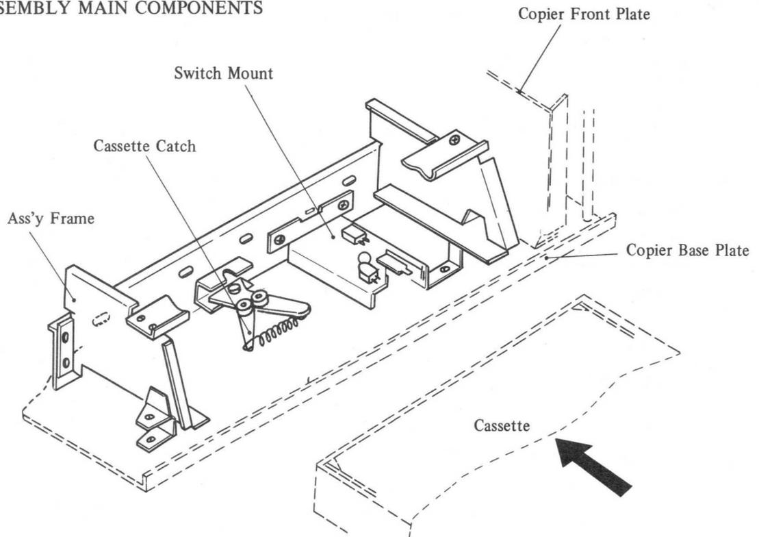
Fig. 4-56 Cassette Holder Assembly Main Components
