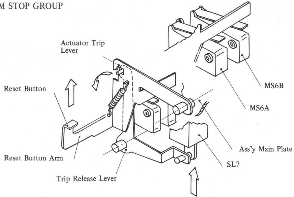
Fig. 4-120 Jam Stop Group Main Components
