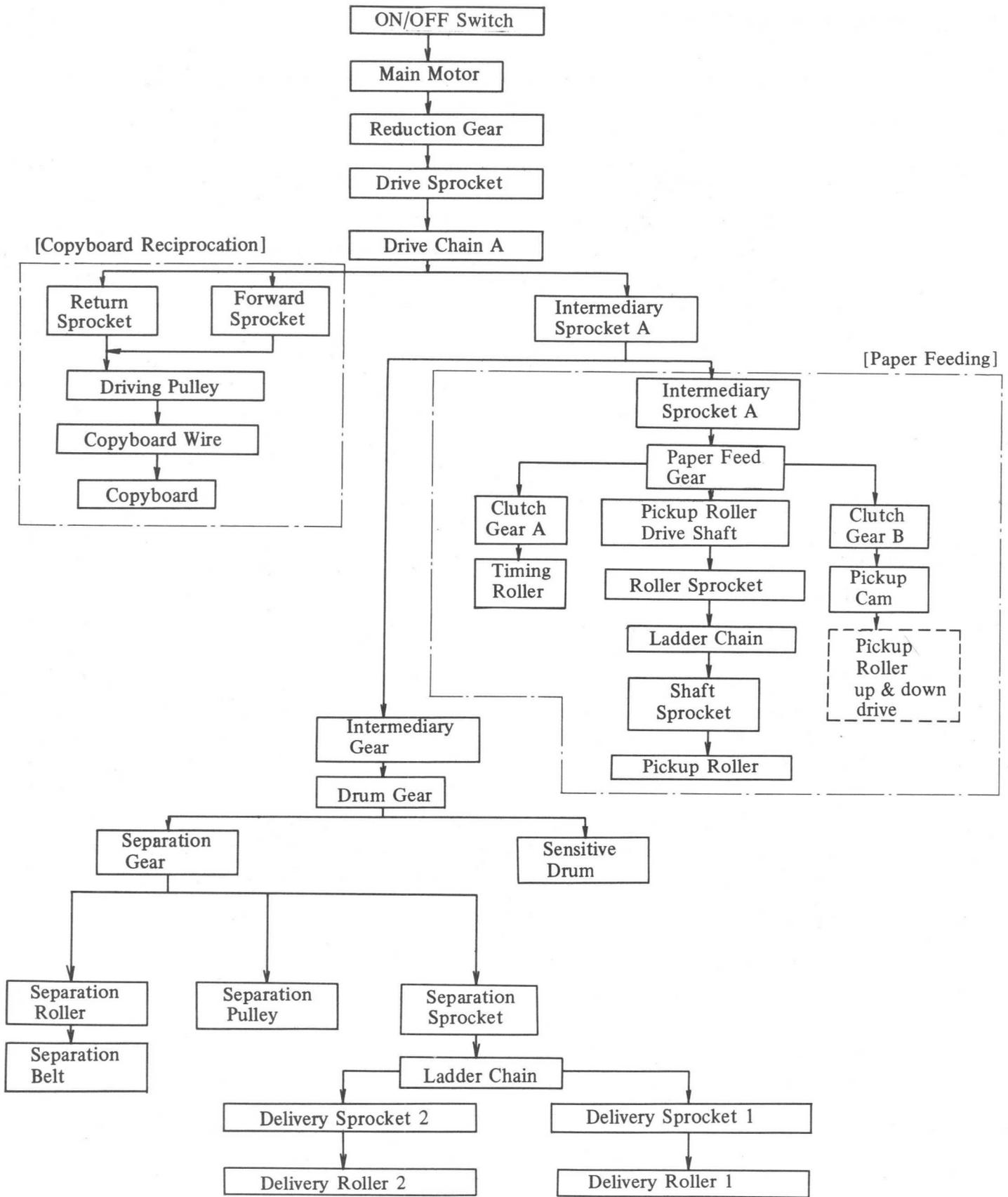
Fig. 2-5 Block Diagram of the Drive System
