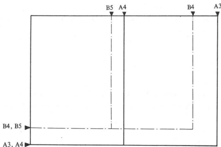
Fig. 1-3 Original Positioning on Copyboard
