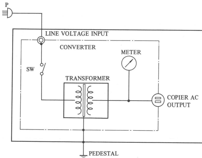
Fig. 3-26 Voltage Adapter Pedestal - Schematic Diagram
