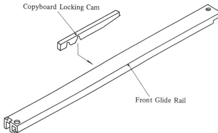
Fig. 4-2 Front Rail Components
