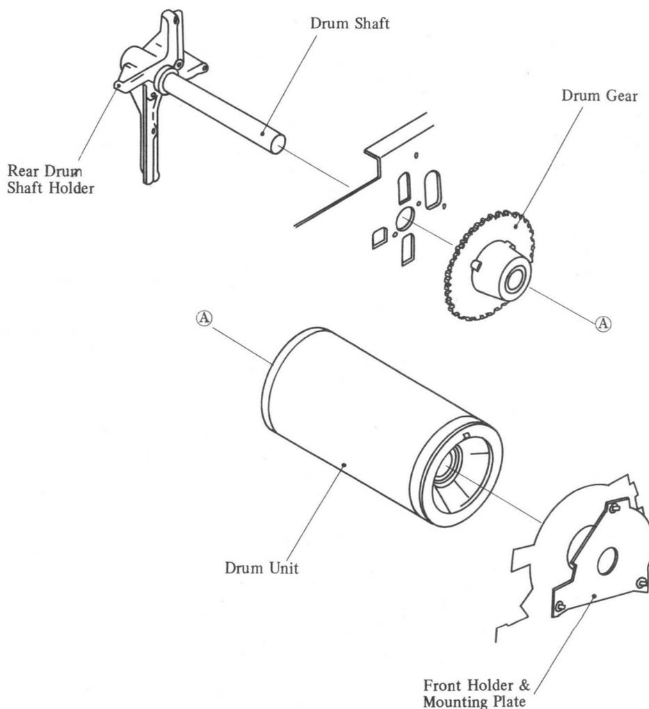
Fig. 4-25 Drum Assembly Main Components
