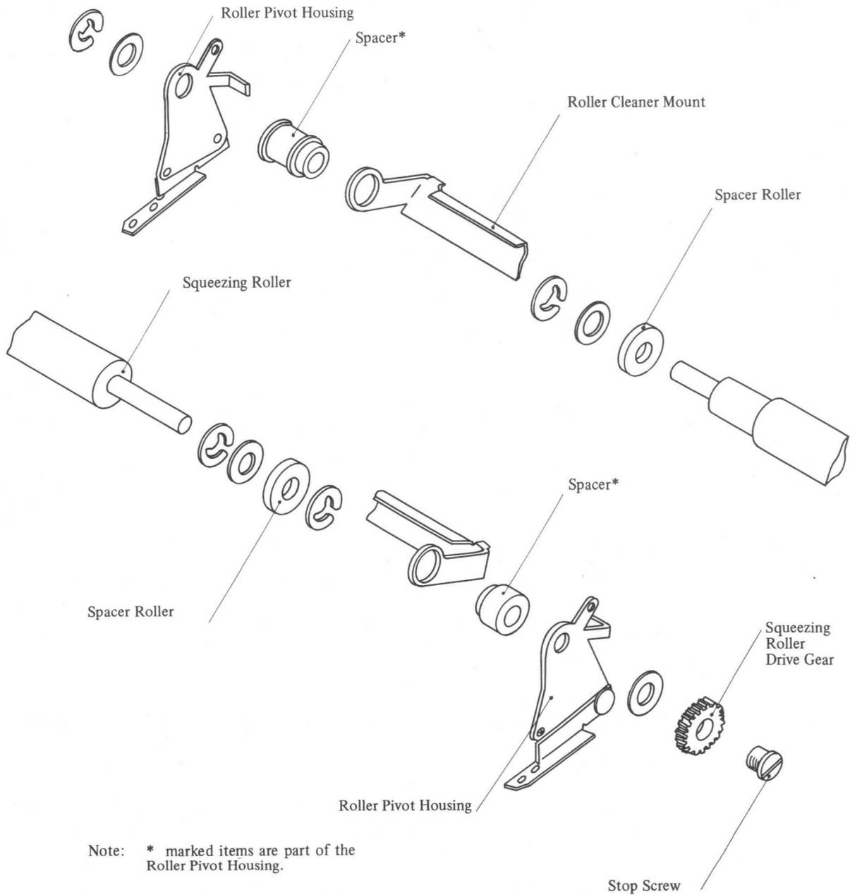
Fig. 4-48 Components of Squeezing Roller (Detailed)
