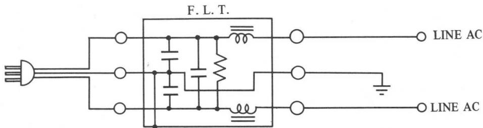
Fig. 3-5 Low-Pass Filter—Schematic Diagram
