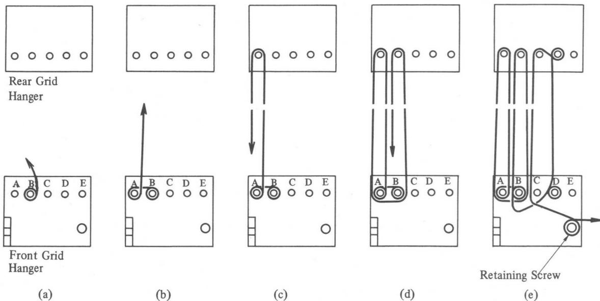
Fig. 4-33 Wiring Procedure
