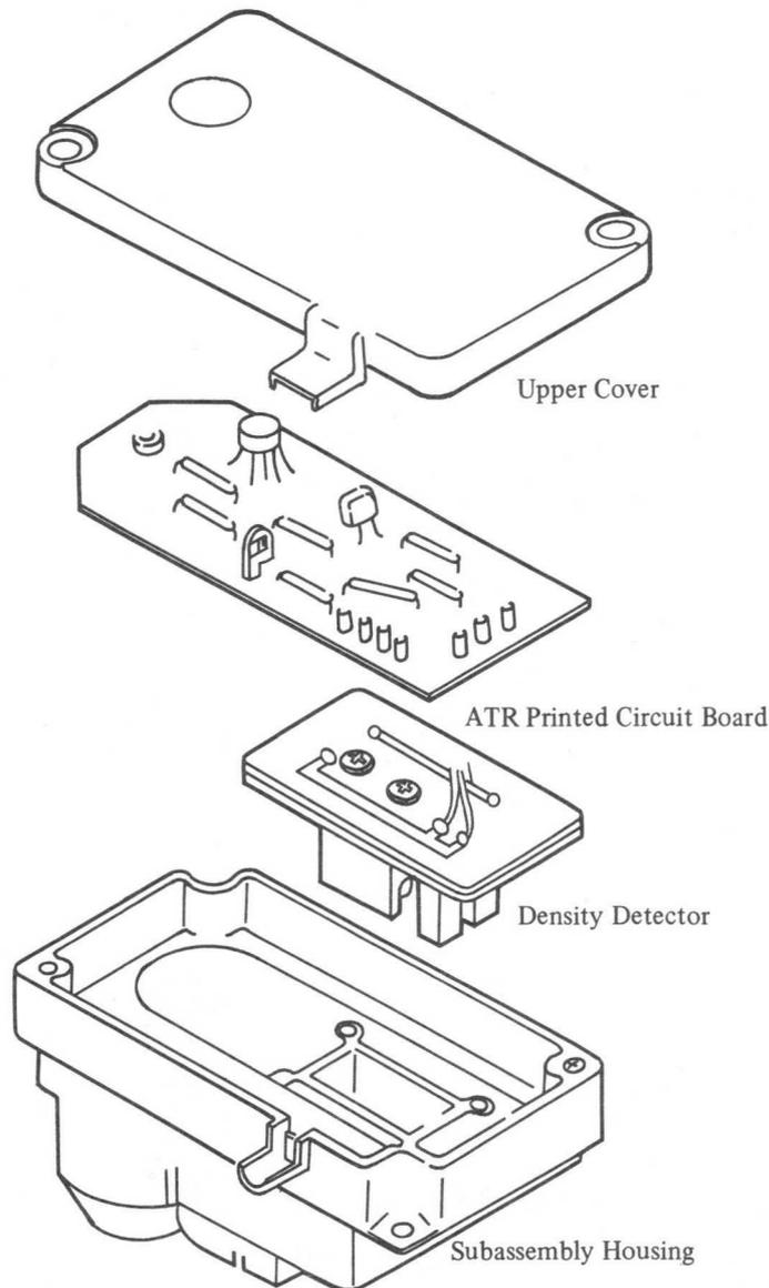
Fig. 4-36 ATR Subassembly Main Components
