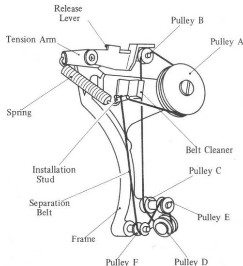
Fig. 4-97 Paper Separating Subassembly Main Components
