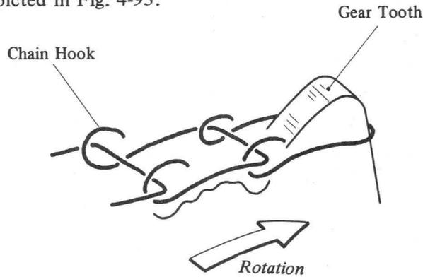
Fig. 4-93 Correct Chain Positioning
