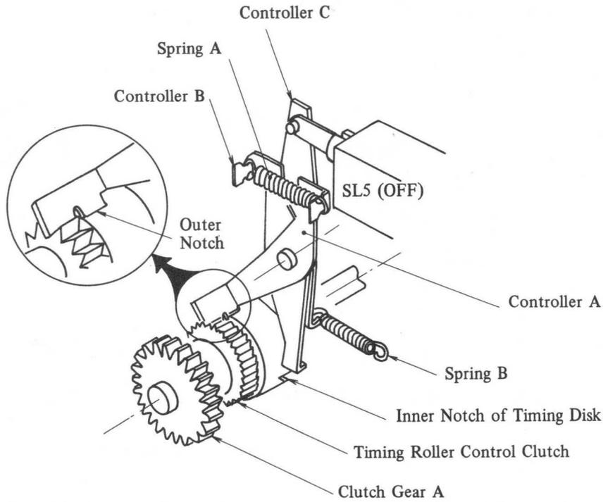
Fig. 4-66 Controller Assembly Operation (E)
