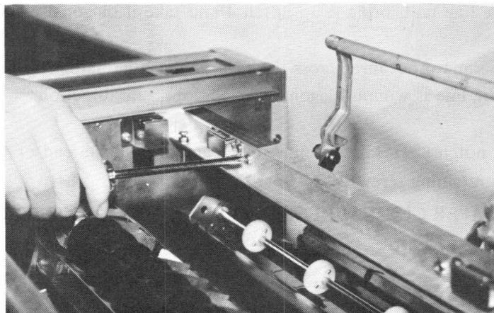
Fig. 4-29 Eliminator Assembly Removal
