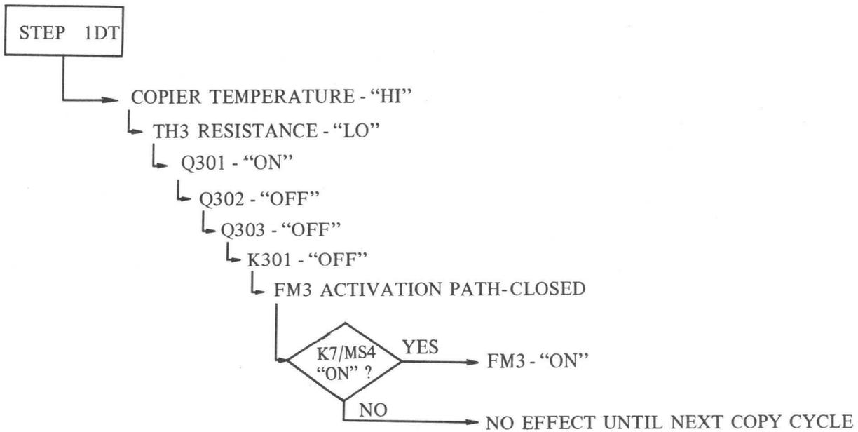
Fig. 3-15 Developer Cooling Flowchart
