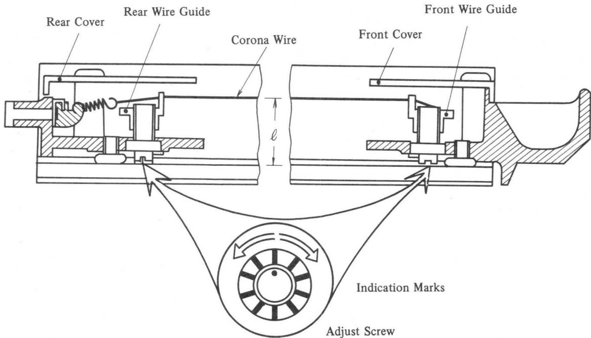
Fig. 4-34 Corona Wire Adjustment
