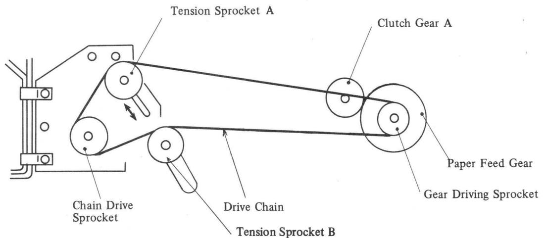
Fig. 4-71 Drive Chain Removal
