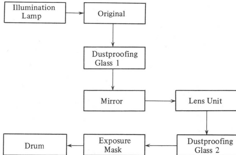
Fig. 4-17 Block Diagram of Light Travel
