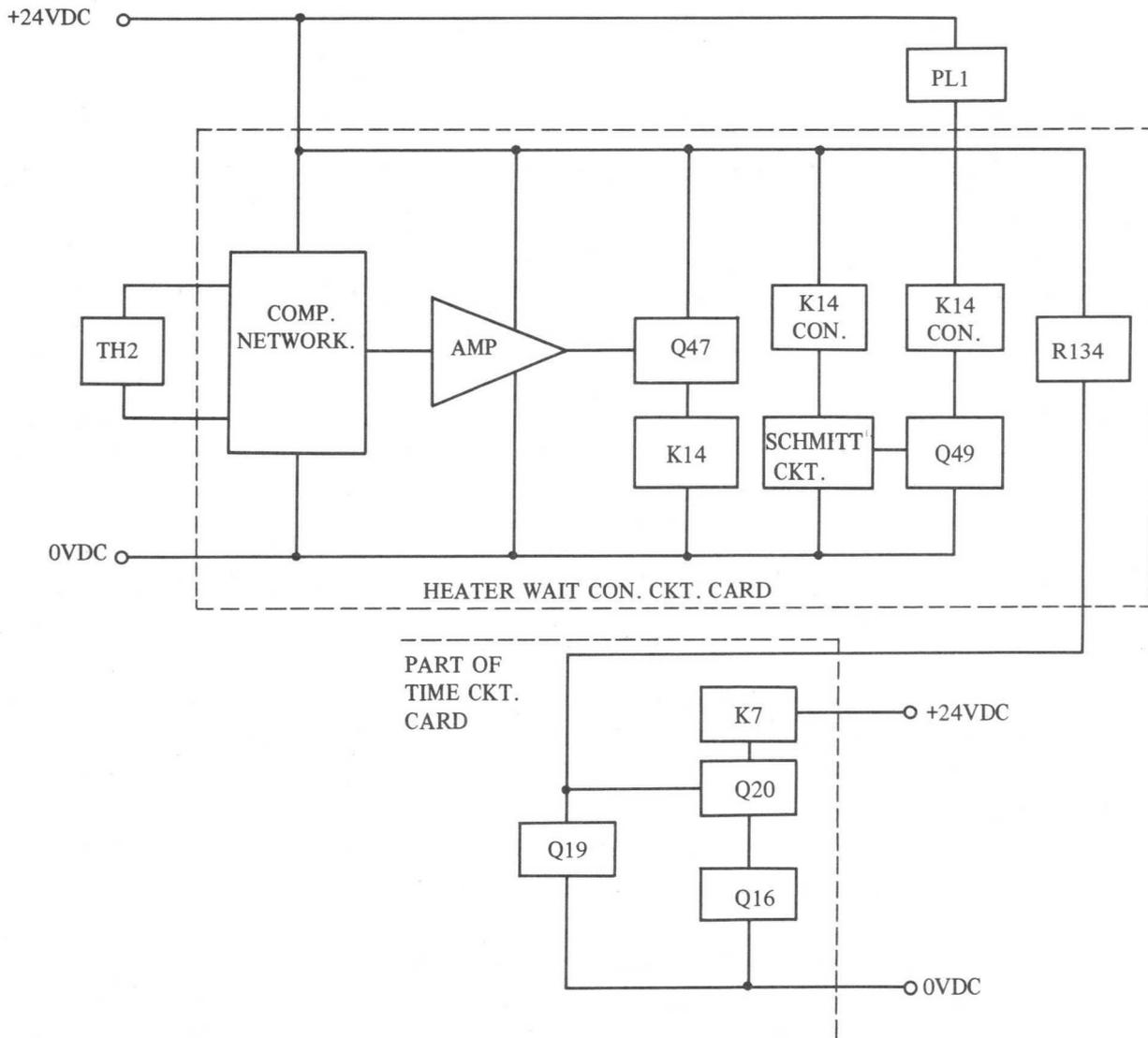
Fig. 3-9 Heater Wait Control Circuit & Associated Components
