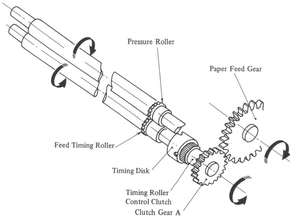
Fig. 4-61 Timing Roller Drive Components
