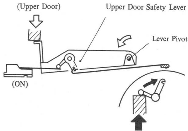
Fig. 4-118 Door Switch Group Operation (C)
