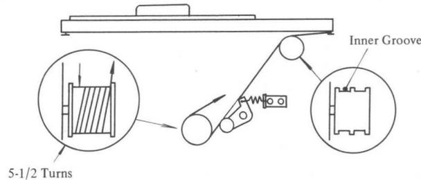
Fig. 4-6 Copyboard Wire Installation (B)
