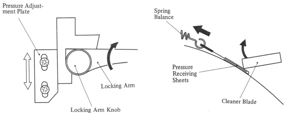
Fig. 4-54 Adjustment of Cleaner Blade Pressure (A)
