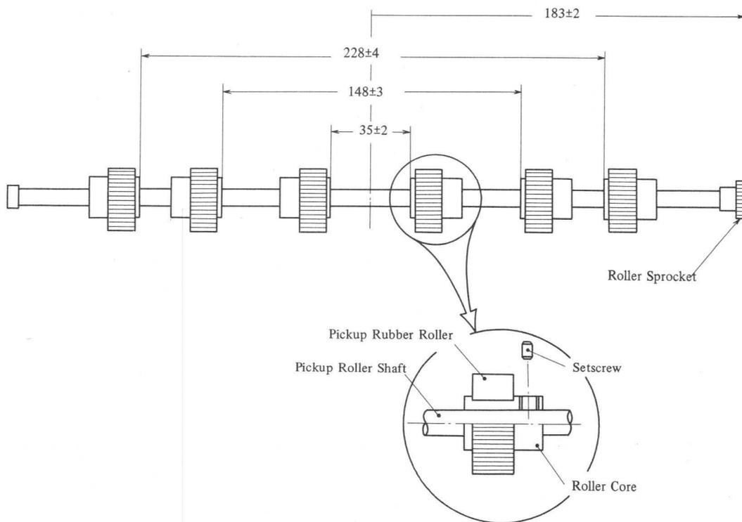
Fig. 4-81 Pickup Roller Spacing
