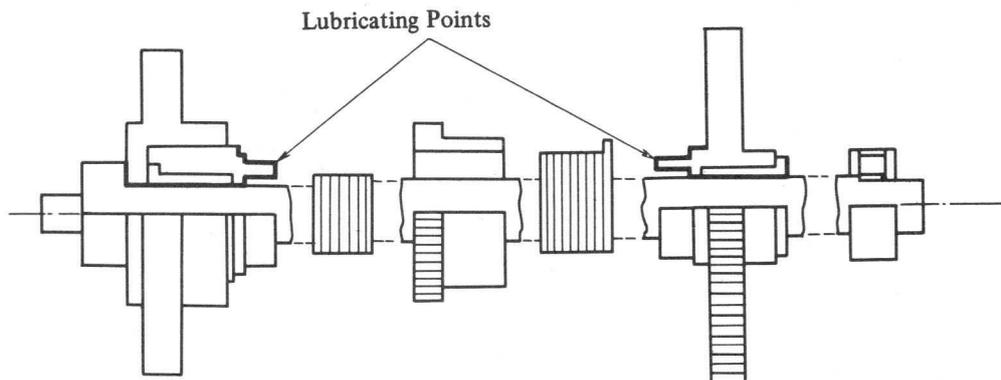
Fig. 4-84 Paper Feed Cam Drive Lubrication
