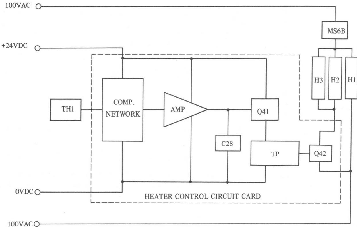
Fig. 3-19 Heater Control Circuit & Associated Components
