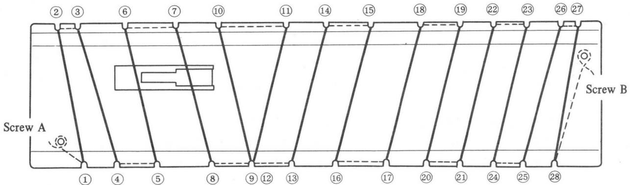
Fig. 4-92 Copy Paper Guide Lacing Pattern
