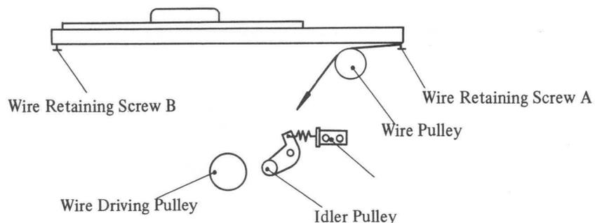
Fig. 4-5 Copyboard Wire Installation (A)
