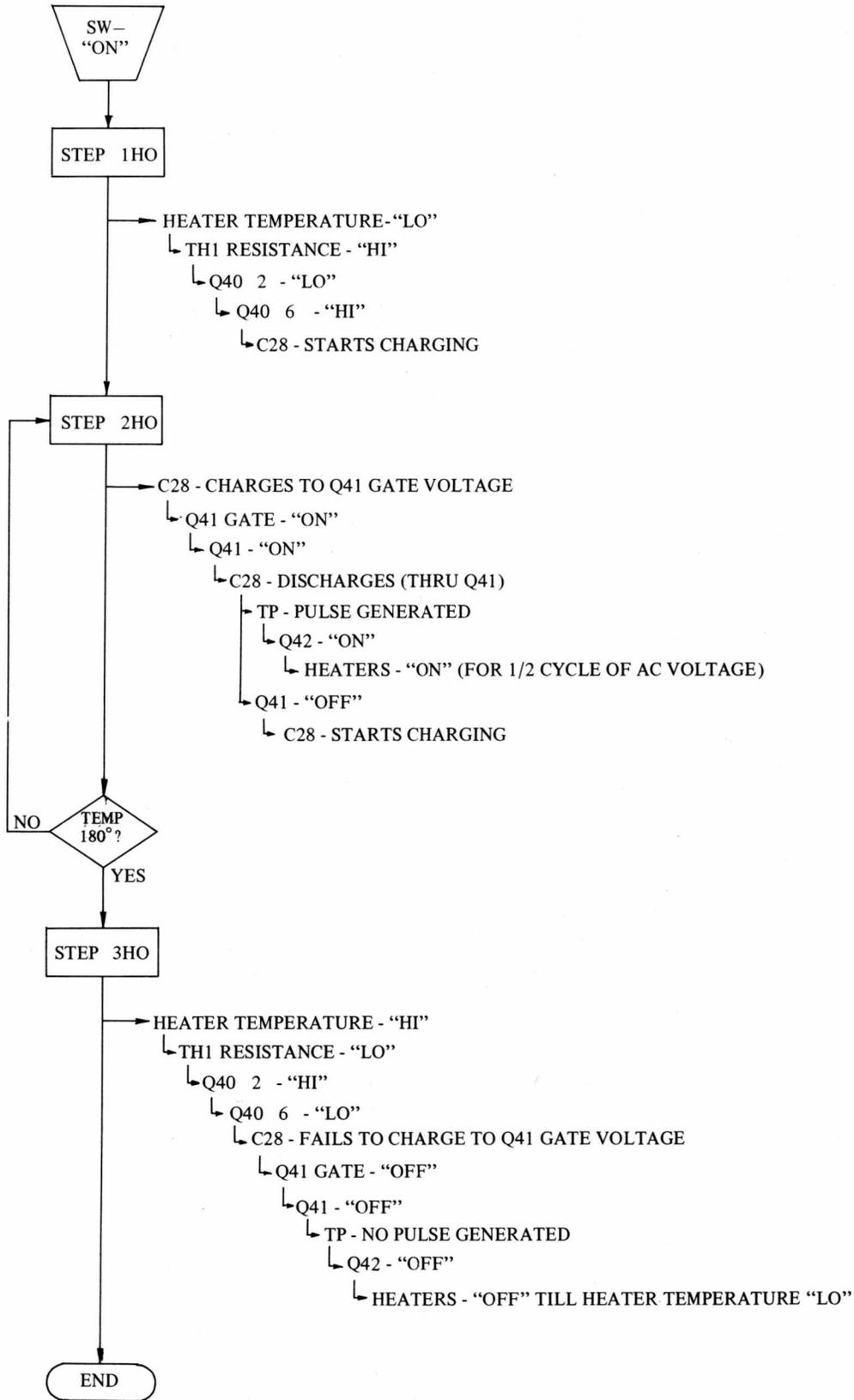
Fig. 3-20 Heater Operation Flowchart
