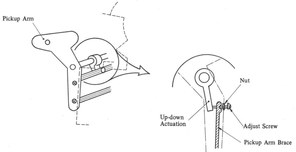
Fig. 4-83 Pickup Roller Height Adjustment
