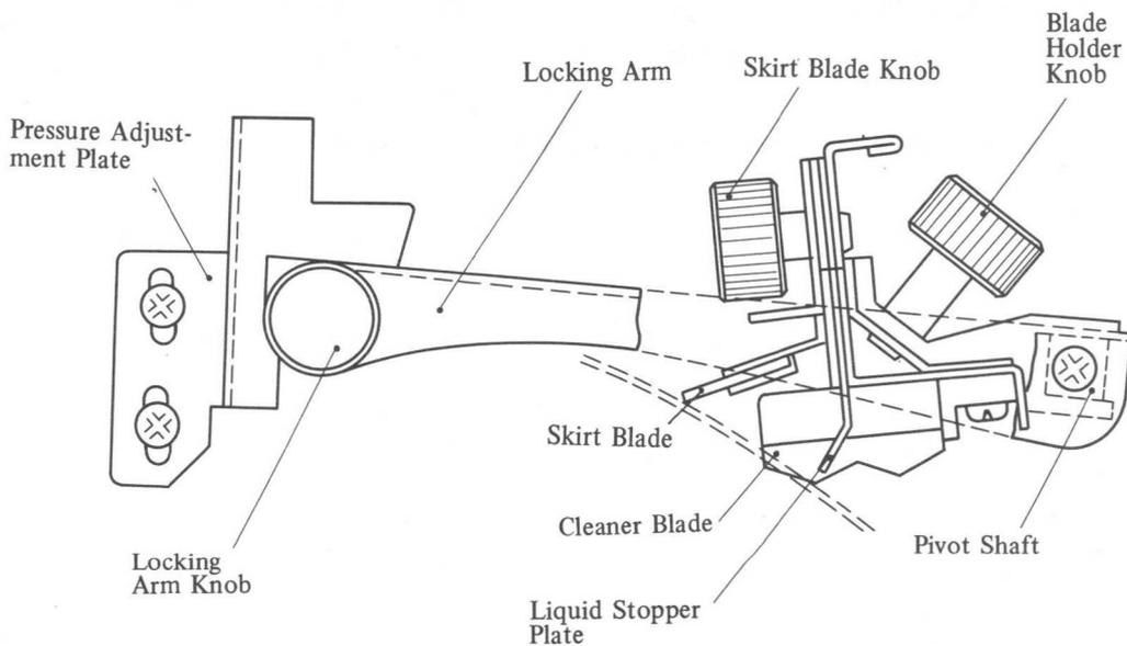
Fig. 4-52 Drum Cleaner Assembly Main Components (from Copier Front)
