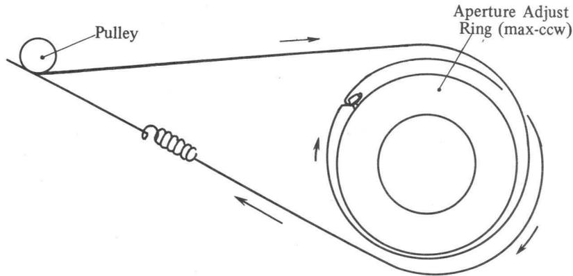
Fig. 4-22 Adjust Line Replacement (C)
