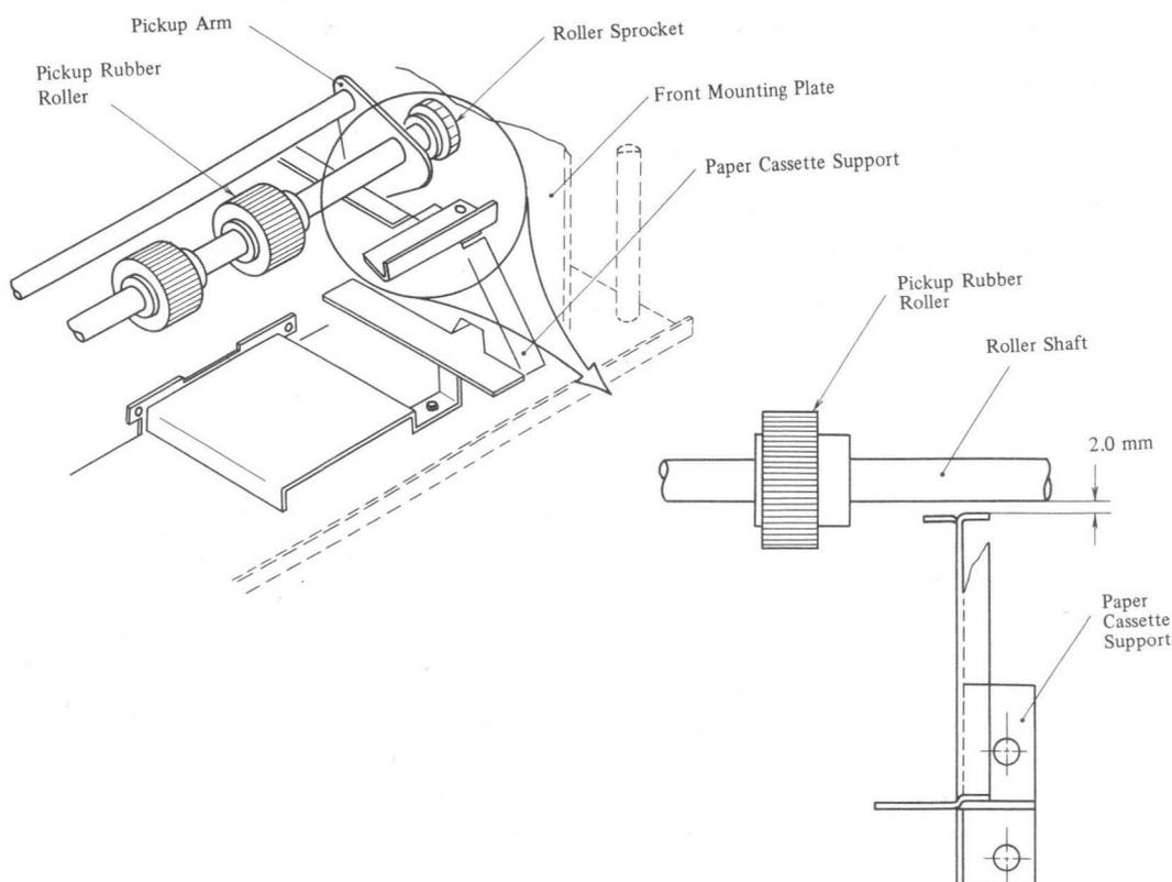
Fig. 4-82 Pickup Roller Height
