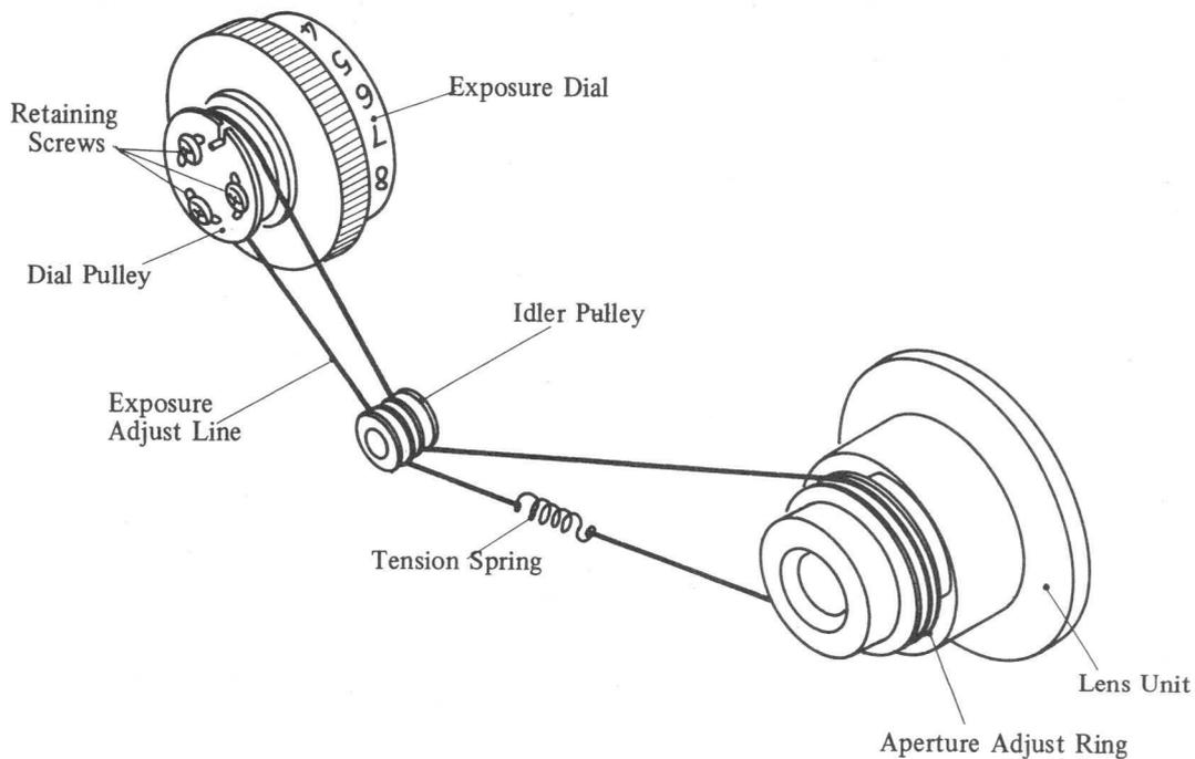
Fig. 4-23 Adjust Line Replacement (D)
