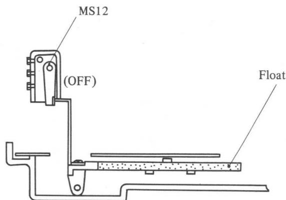
Fig. 4-45 Normal Developer Level
