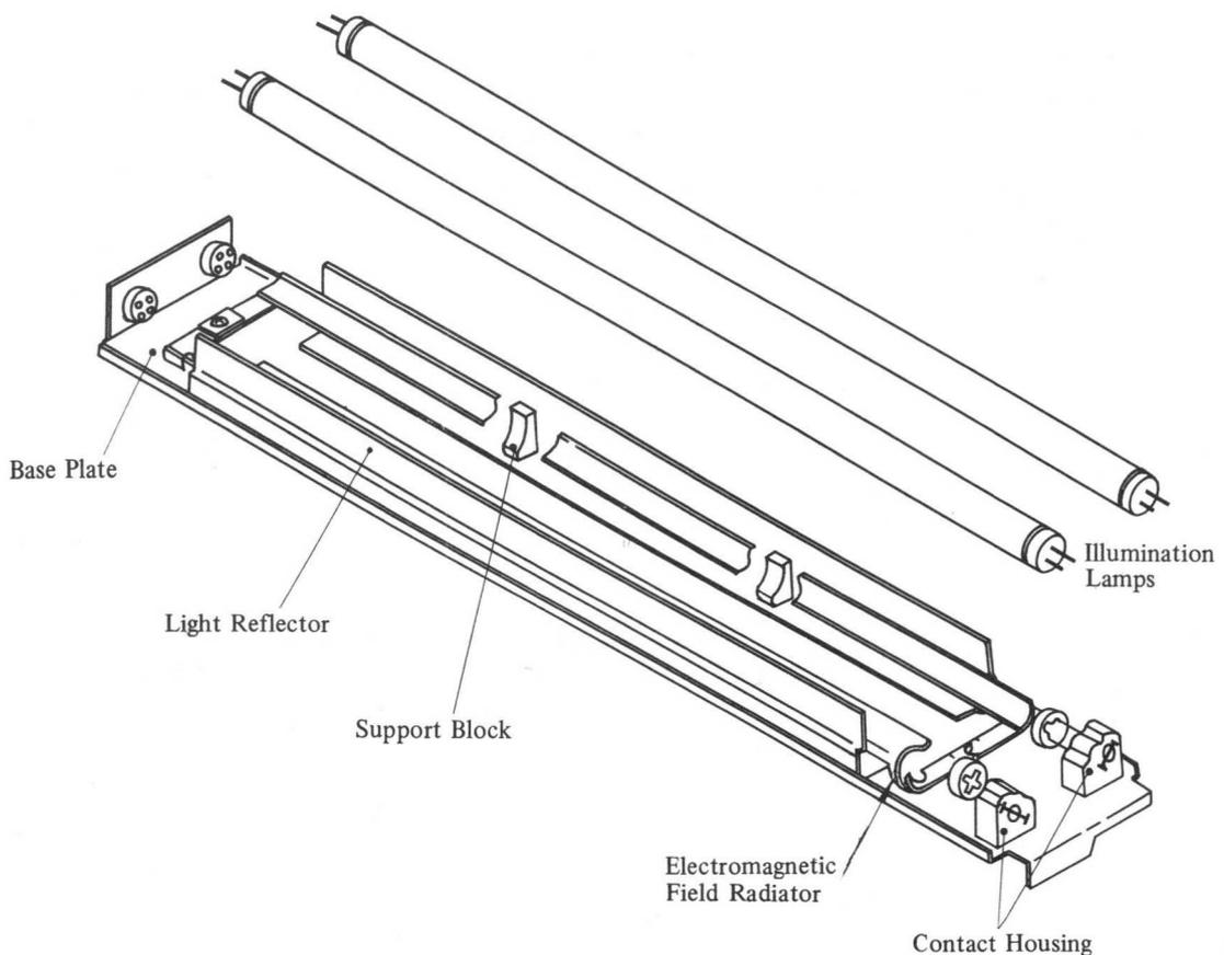
Fig. 4-13 Illumination Assembly Main Components
