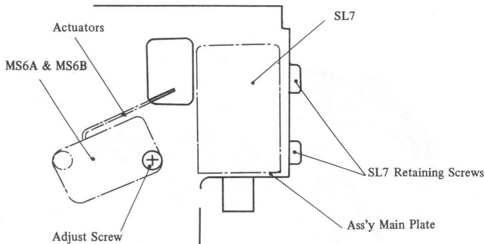
Fig. 4-124 Jam Stop Group Adjustments
