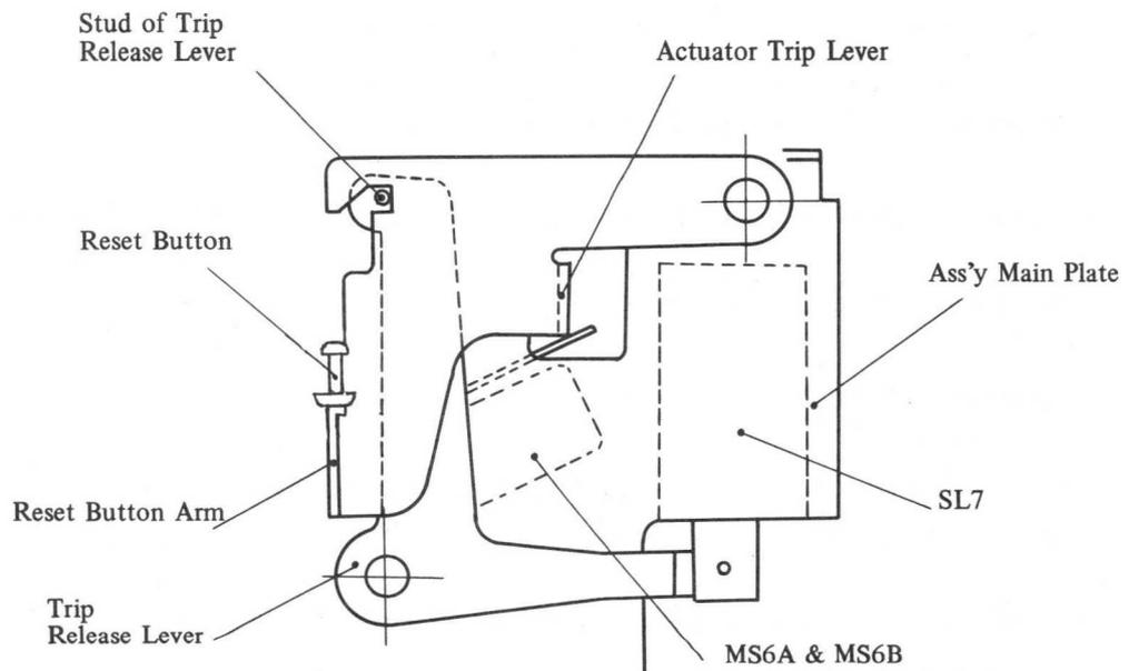
Fig. 4-121 Jam Stop Group Operation (A)
