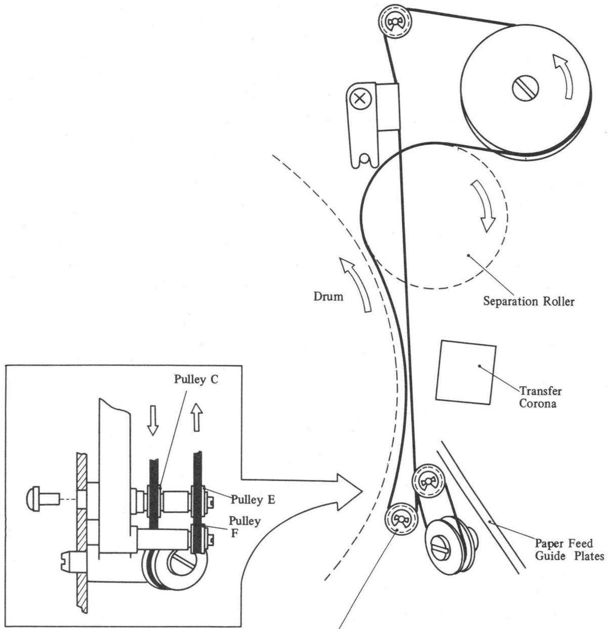
Fig. 4-96 Movement of Separation Belt (from copier rear)
