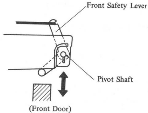
Fig. 4-123 Adjustment of Front Safety Lever
