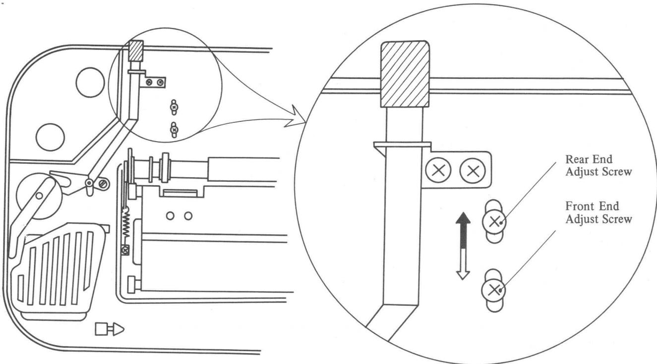
Fig. 4-50 Squeezing Roller Adjustment
