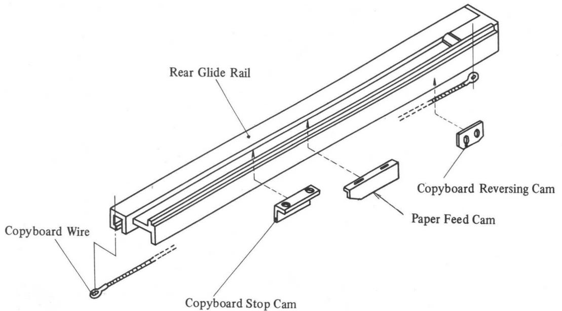
Fig. 4-3 Rear Rail Components
