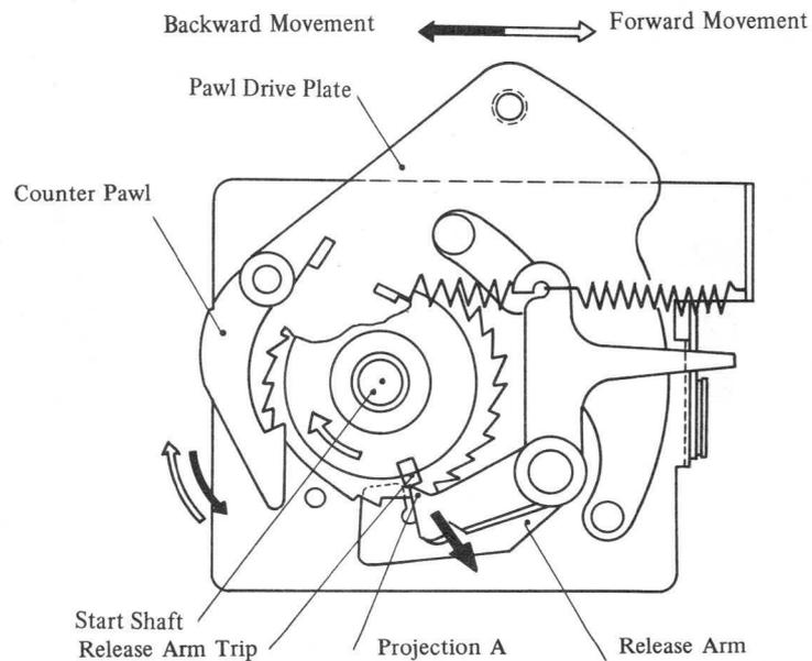
Fig. 4-109 Copy Selector Operation (D)
