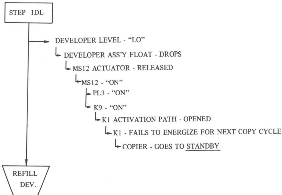
Fig. 3-13 "Developer Low" Flowchart
