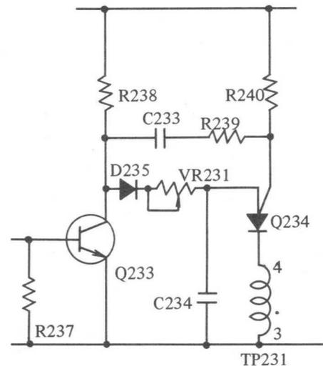
Fig. 3-22 1/4 Zero-Cross Circuit
