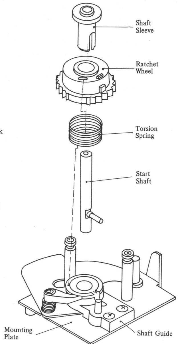
Fig. 4-112 Copy Selector Reassembly
