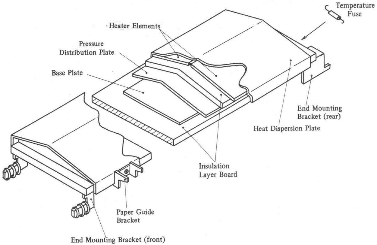
Fig. 4-98 Heater Assembly Bracket (front)
