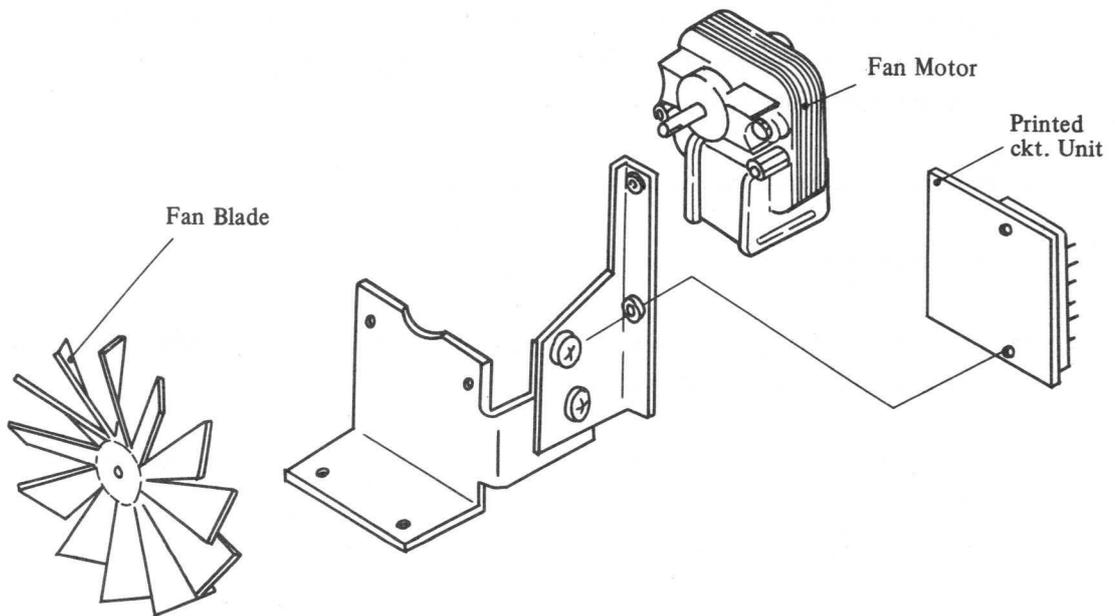
Fig. 4-102 Fan Assembly Main Components
