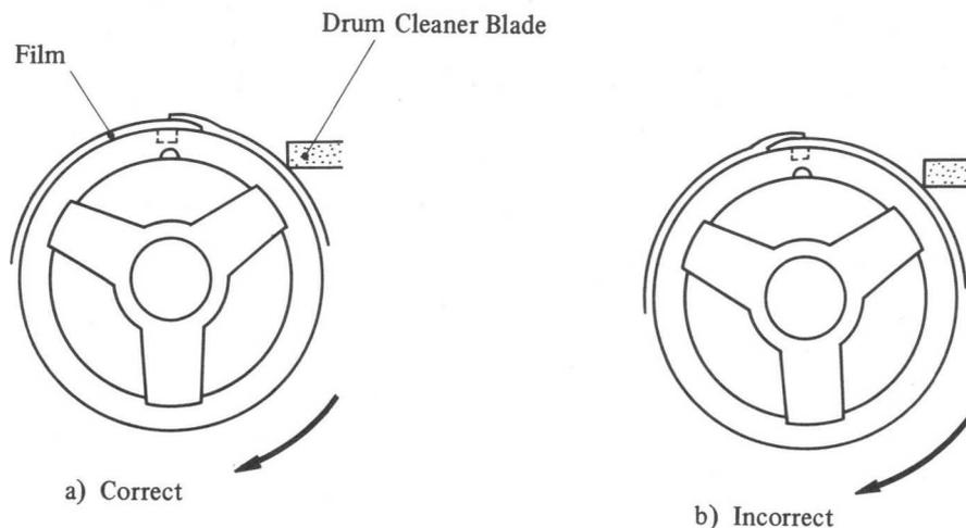
Fig. 4-27 Drum Position in Copier (from copier front)
