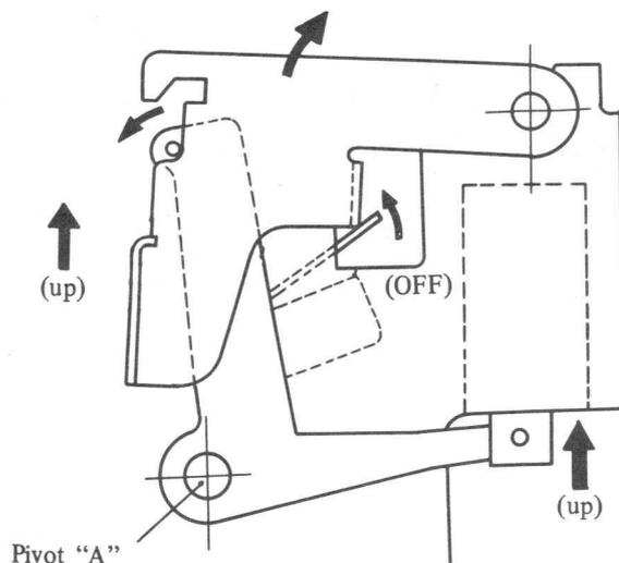
Fig. 4-122 Jam Stop Group Operation (B)
