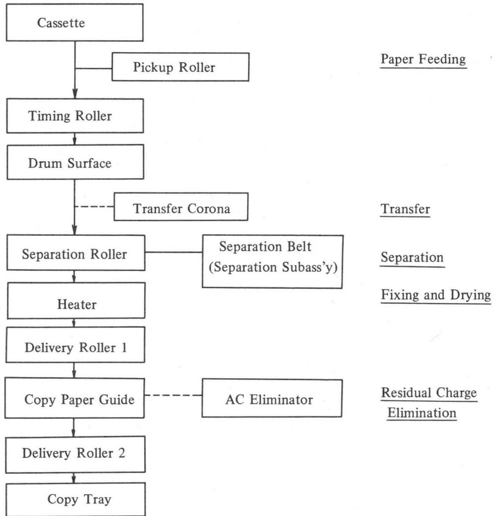
Fig. 2-9 Diagram of Copy Paper Movement
