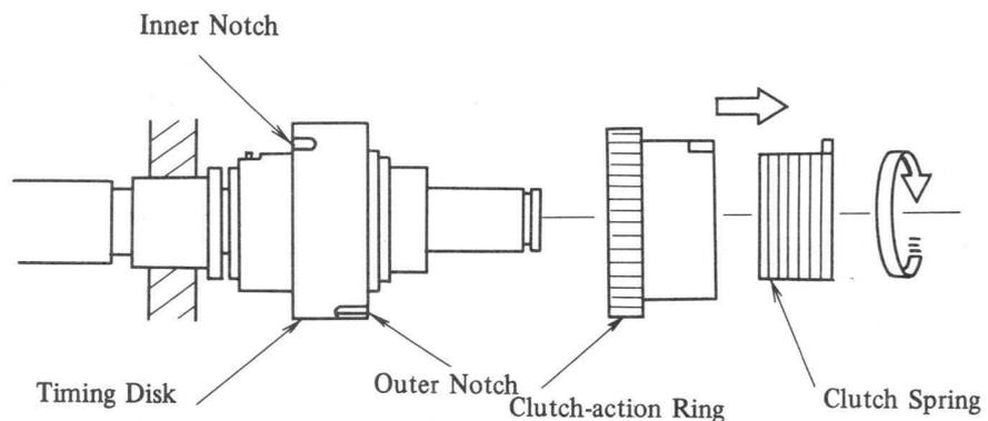
Fig. 4-74 Timing Roller Drive Disassembly (B)
