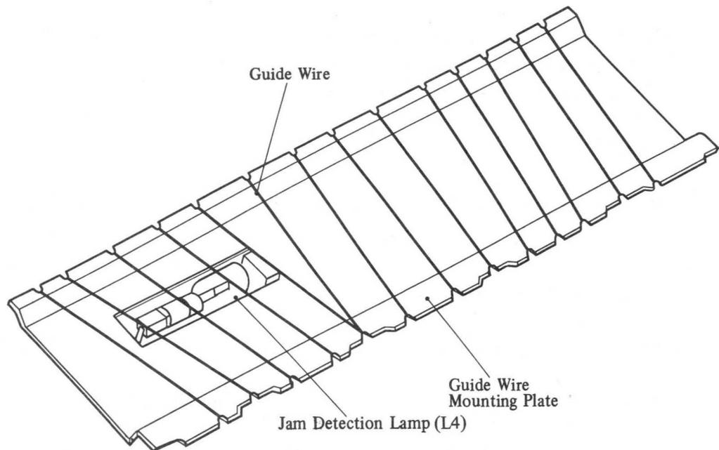
Fig. 4-88 Copy Paper Guide and Jam Detection Lamp
