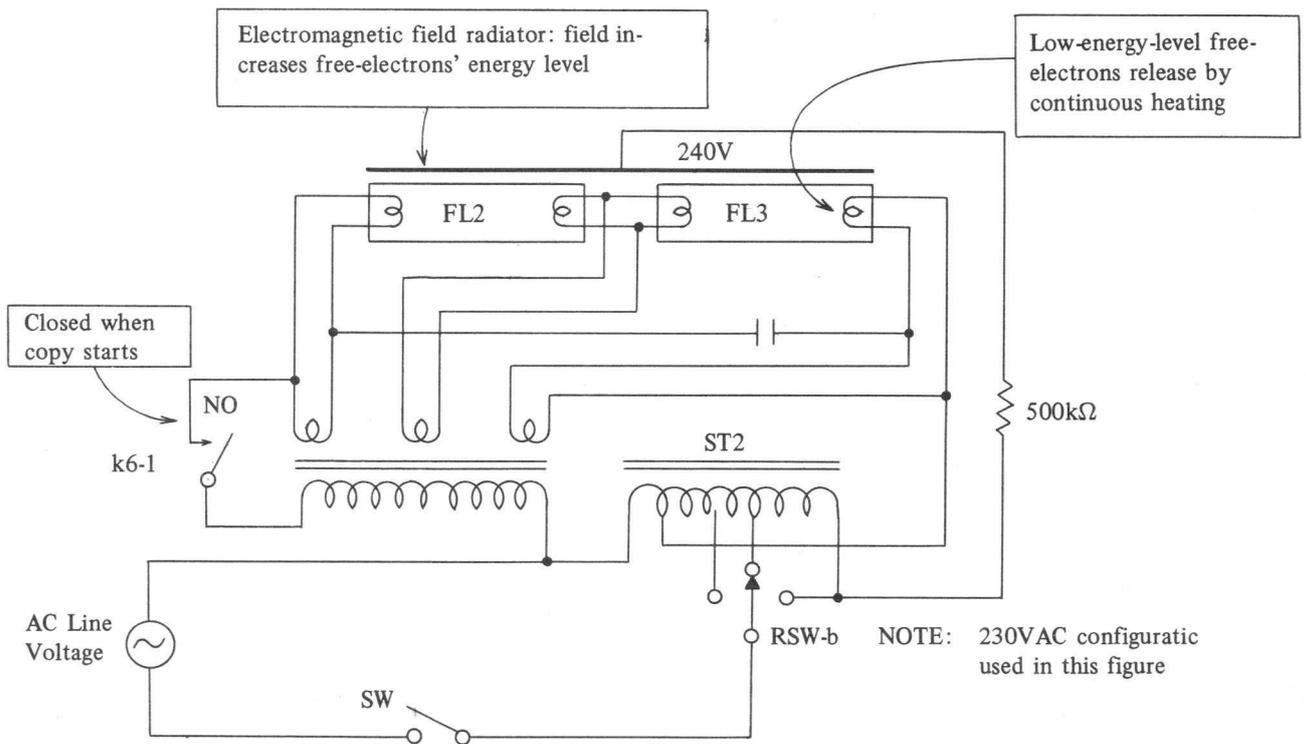
Fig. 3-8 Original Illumination Circuit
