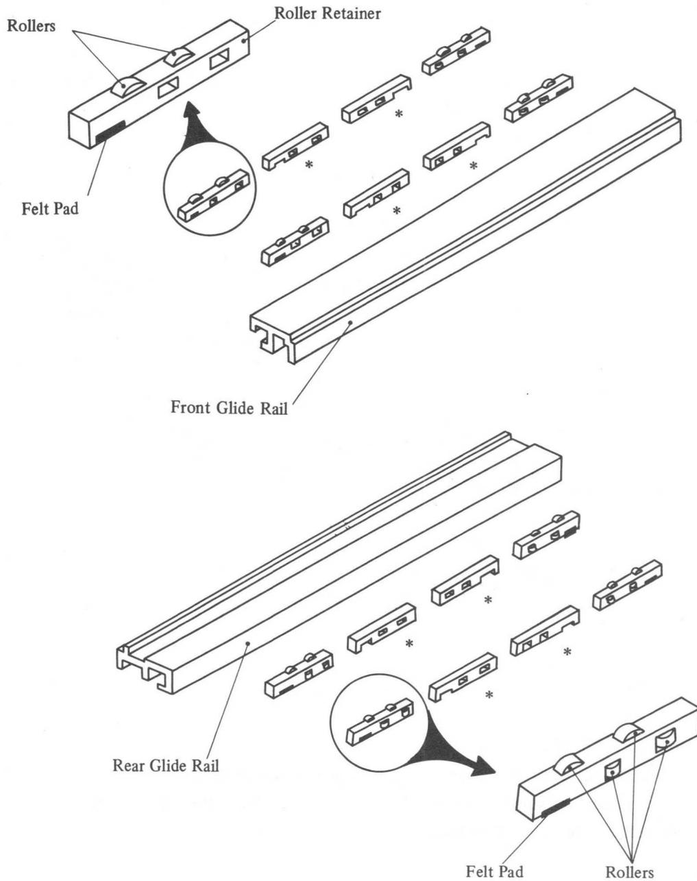
Fig. 4-4 Roller Unit Positioning
