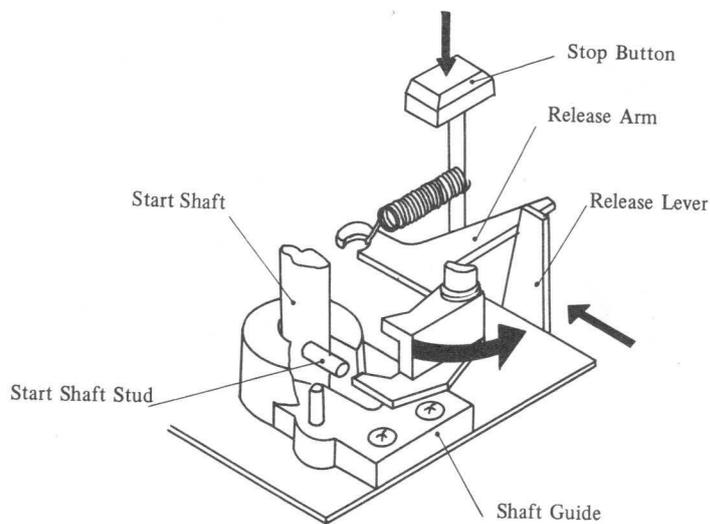
Fig. 4-110 Stop Button Operation
