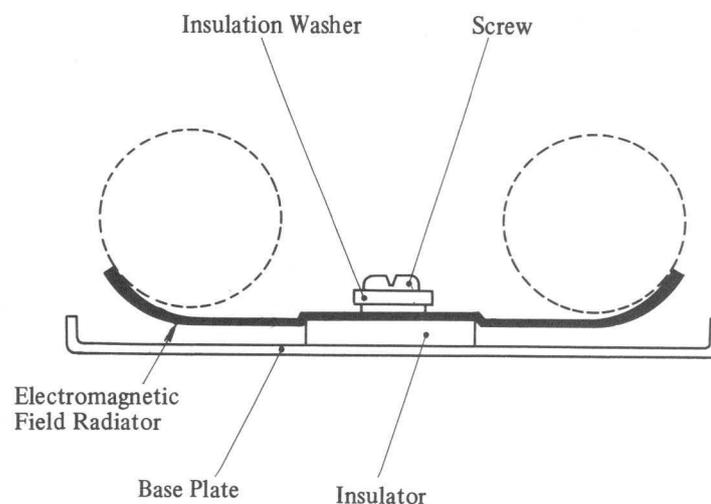
Fig. 4-15 Electromagnetic Field Radiator Mounting
