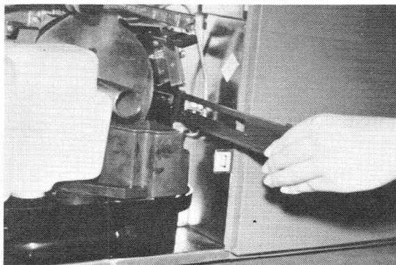
Fig. 4-19 Exposure Mask Removal
