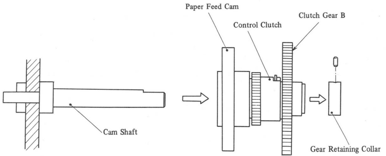
Fig. 4-76 Paper Feed Cam Drive Disassembly (A)
