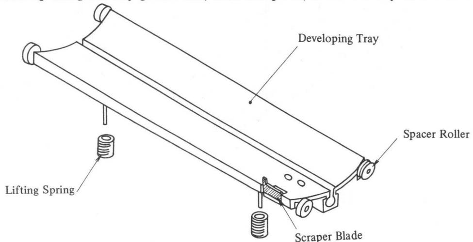
Fig. 4-39 Developing Tray Main Components
