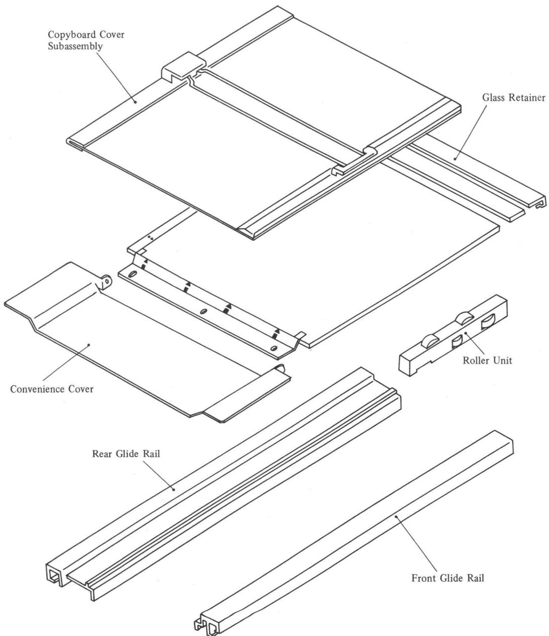
Fig. 4-1 Copyboard Assembly Main Components
