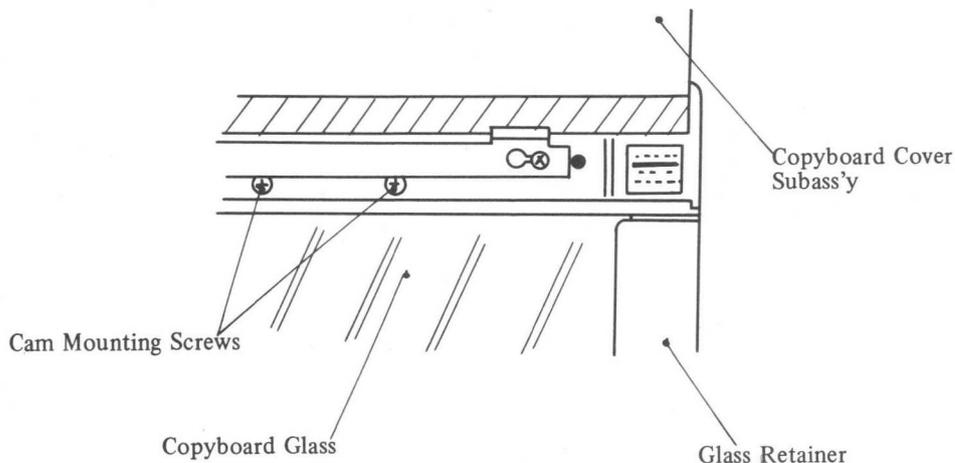
Fig. 4-11 Location of Paper Feed Cam
