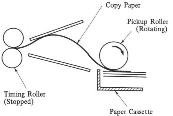
Fig. 4-67 Controller Assembly Operation (F)
