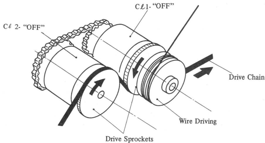
Fig. 4-125 Driving Mechanism Operation (A)
