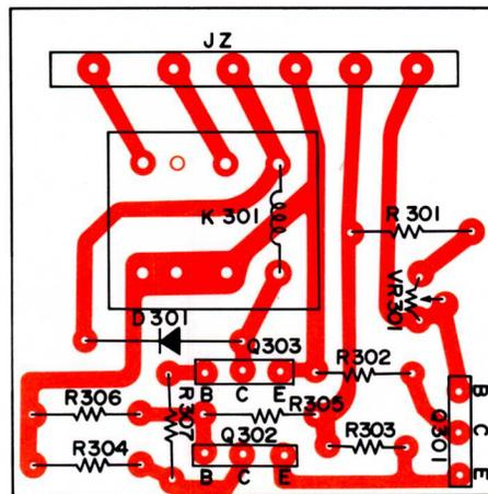
Developer Temperature Control Circuit
