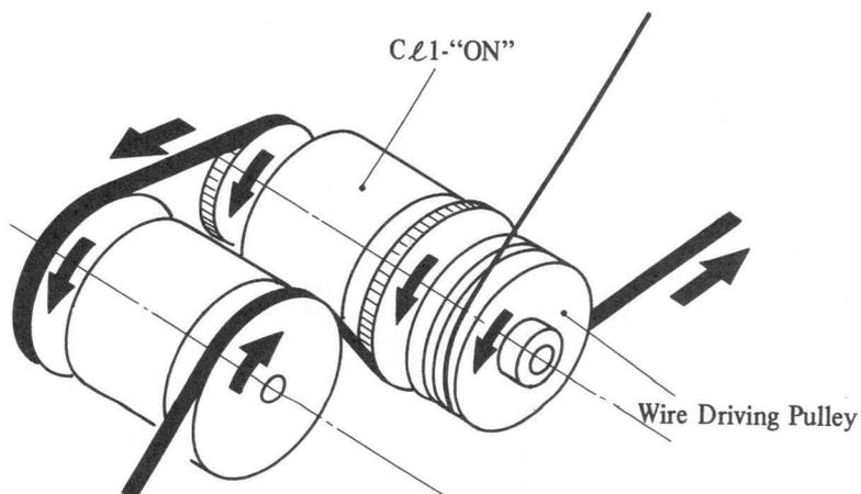
Fig. 4-126 Driving Mechanism Operation (B)
