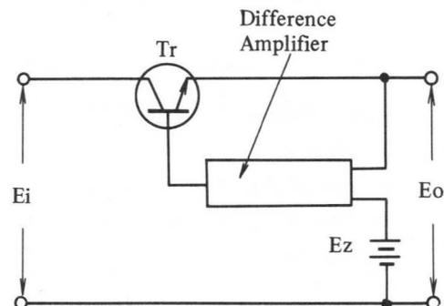
Fig. 3-6 Voltage Regulator - Typical
