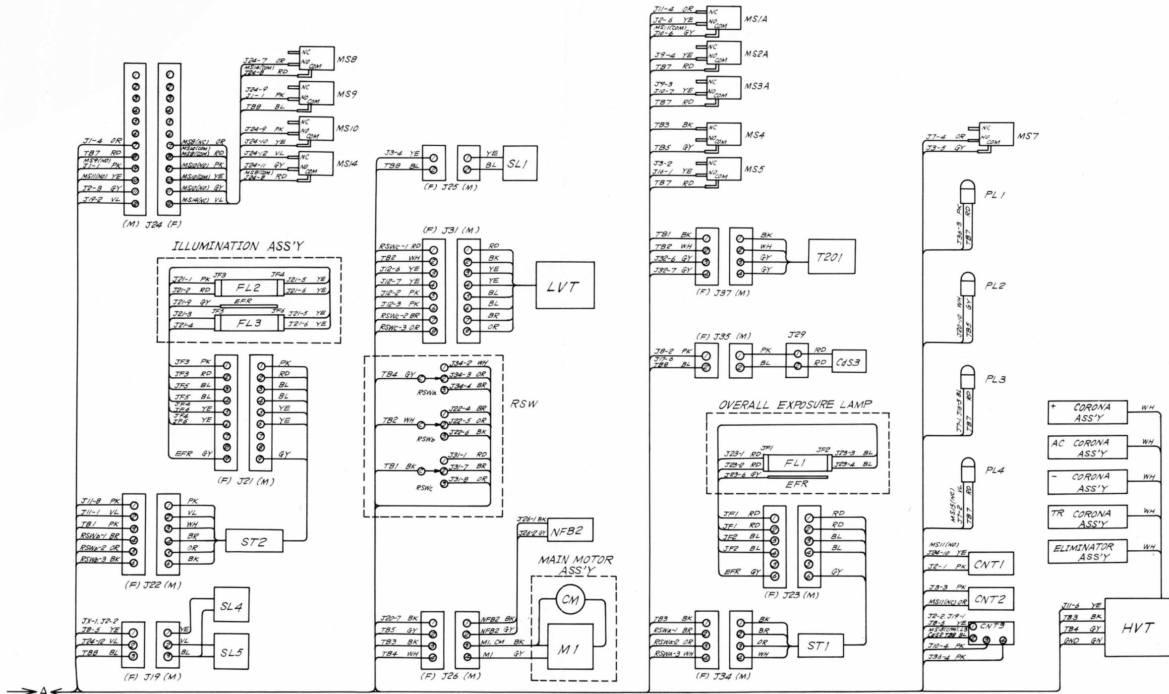
Photocopier Wiring Diagram, Prod. No. 8-11154/55 (2 of 2)
