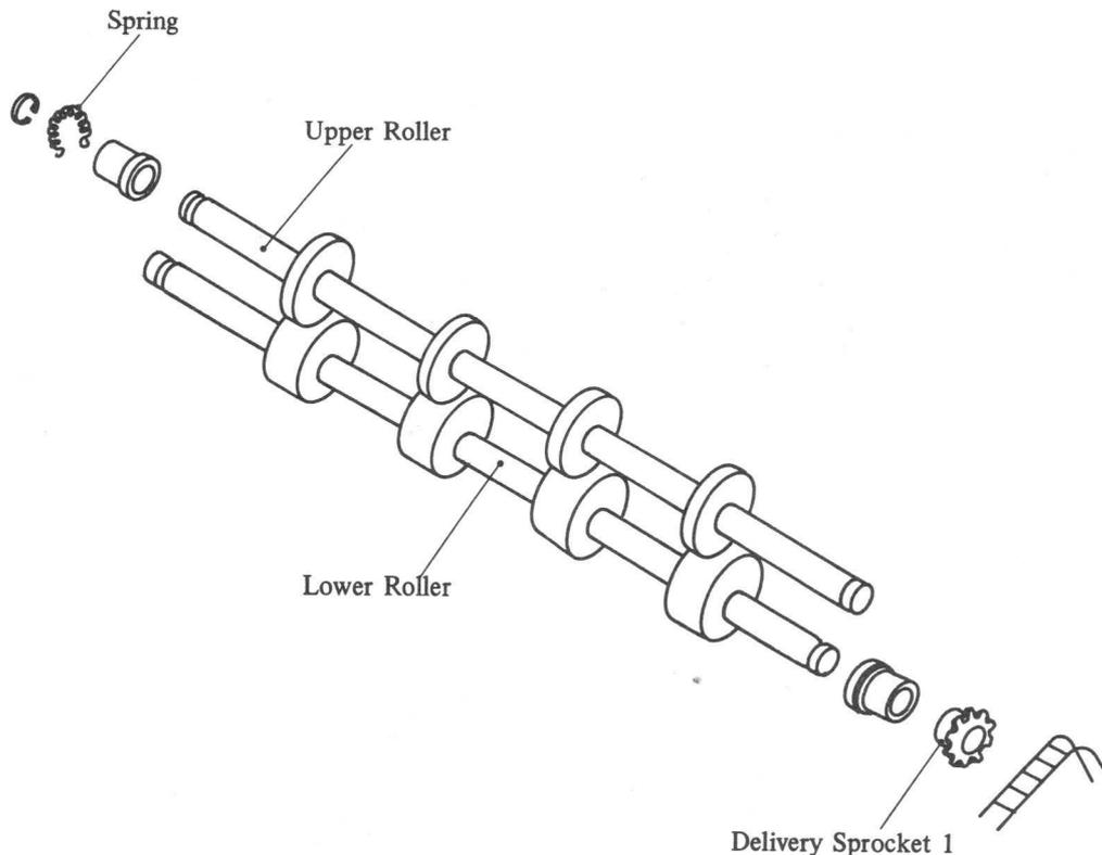
Fig. 4-87 Upper and Lower Rollers
