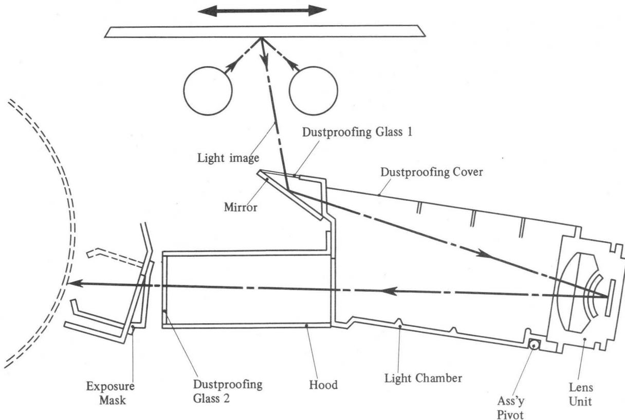
Fig. 4-18 Optical Assembly Main Components
