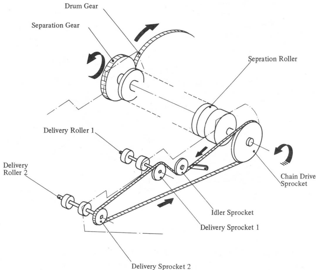
Fig. 2-8 Conveying Drive Mechanism
