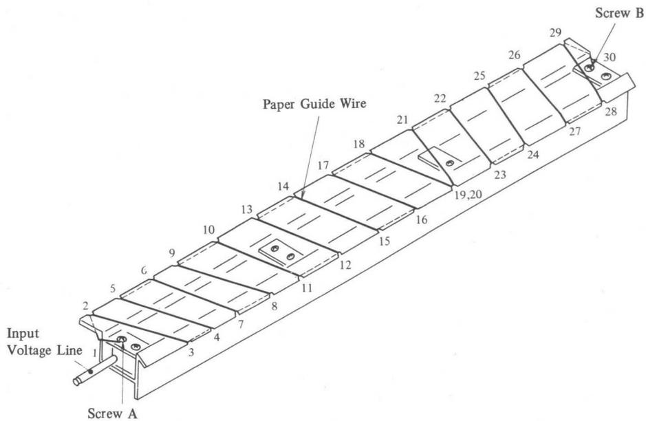
Fig. 4-30 Paper Guide Wire Replacement of Residual Charge Eliminator Assembly
