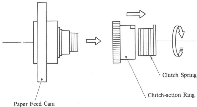
Fig. 4-78 Paper Feed Cam Drive Disassembly (C)
