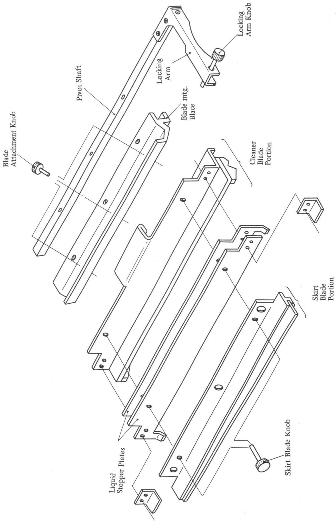
Fig. 4-53 Drum Cleaner Assembly Main Components (Exploded View)
