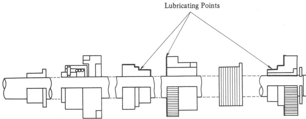
*Fig. 4-85 Timing roller Drive Lubrication*
