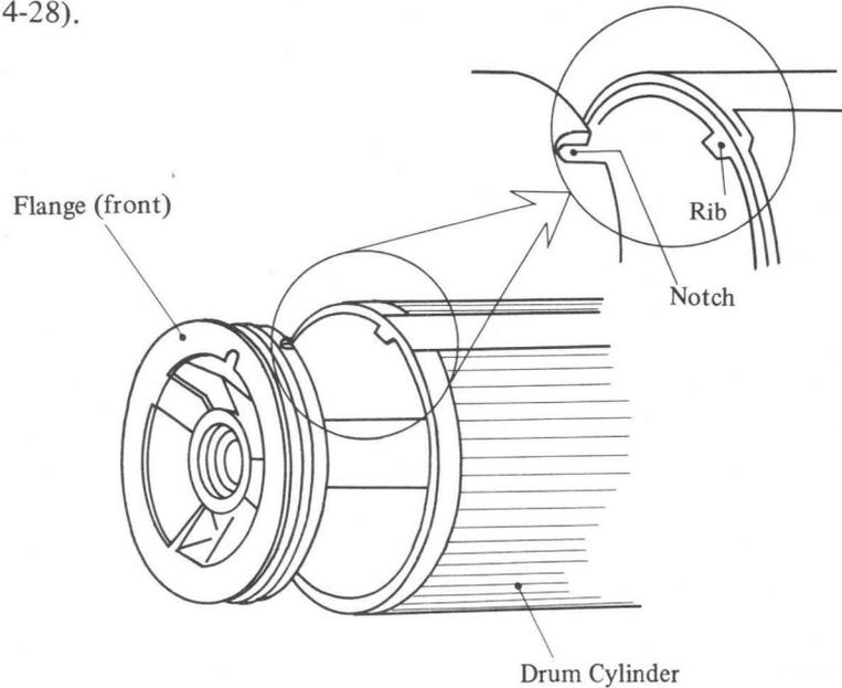
Fig. 4-28 Drum Unit Reassembly
