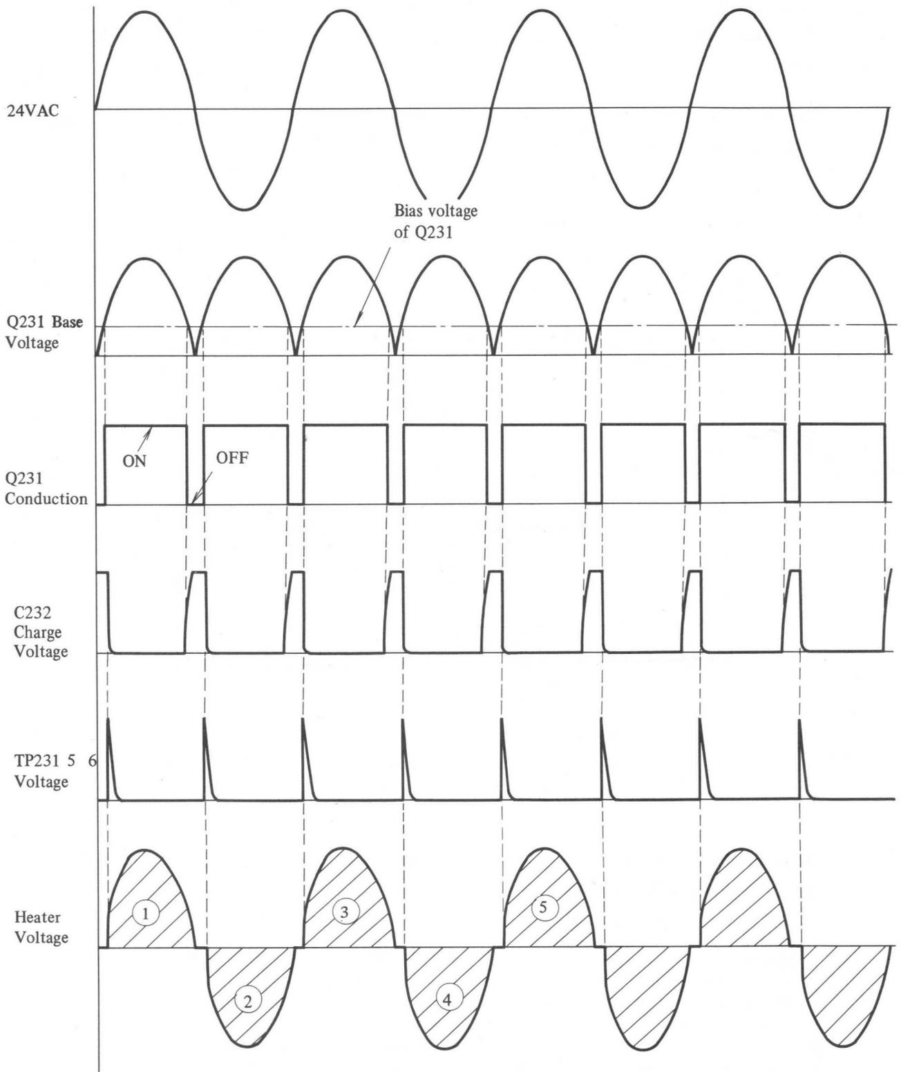
Fig. 3-25 1/1 "Zero-Cross" Waveforms
