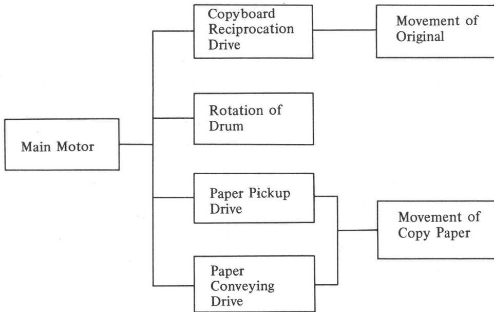
Fig. 2-3 General Diagram of the Drive System
