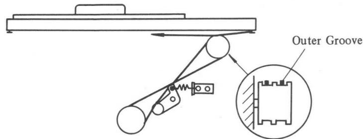
Fig. 4-7 Copyboard Wire Installation (C)
