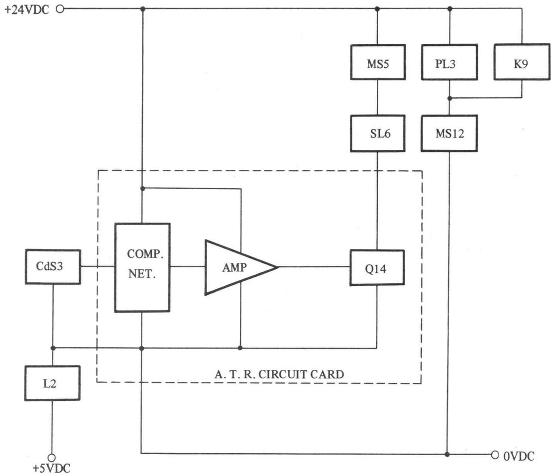
Fig. 3-11 Developer Monitoring Circuitry
