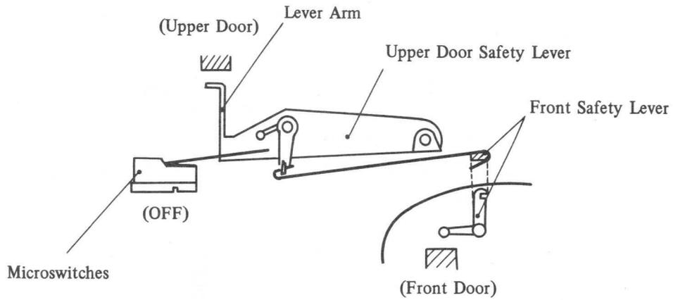
Fig. 4-116 Door Switch Group Operation (A)
