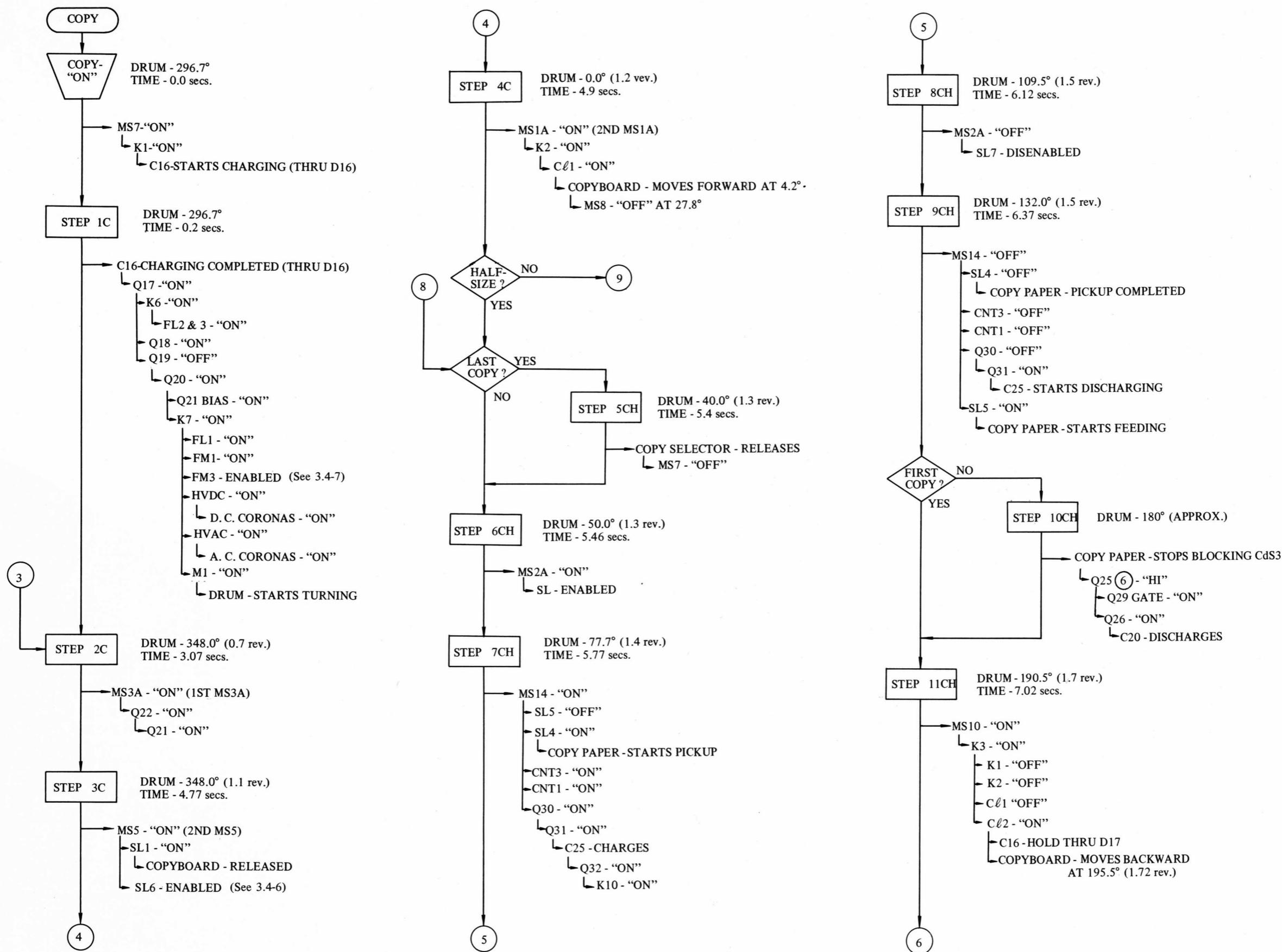
Fig. 3-2 **COPY** Flowchart (Sheet 1 of 3)
