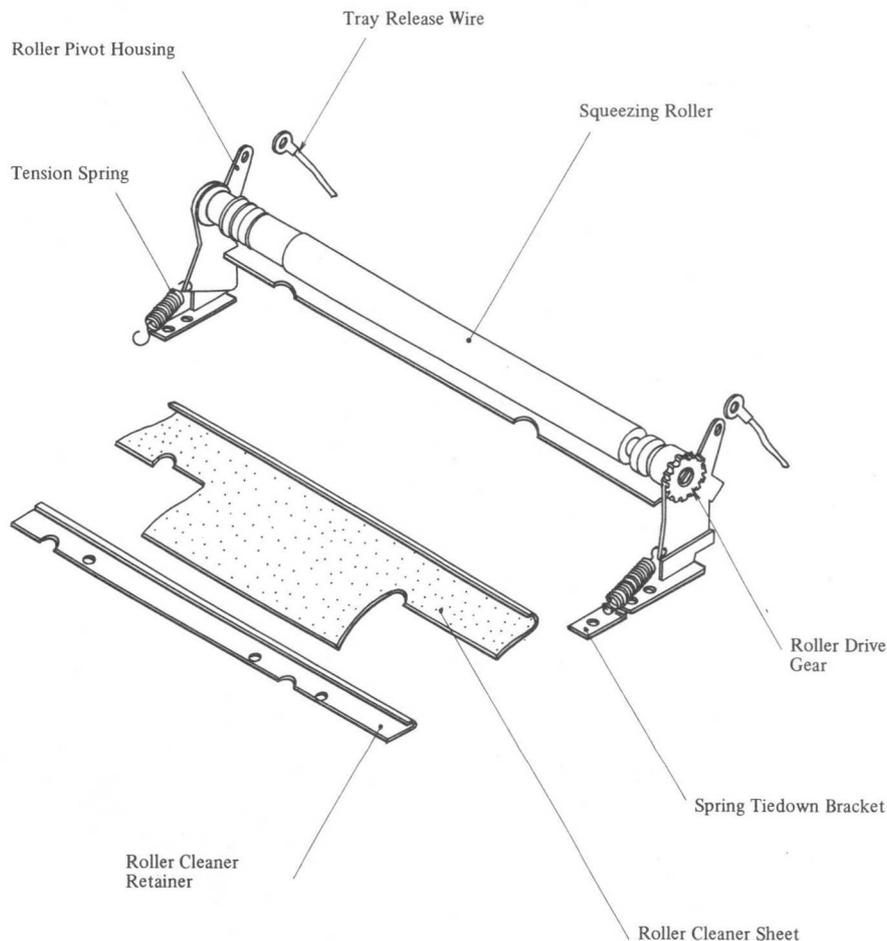
Fig. 4-40 Squeezing roller Main Components
