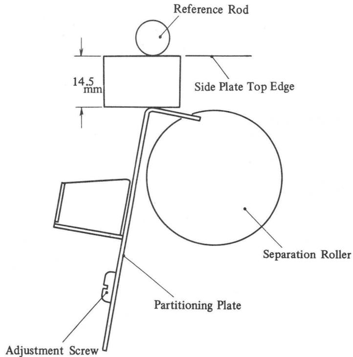
Fig. 4-94 Partitioning Plate Height Adjustment
