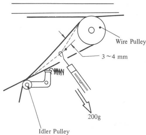
Fig. 4-9 Measuring of Wire Tension
