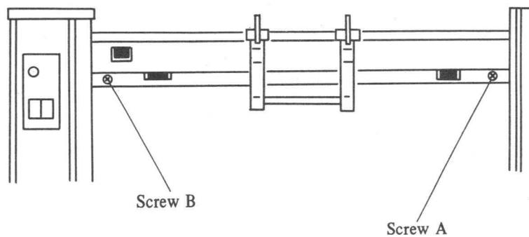
Fig. 4-95 Positions of Screws A and B
