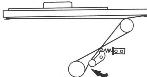
Fig. 4-8 Copyboard Wire Installation (D)
