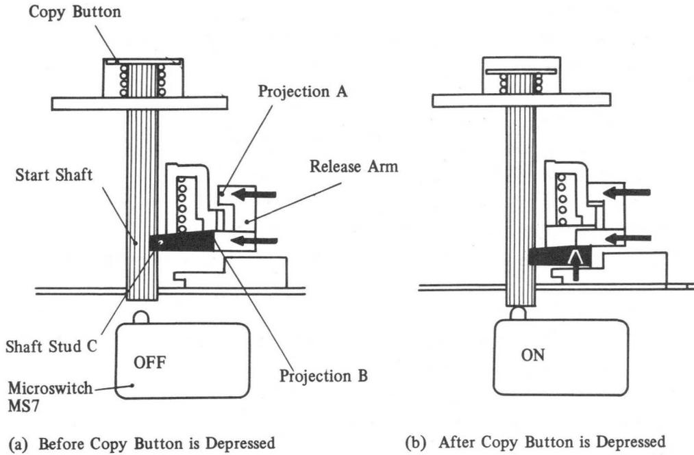
Fig. 4-106 Copy Selector Operation (A)
