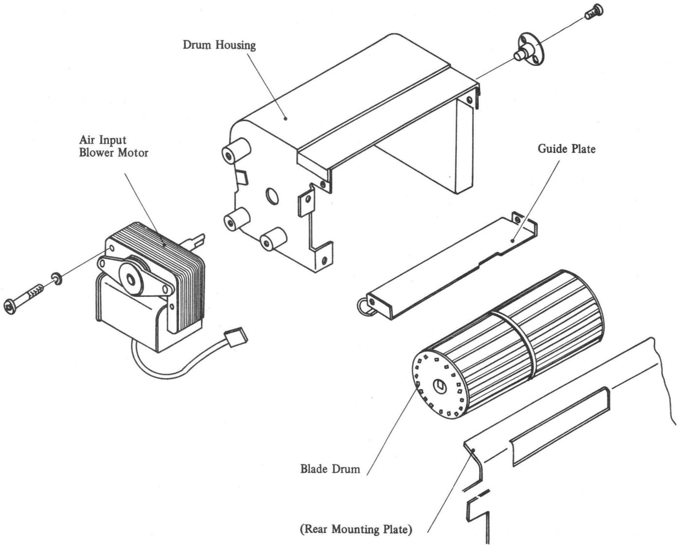
Fig. 4-101 Air Input Blower Assembly Main Components
