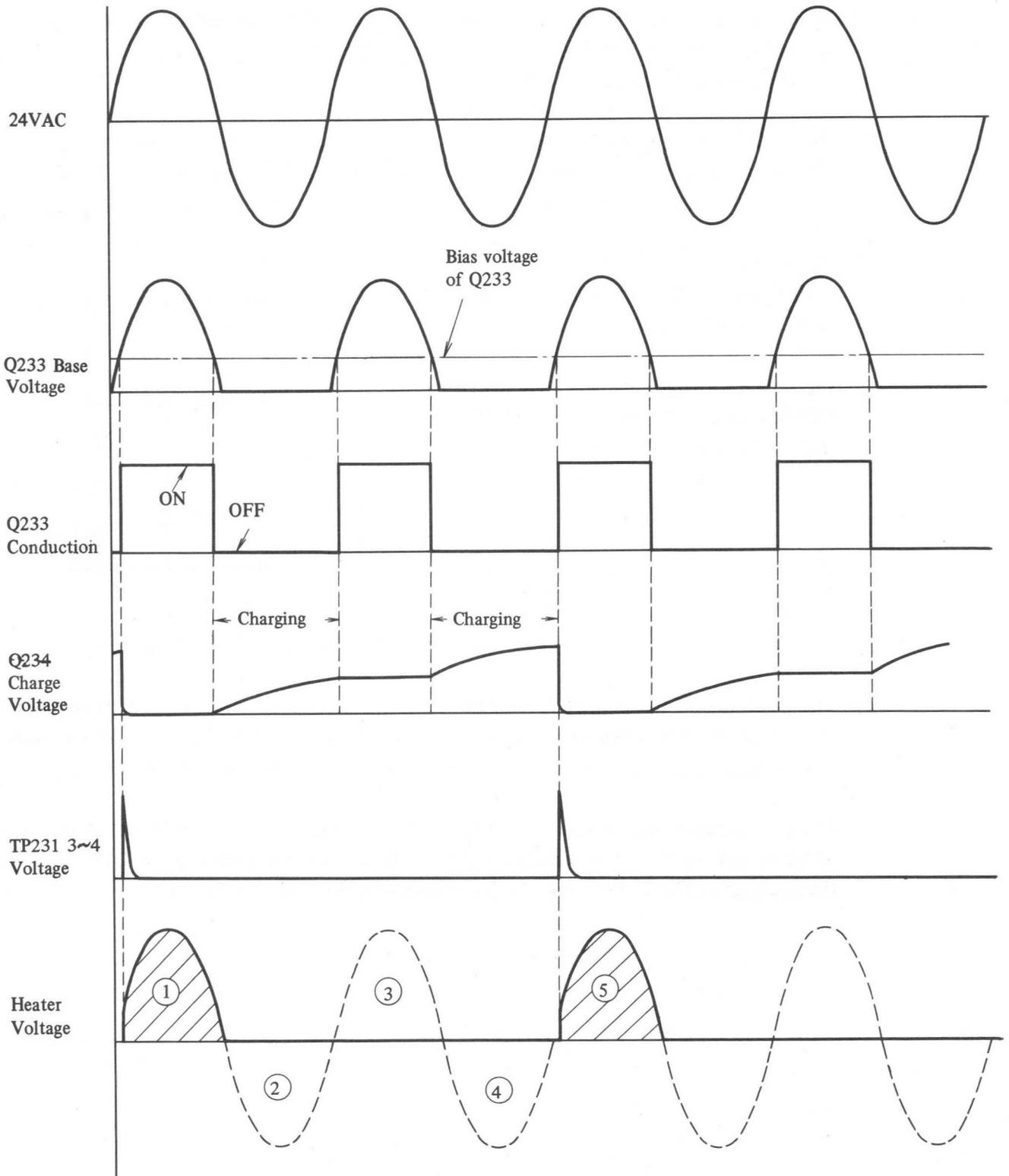
Fig. 3-23 1/4 "Zero-Cross" Waveforms
