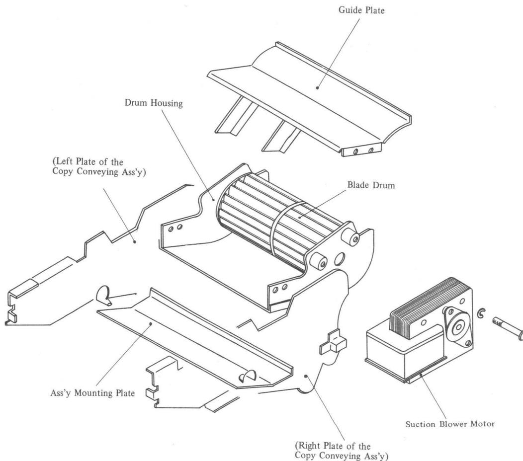
Fig. 4-100 Suction Blower Assembly Main Components
