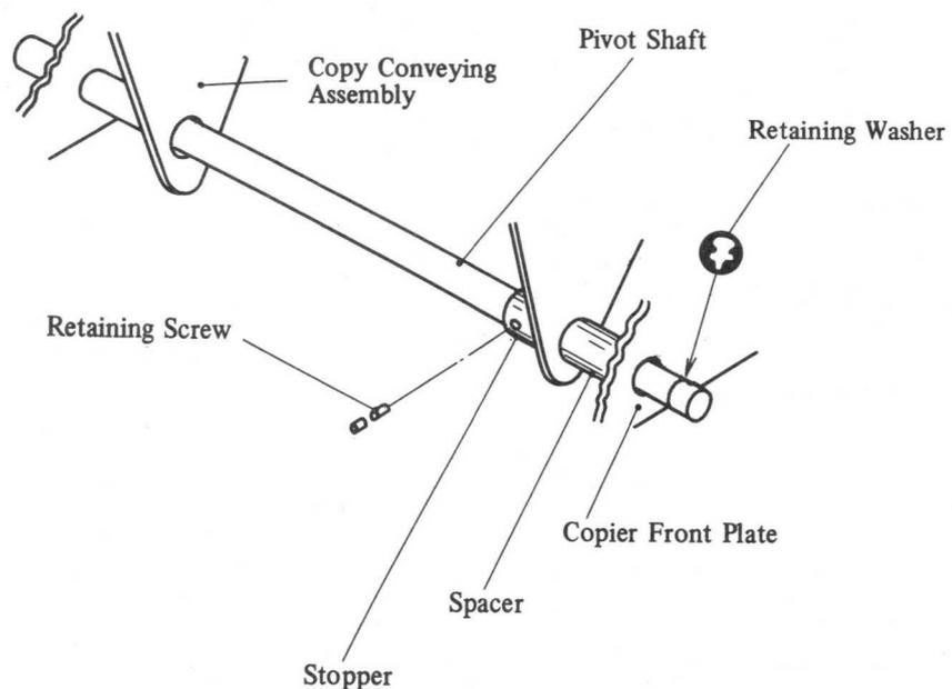
Fig. 4-91 Pivot Shaft Removal
