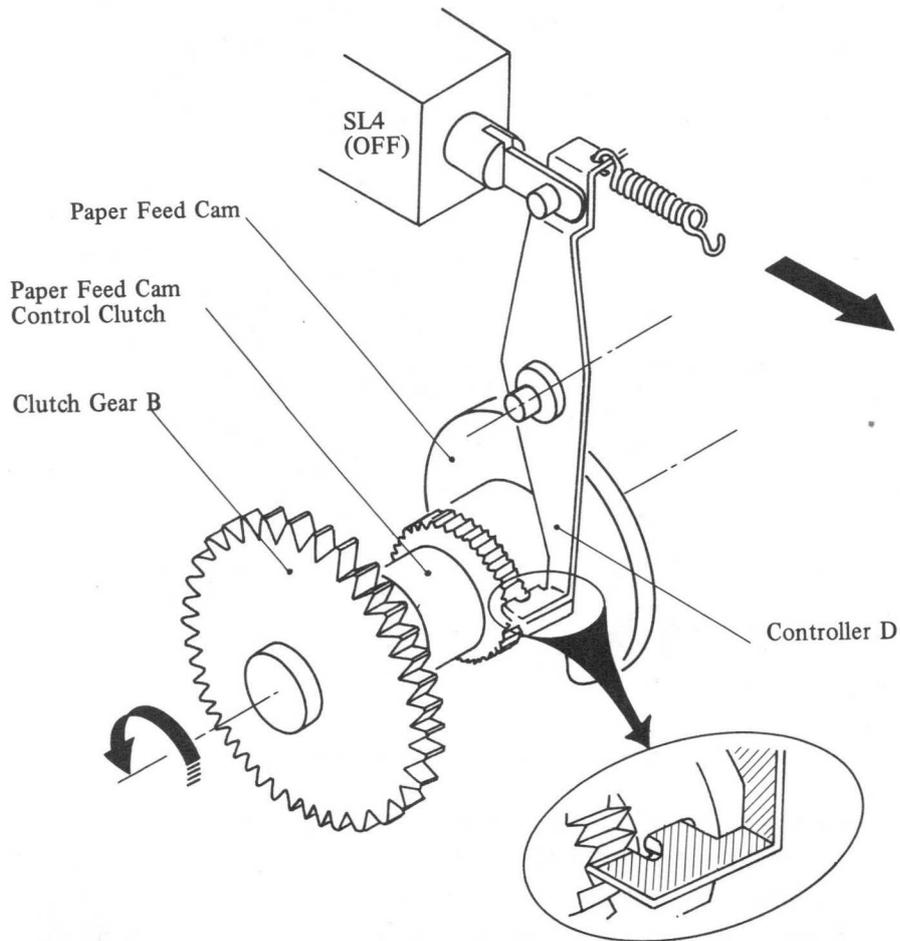
Fig. 4-62 Controller Assembly Operation (A)
