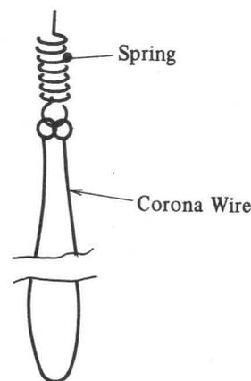
Fig. 4-32 Attaching Corona Wire
