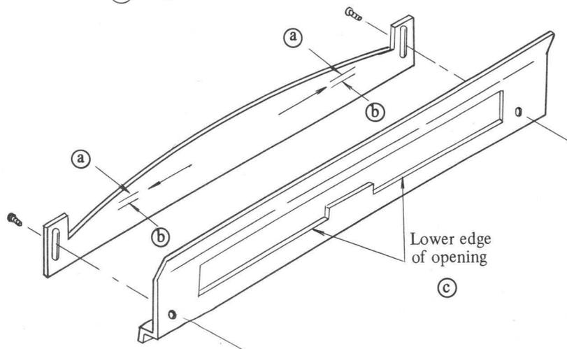
Fig. 4-24 Exposure Mask Adjustment
