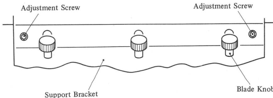
Fig. 4-55 Adjustment of Cleaner Blade Pressure (B)
