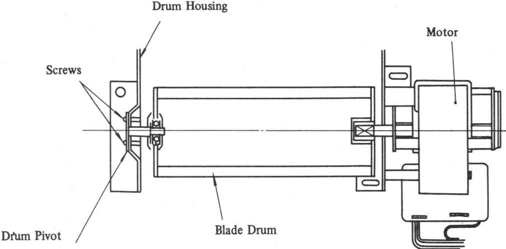
Fig. 4-103 Blower Blade Drum Adjustment
