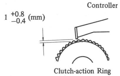
Fig. 4-80 Controller Spring
