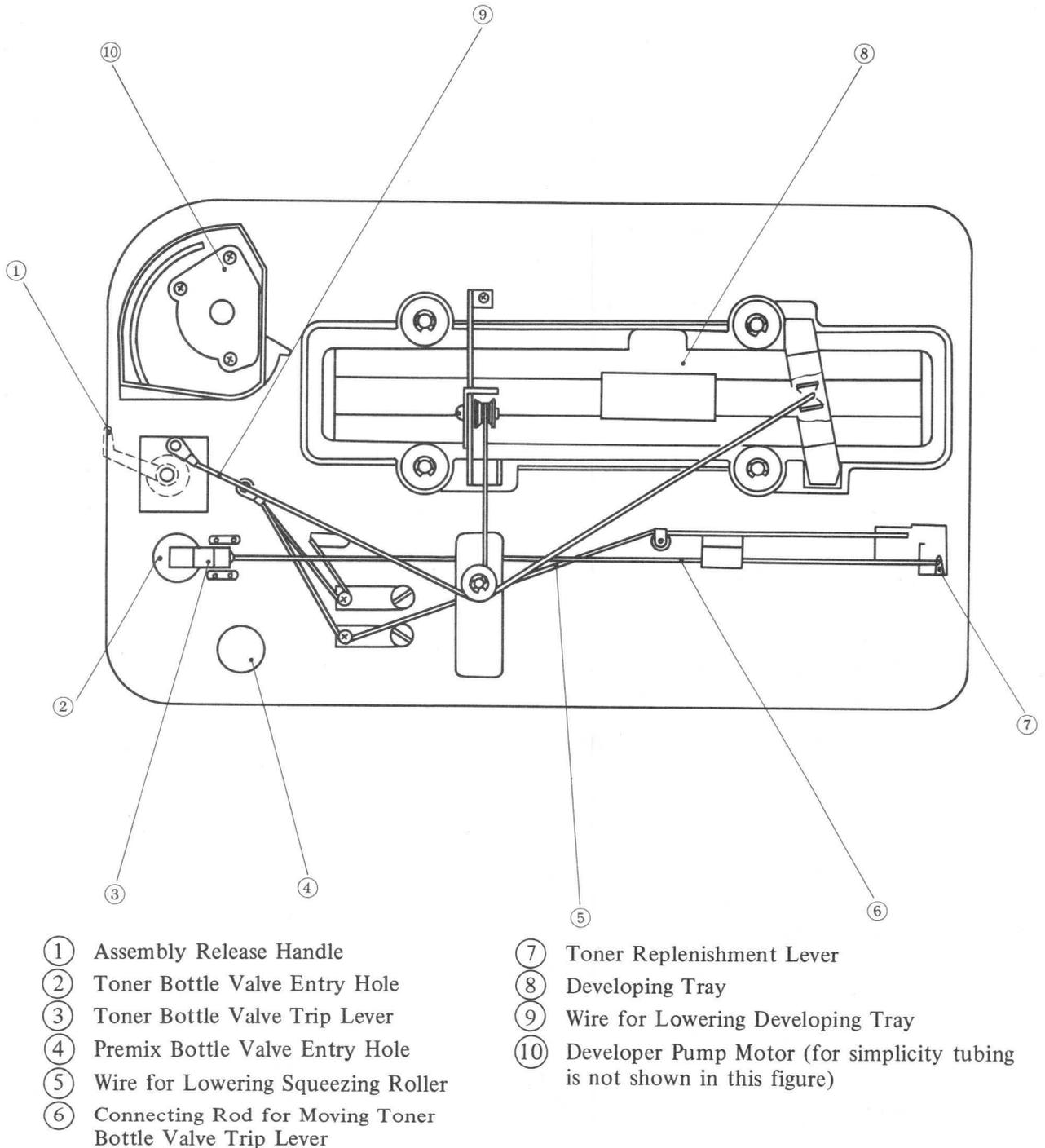
Fig. 4-41 Reservoir Cover Components (Underside View)
