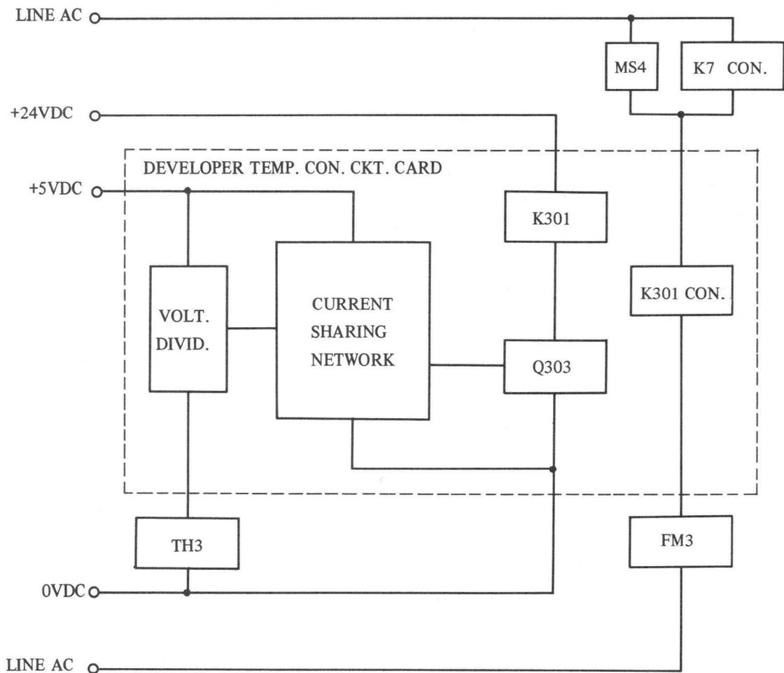
Fig. 3-14 Developer Temperature Control Circuit & Associated Components
