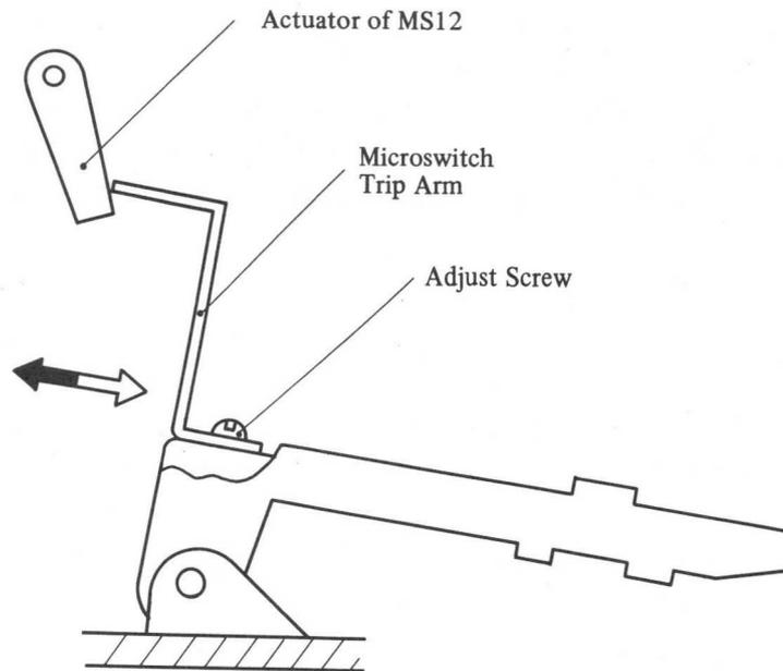
Fig. 4-51 Developer Float Adjustment
