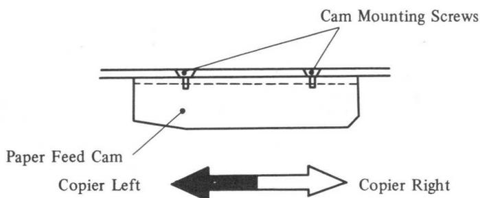
Fig. 4-12 Paper Feed Cam Adjustment
