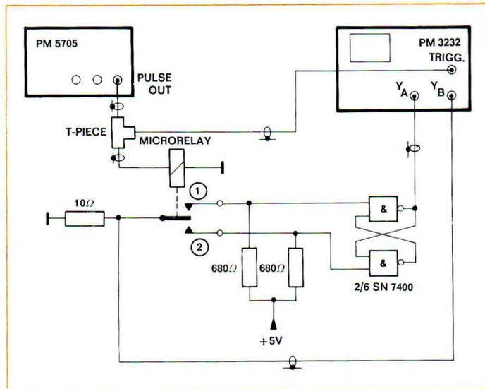
Fig. 4.51. Test set-up
