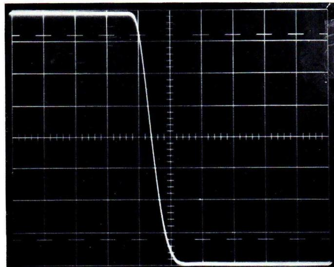
Fig. 4.8. PM 3232 Generator output unloaded
