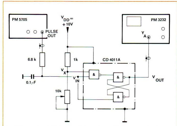
Fig. 4.103. Test set-up
