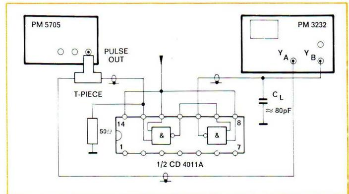
Fig. 4.88. Test set-up
