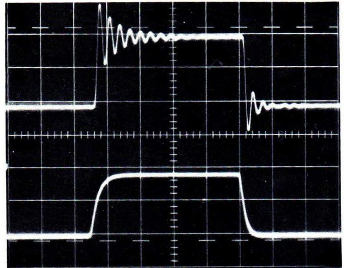
Fig. 4.30. Upper trace: Unterminated cables
