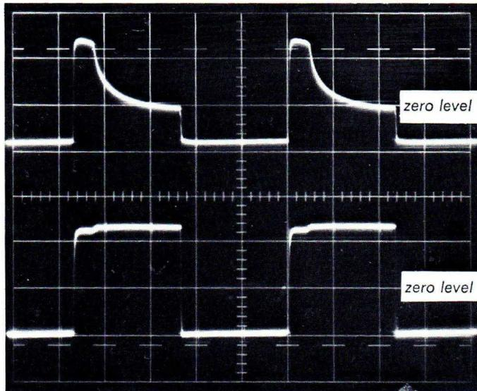
Fig. 4.41. Upper trace, ch. B: diode current. Forward current approx. 35 mA.
