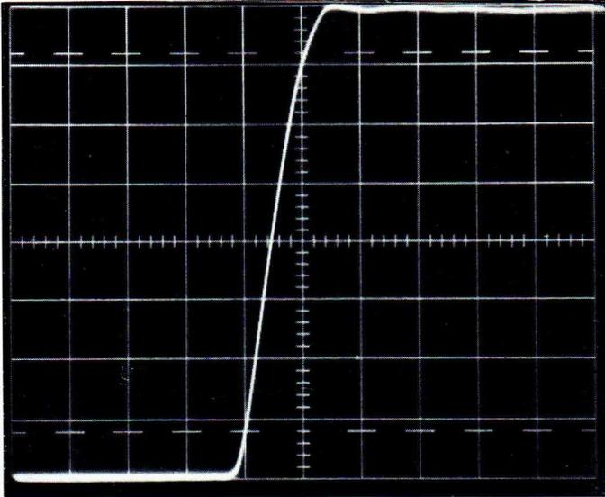
Fig. 4.11. PM 3232 Measured rise time 44 ns
