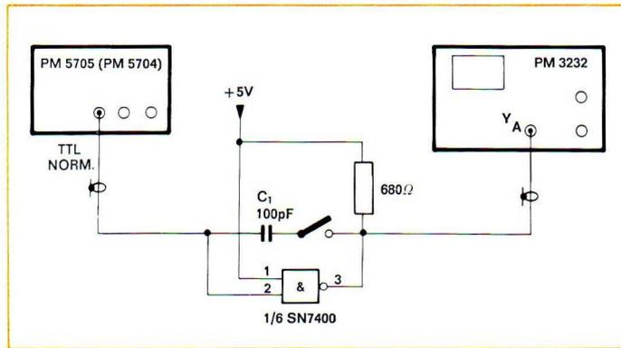
Fig. 4.16. Test set-up
