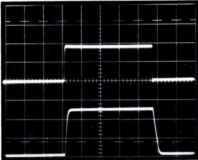
Fig. 4.92. Upper trace: Channel A, TTL pulse
