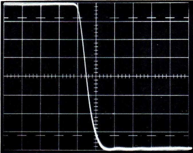
Fig. 4.14. PM 3232: measured fall time 36 ns
