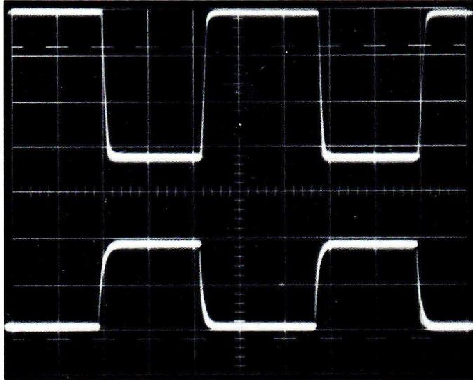
Fig. 4.100. Upper trace: channel A, 2 V/cm. Amplitude 6  $V_{p-p}$
