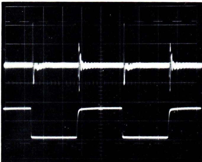
Fig. 4.85. Upper trace (A): voltage across the 100 ohm resistor
