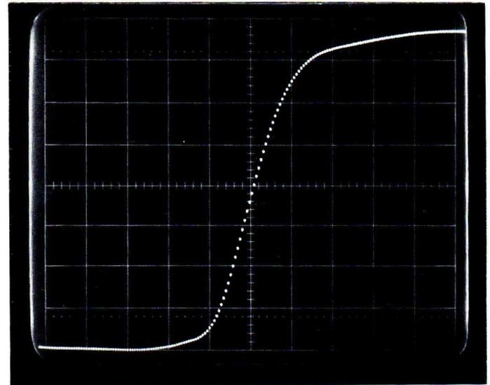
Fig. 4.13. PM 3400 Measured rise time 13 ns
