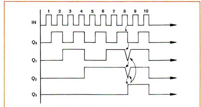
Fig. 4.73. Timing diagram for a ripple decade counter
