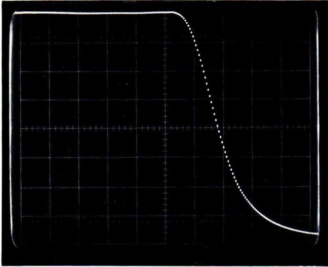
Fig. 4.9. PM 3400 Generator output unloaded
