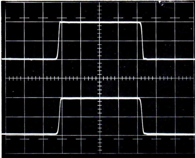
Fig. 4.36. Upper trace: Unterminated cables.
