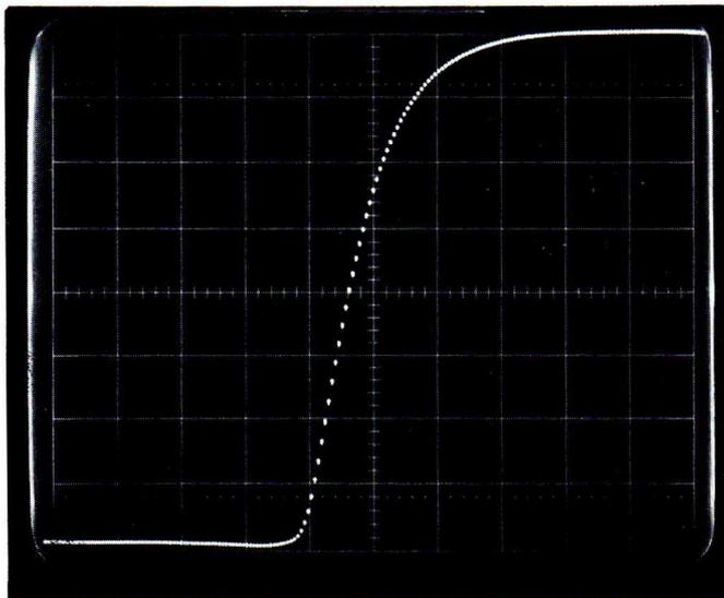
Fig. 4.7. PM 3400 Output unloaded:
