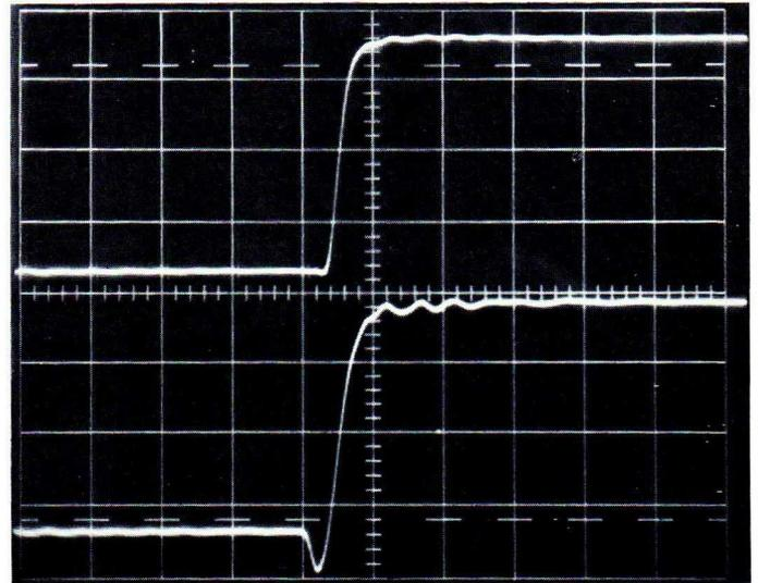
Fig. 4.17. Upper trace: without  $C_1$  a small preshoot can be observed
