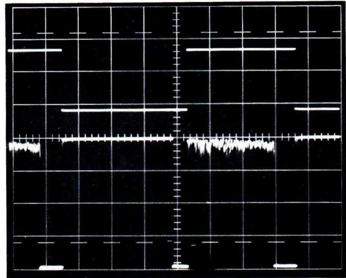
Fig. 4.52. Upper trace: (channel A) the output signal of the RS flip-flop
