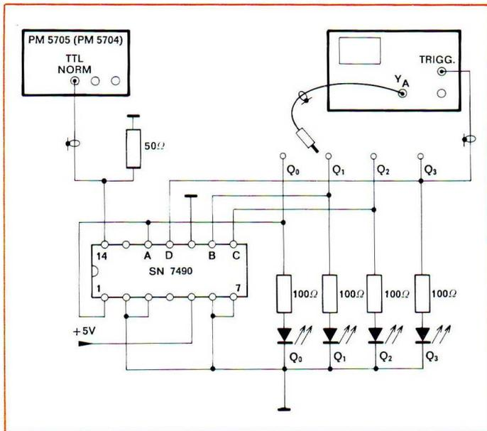
Fig. 4.84. Test set-up
