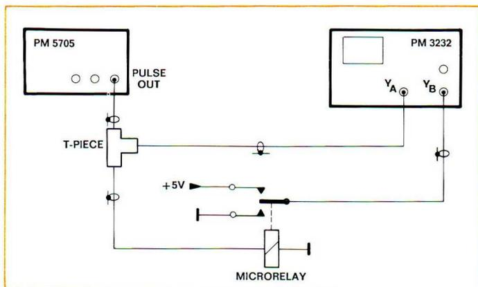
Fig. 4.47. Test set-up
