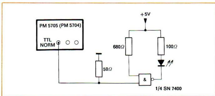
Fig. 4.113. Test set-up
