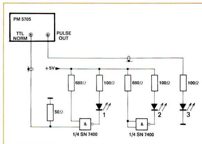
Fig. 4.114. Test set-up
