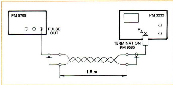
Fig. 4.31. Test set-up
