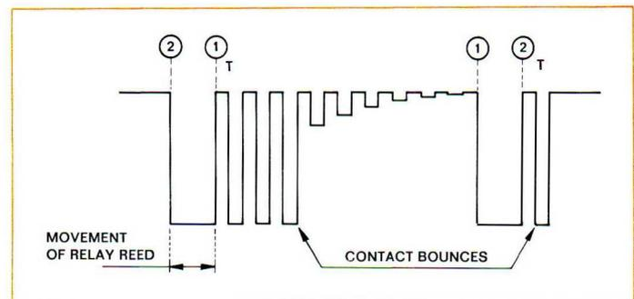
Fig. 4.53. Notice how the RS flip-flop is triggering on the very first contact at position  $1_T$  and  $2_T$  respectively.
