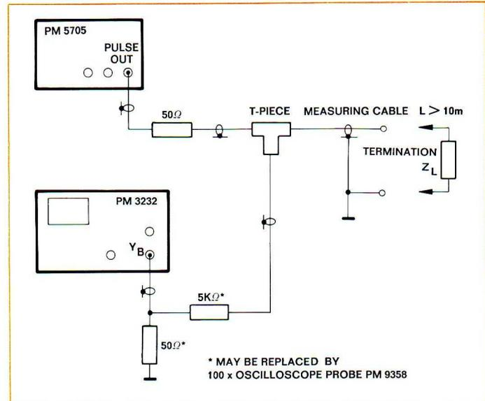
Fig. 4.18. Test set-up
