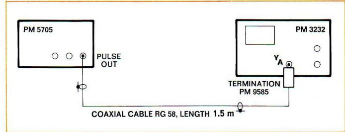
Fig. 4.33. Test set-up
