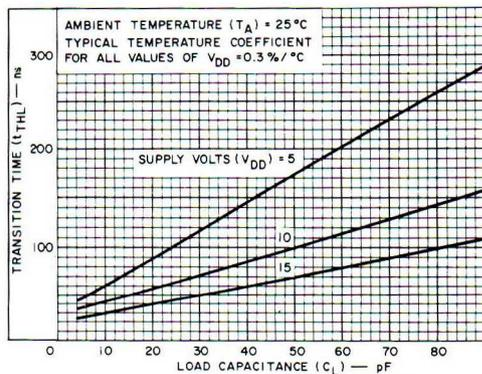
Typ. high-to-low level transition time vs.  $C_L$  – CD4011A & CD4023A.
