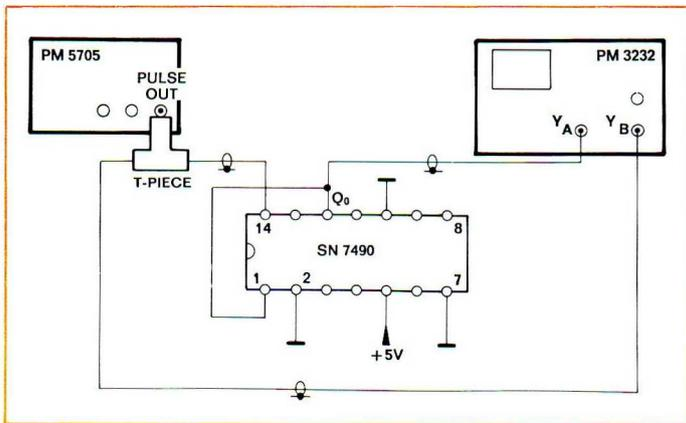
Fig. 4.56. Test set-up
