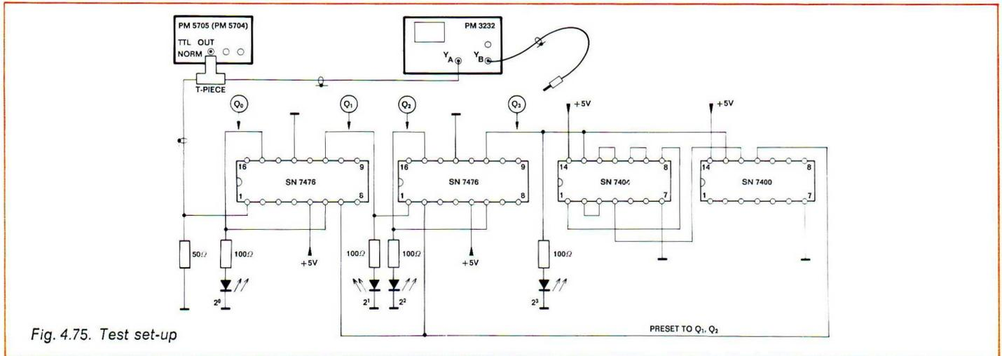
The pulse generator is connected as in exercise 20. Using the SINGLE SHOT function, we can verify that the counter now has a cycle of 10 pulses.
