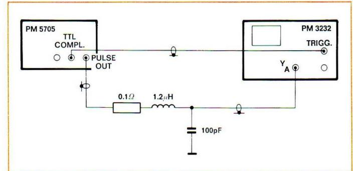
Fig. 4.37. Test set-up
