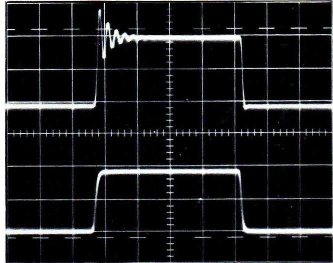
Fig. 4.34. Upper trace: Still overshoots without termination. Matching improved at negative step.
