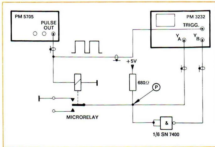
Fig. 4.49. Test set-up
