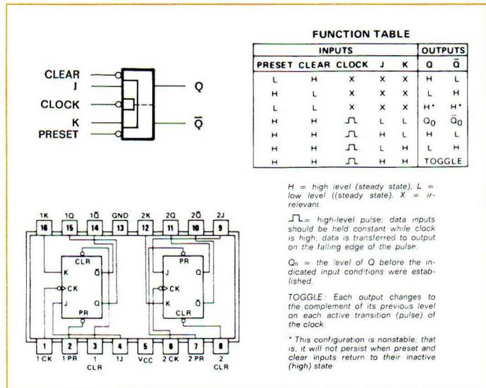
Fig. 4.68. Schematic symbol, truth table and data sheet drawing of SN 7476N
