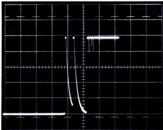
Fig. 4.48. The micro-relay turns on. Spacing between contact bounces is about 0.1 ms i.e. a frequency of 10 kHz.
