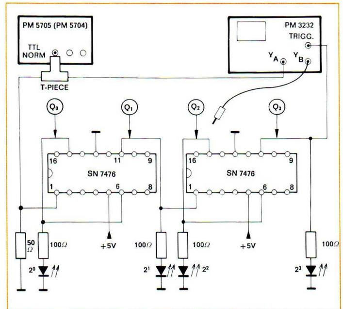
Fig. 4.71. Test set-up
