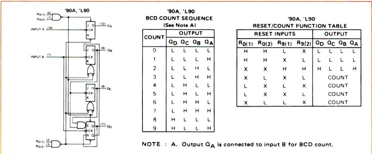
Fig. 4.83. Truth tables, diagram of SN 7490
