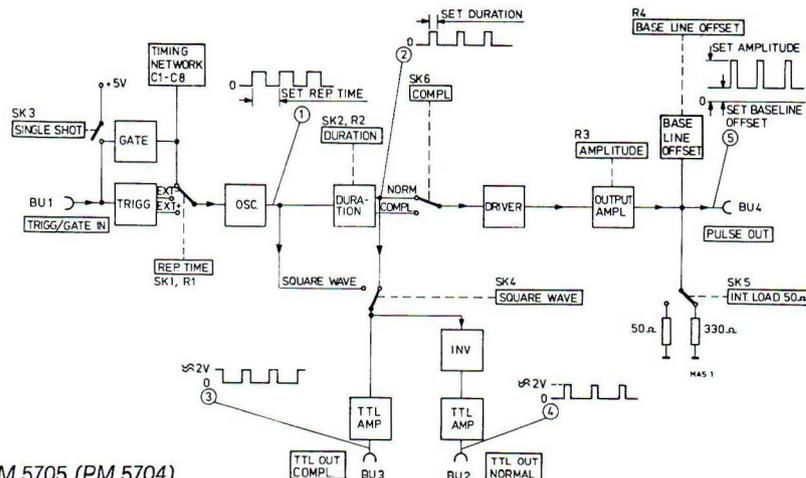
Fig. 2.1. Block diagram PM 5705 (PM 5704)
