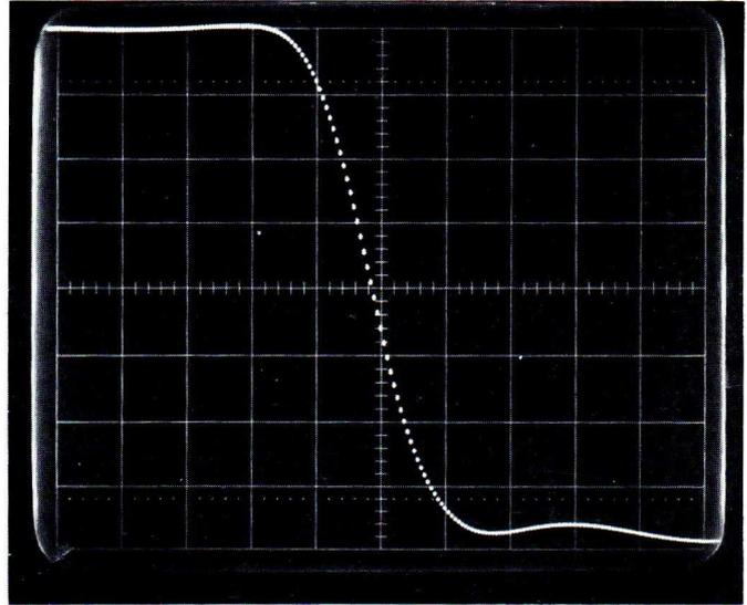
Fig. 4.15. PM 3400: measured fall time 9 ns
