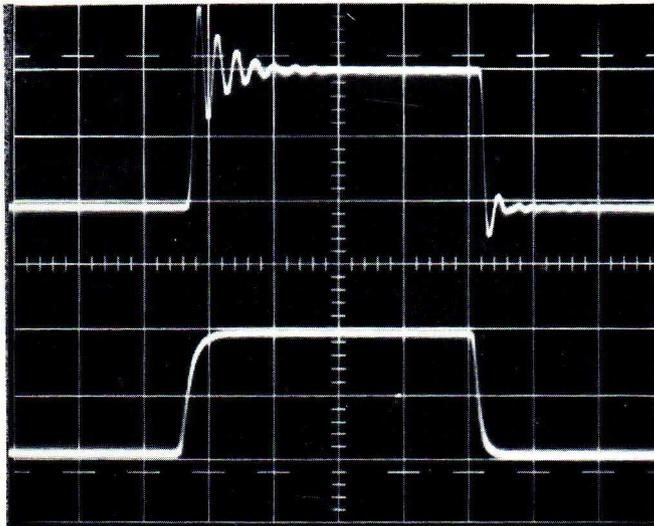
Fig. 4.32. Upper trace: Underterminated cables
