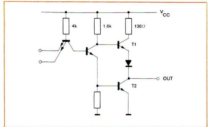
Fig. 4.42. Circuit diagram of a TTL output
