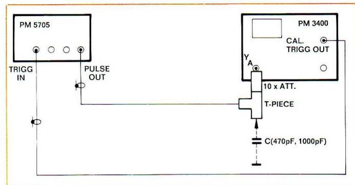
Fig. 4.6. Test set-up
