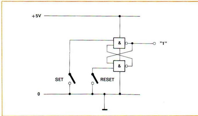
Fig. 4.45. RS flip-flop
