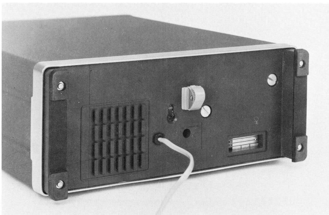
Fig. 2.1. Rear view of the oscilloscope showing the voltage adapter set to 220 V.
