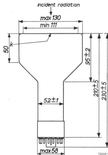
Dimensions (in mm) and electrode connections
