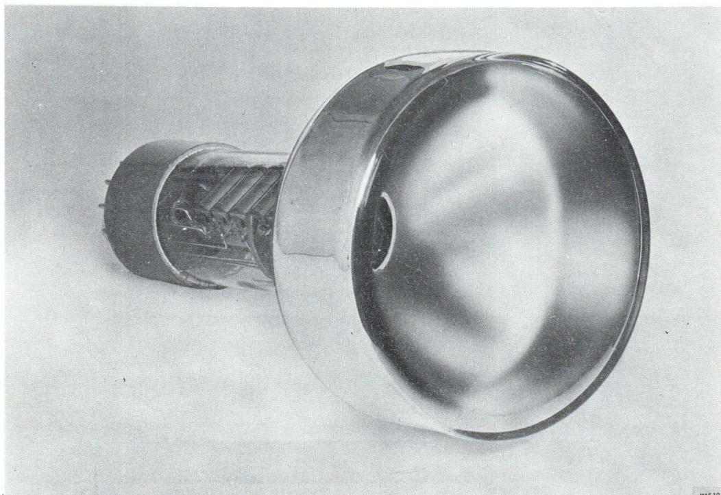
The 54AVP is an 11-stage photomultiplier tube provided with a caesium-antimony, semi-transparent flat cathode having a diameter of 111 mm. The highly sensitive uniform photocathode has a typical sensitivity of  $60 \mu\text{A}/\text{lm}$  and a spectral response lying mainly in the visible region, with its maximum at  $4200 \text{ \AA}$ , as shown in the spectral response curve.
