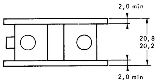
The pinch off cap must not extend beyond the flange.
