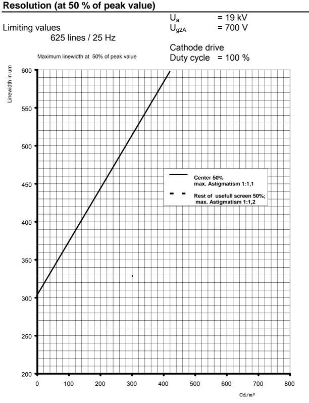
The focus is adjusted at 100 cd/m<sup>2</sup> and it is not allowed to readjust the focus voltage during the measurement. Measured with PDS spotvision system or Microvision SS100
