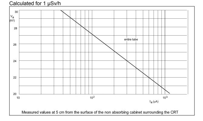
The X-radiation emitted will not exceed 1  $\mu$ Sv/h for anode voltage and current combinations shown in the iso-exposure-rate limit curve, according to Eigensichere Kathodenstrahlröhre nach "*Anlage III Röntgenverordnung*".
